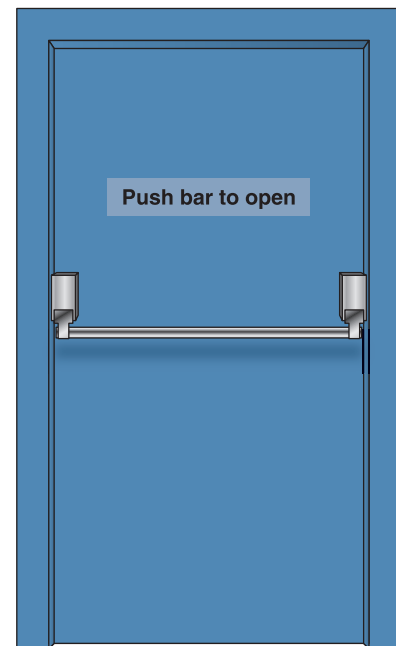
FIGURE 12-23 A typical personnel door that opens easily by pushing on the panic bar.
