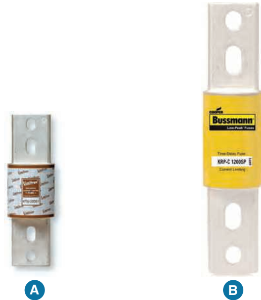
FIGURE 17-10 Class L fuses. All Class L fuses are rated 600 volts. Listed in 100- to 6000-ampere rating.
