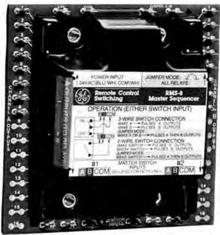
FIGURE 20-8 Master sequencer available in three sizes to control 8, 16, or 32 relays.
