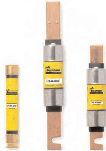
FIGURE 17-4 Dual-element, time-delay, current-limiting Class RK1 fuses. They provide time delay in the overload range and are fast acting in the short-circuit range.
