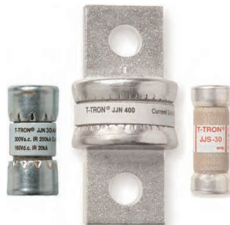
FIGURE 17-11 Class T current-limiting, fast-acting fuse; 200,000-ampere interrupting rating.
