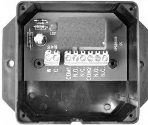
FIGURE 11-10 Relay in NEMA 1 enclosure.
