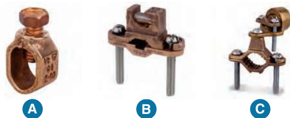
FIGURE 13-26 Typical ground clamps. (A) For ground rods; (B) for connection to concrete-encased grounding electrodes or smaller pipes; (C) for connecting conduit containing grounding electrode conductor and the grounding electrode conductor to metal pipe.
