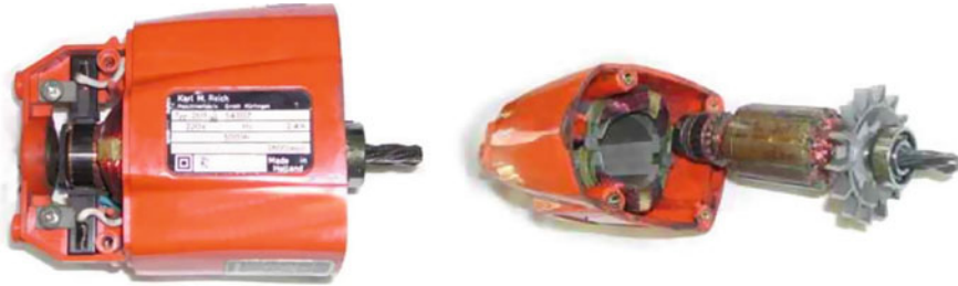
Fig. 19.6 Small grinding motor
