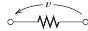
Figure 1.13 The positive reference for v is at the head of the arrow.
