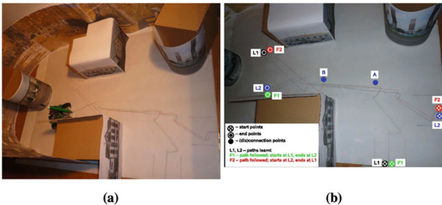
Fig. 23.8 Paths learnt ( blue and black ) and followed, with small scenario changes. The robot plans correctly the routes and is immune to small changes in the reconstituted urban scenario
