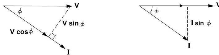
Figure 2.2 Phasor Diagrams Leading to Power Triangles.
