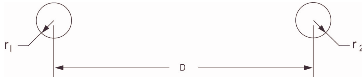
Figure 5.1 Single-Phase Two-Wire Line Configuration.
