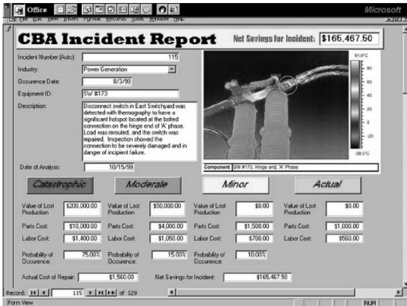
FIGURE 11.21 Typical cost benefits analysis report provided by the web-based method developed by the Maintenance Reliability Group (MRG). (From Wurzbach, R. N., A web-based cost benefit analysis method for predictive maintenance, http://www.mrgcorp.com . With permission.)
