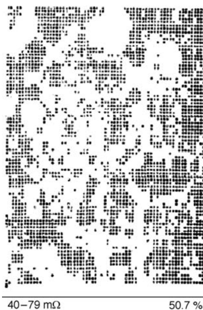
FIGURE 10.2 Distribution of measuring points with a surface resistance between 40–79 m \Omega . The total surface area scanned is 450 \times 600 \mu\text{m}^2 . (From Voostrom, A., Augustus, L., Steinmetz, A., and Berg, G., Proceedings of 24th Holm Conference on Electrical Contacts , Illinois Institute of Technology, Chicago, IL, 1978, 521–526. With permission.)
