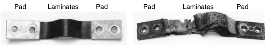
FIGURE 7.11 Typical examples of flexible tinned copper connectors: intact and failed connector.
