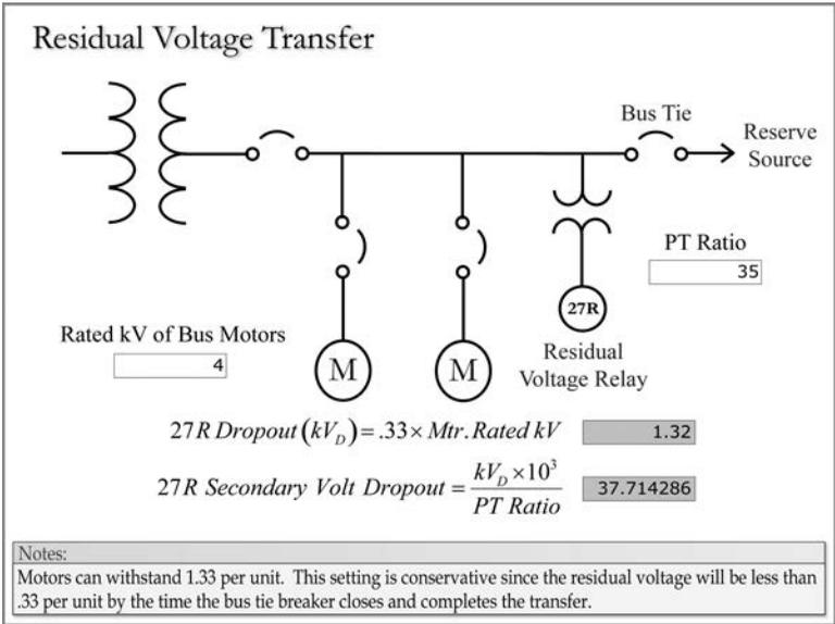
FIGURE 3.40 Residual voltage relay settings.
