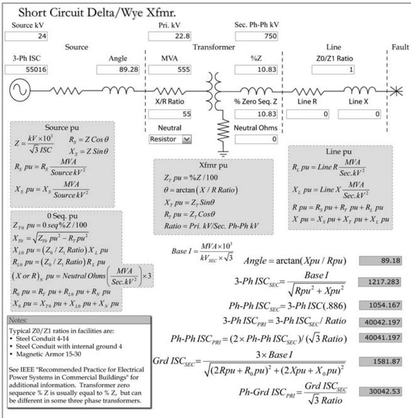
**FIGURE 4.38** GSUT short circuit currents.
