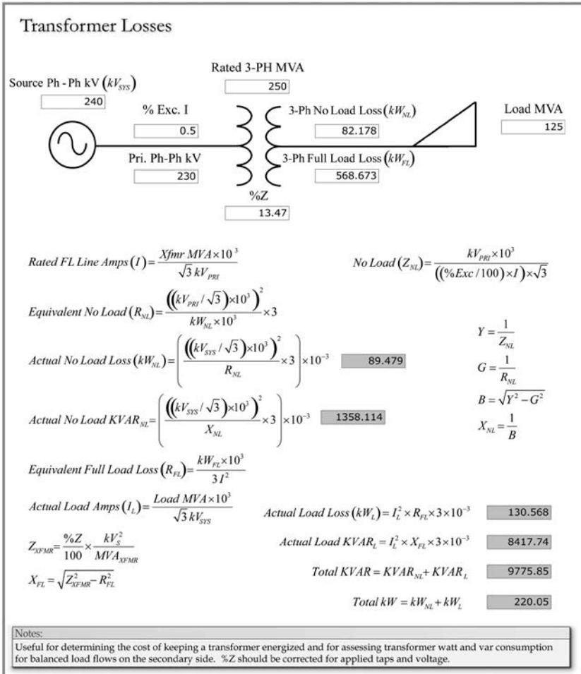
FIGURE 5.32 Transformer losses.
