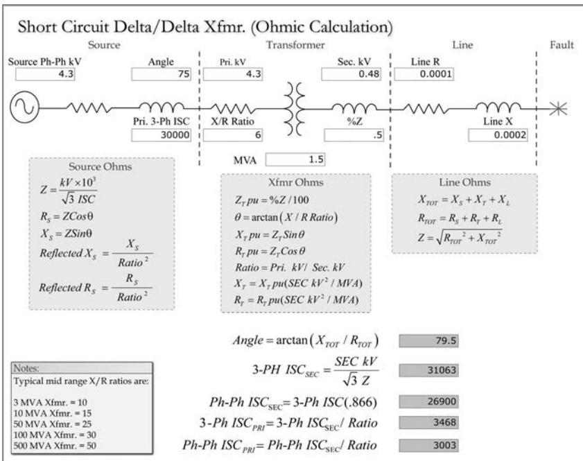
**FIGURE 2.48** Comparing per-unit to ohmic short circuit procedures.
