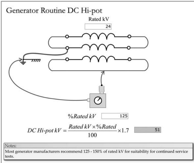
**FIGURE 5.8** Generator stator routine DC overvoltage testing.
