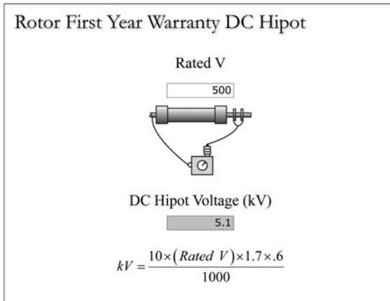
**FIGURE 7.10** Generator rotor first-year warranty DC overvoltage testing.
