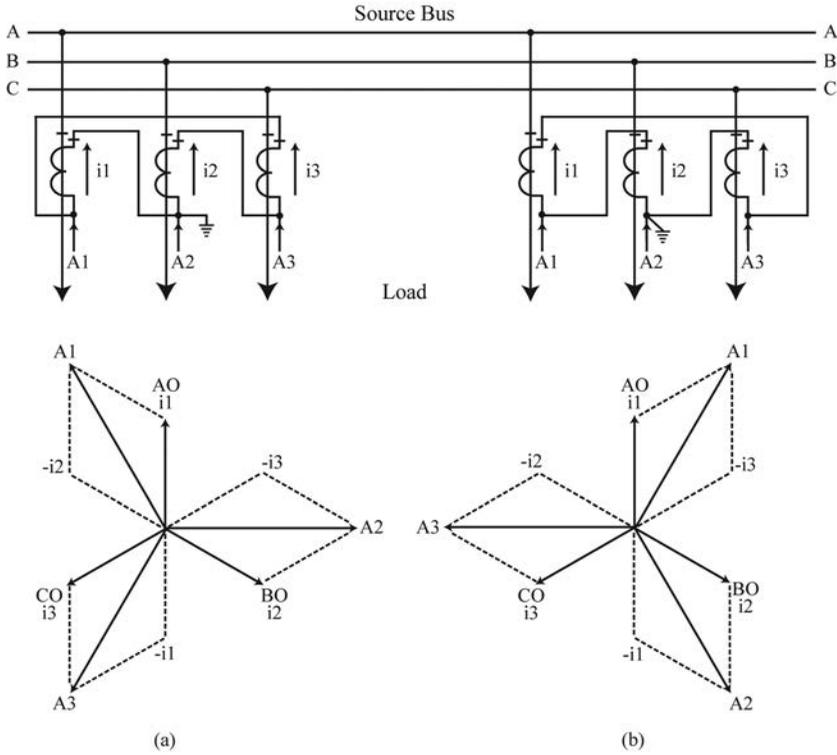
**FIGURE 1.65** Current transformer delta lead and lag connections.
