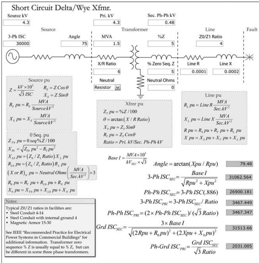
FIGURE 2.43 Delta-wye transformer short circuit.
