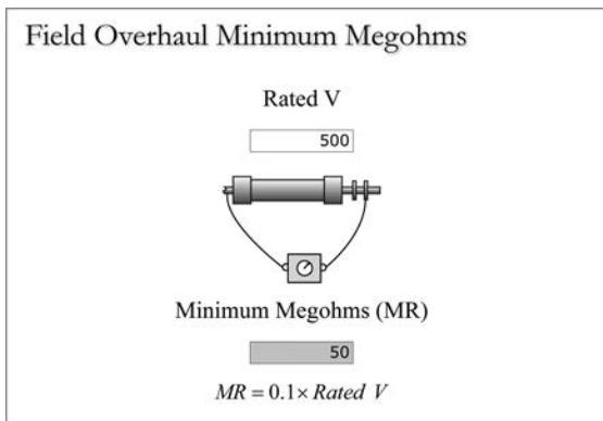
**FIGURE 7.11** Generator rotor routine overhaul insulation testing.
