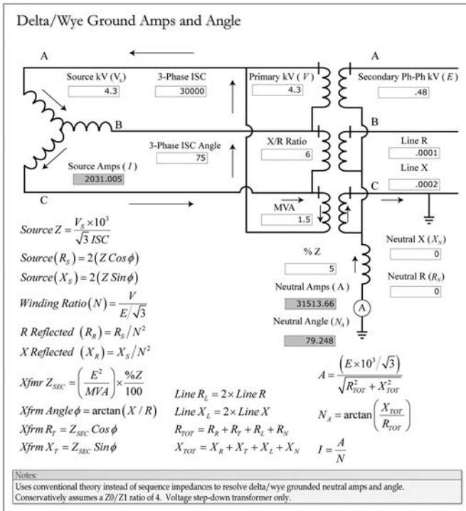
**FIGURE 2.53** Step-down transformer ohmic ground fault calculation.
