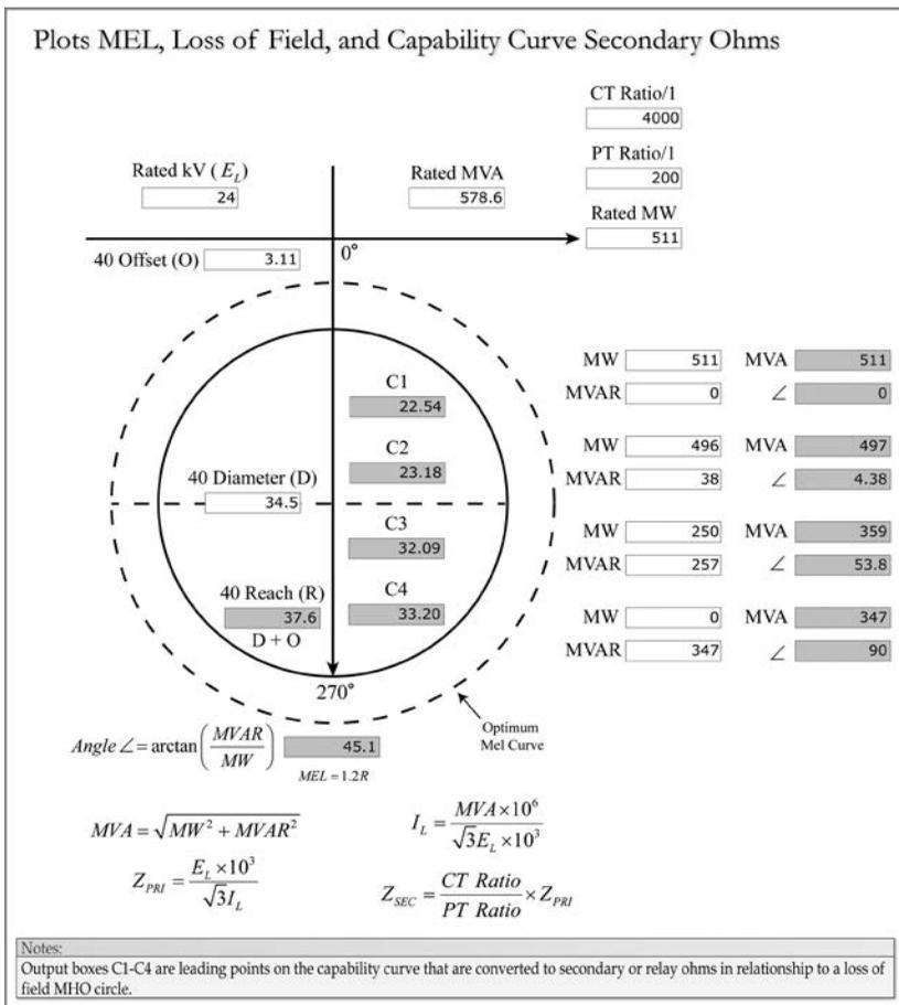
**FIGURE 7.15** Loss-of-field, MEL, and capability curve ohmic plots.
