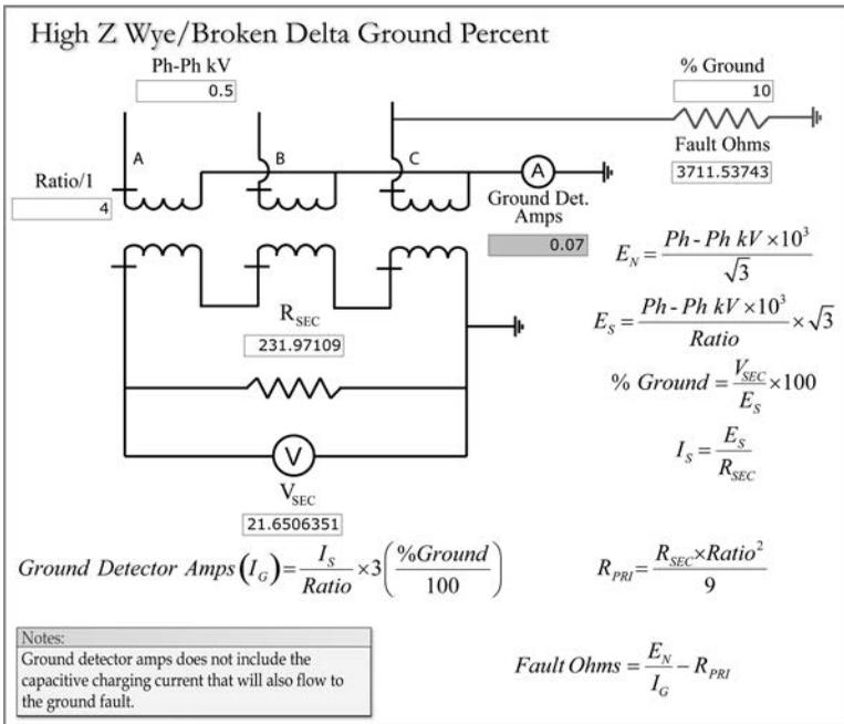
**FIGURE 3.34** Grounded wye–broken delta ground detector fault ohms.
