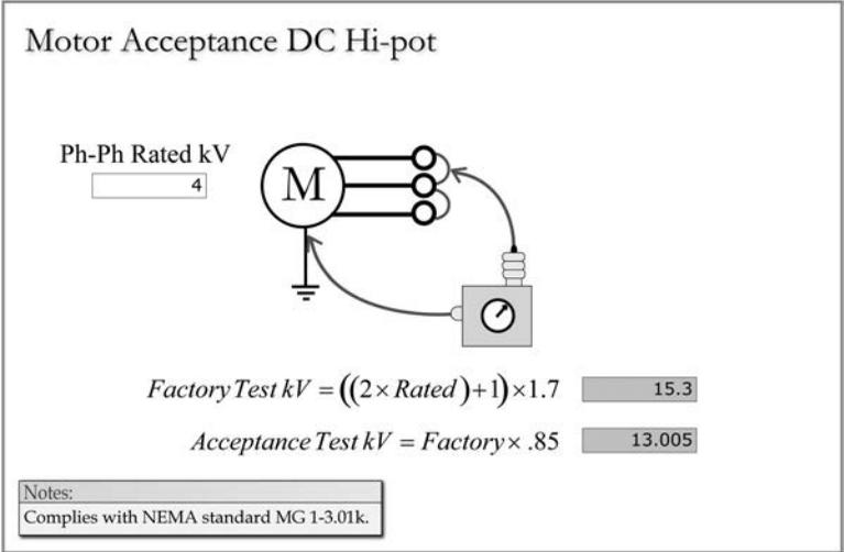
**FIGURE 5.22** Motor acceptance DC overvoltage testing.
