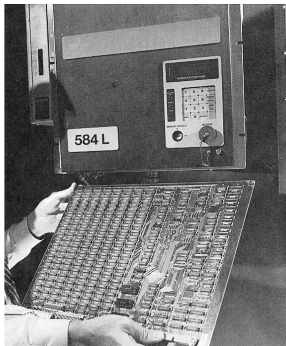
Fig. 59–7 Troubleshooting complex systems is simplified by modular construction. This industrial process controller has removable circuit boards to allow for troubleshooting and also for convenient upgrading of capabilities. (Courtesy of Schneider Electric)
