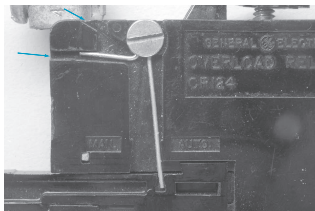
Fig. 3-18 The bimetal strip type overload relay can be set for manual or automatic reset by changing the position of the spring.
