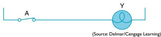
Fig. 22–8 The output of an INVERTER will always be the opposite of the input.
