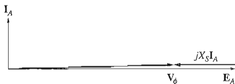
FIGURE 5-14 The phasor diagram of a synchronous capacitor or synchronous condenser .
