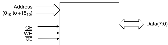
Figure 6.87: 16 address \times 8 data bit RAM
