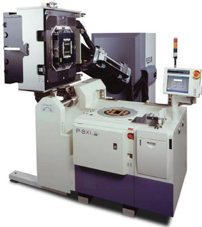
Another implementation of Fig. 1.3 is using an automatic test equipment (ATE). An ATE is an equipment that consists of processors, storage, and fixtures for mounting devices. ATEs are used for die testing, wafer testing, or testing a packaged product. An ATE runs a test program that implements the specific procedure designed for testing the DUT.
