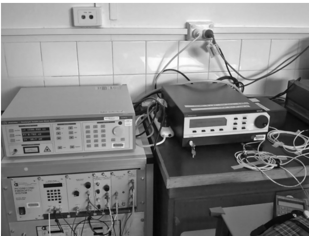
FIGURE 5.28 Laser sources. The white laser power box is used as an LO, and the black one is assumed as received optical signal.
