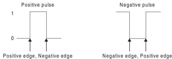
Figure 7.46 Clock pulse transition.
