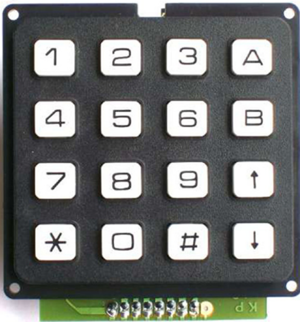
Figure 2.11 16-key matrix keyboard
