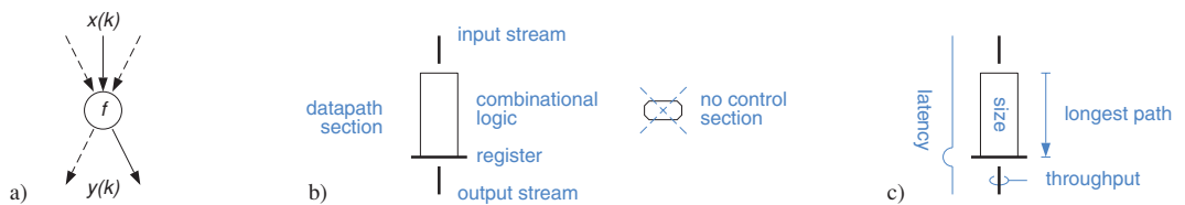
Fig. 2.12 DDG for some combinational function f (a). A symbolic representation of the reference hardware configuration (b) with its key characteristics highlighted (c).
