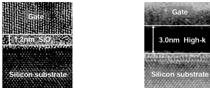
Fig. 14.30 Traditional poly-Si/SiO 2 /Si stack (90 nm, left) versus prospective metal/HfO 2 /strained-Si stack (45 nm, right) (source Intel, reprinted with permission).
