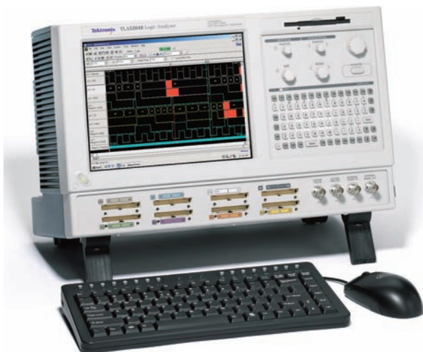
FIGURE 54 Typical logic analyzer. Used with permission from Tektronix, Inc.
