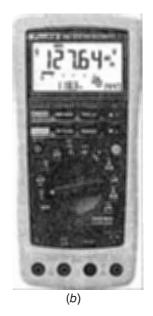
Fig. 1-3 (a) Analog meter. (b) Digital multimeter (DMM). Courtesy Fluke Corporation. Reproduced with permission
