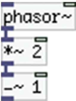
Figure 1-22. The sawtooth oscillator Pd patch
