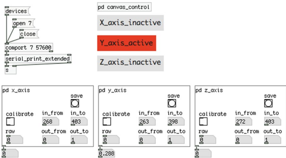
Figure 6-10. Parent patch with canvases indicating the activity of the sensor axes
