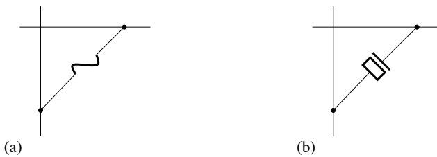
Figure 7.12. Programmable a) fuse-based and b) antifuse-based interconnects
