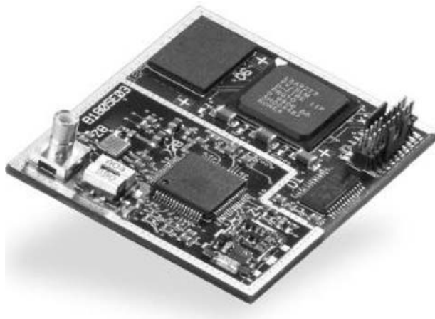
Figure 8.6 DAB module based on single chip tuner
