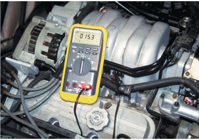
FIGURE 37-12 To measure fuel-injector resistance, a technician constructed a short wiring harness with a double banana plug that fits into the V and COM terminals of the meter and an injector connector at the other end. This setup makes checking resistance of fuel injectors quick and easy.
