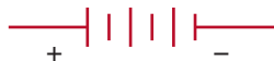
FIGURE 9-5 The symbol for a battery. The positive plate of a battery is represented by the longer line and the negative plate by the shorter line. The voltage of the battery is usually stated next to the symbol.
