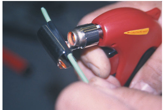
FIGURE 8-22 A butane torch especially designed for use on heat shrink applies heat without an open flame, which could cause damage.
