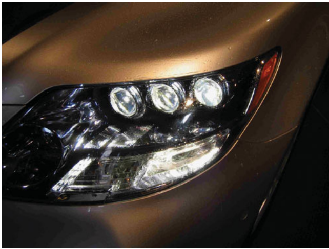
FIGURE 21-21 LED headlights usually require multiple units to provide the needed light as seen on this Lexus LS600h.
