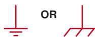
FIGURE 9-6 The ground symbol on the left represents earth ground. The ground symbol on the right represents a chassis ground.
