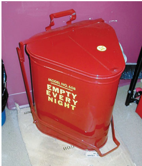
FIGURE 1-69 All oily shop cloths should be stored in a metal container equipped with a lid to help prevent spontaneous combustion.
