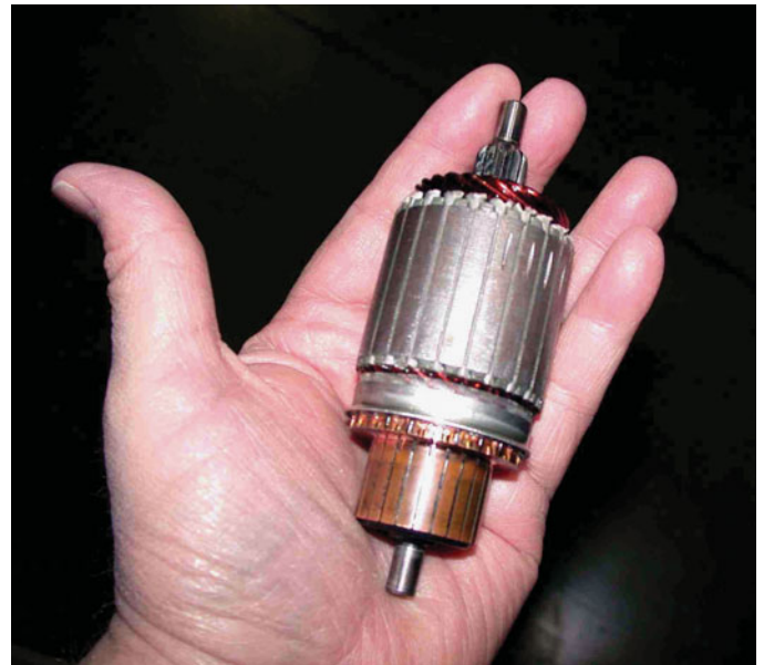
FIGURE 17-26 A palm-size starter armature.
