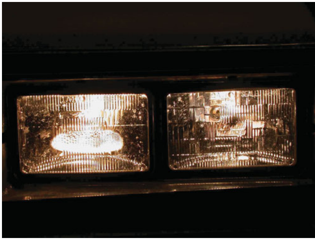
FIGURE 21-16 A typical four-headlight system using sealed beam headlights.
