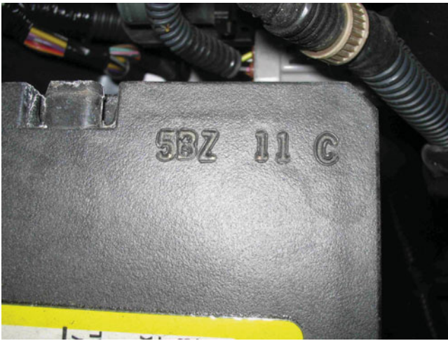
FIGURE 16-15 The code on the Delphi battery indicates that it was built in 2005 (5), in February (B), on the eleventh day (11), during third shift (C), and in the Canadian plant (Z).
