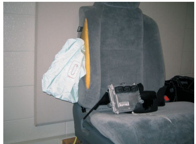
FIGURE 25-24 A typical seat (side) airbag that deploys from the side of the seat.
