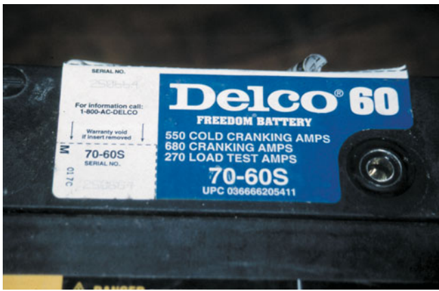
FIGURE 16-6 This battery has cold-cranking amperes (CCA) of 550 A, cranking amperes (CA) of 680 A, and load test amperes of 270 A listed on the top label. Not all batteries have this complete information.
