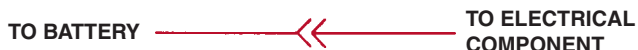
FIGURE 9-4 In this typical connector, note that the positive terminal is usually a female connector.
