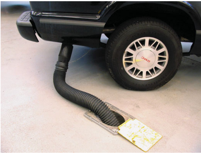
FIGURE 1-66 Always connect an exhaust hose to the tailpipe of a vehicle to be run inside a building.
