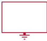
FIGURE 9-21 This symbol represents a component that is case grounded.
