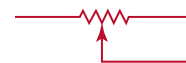
FIGURE 9-16 A rheostat uses only two wires—one is connected to a voltage source and the other is attached to the movable arm.
