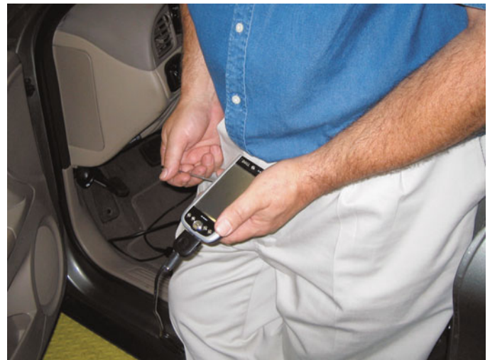
FIGURE 40-12 Some scan tools use pocket PCs which make it very convenient to use.
