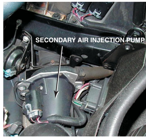
FIGURE 39-21 A typical electric motor-driven SAI pump. This unit is on a Chevrolet Corvette and only works when the engine is cold.
