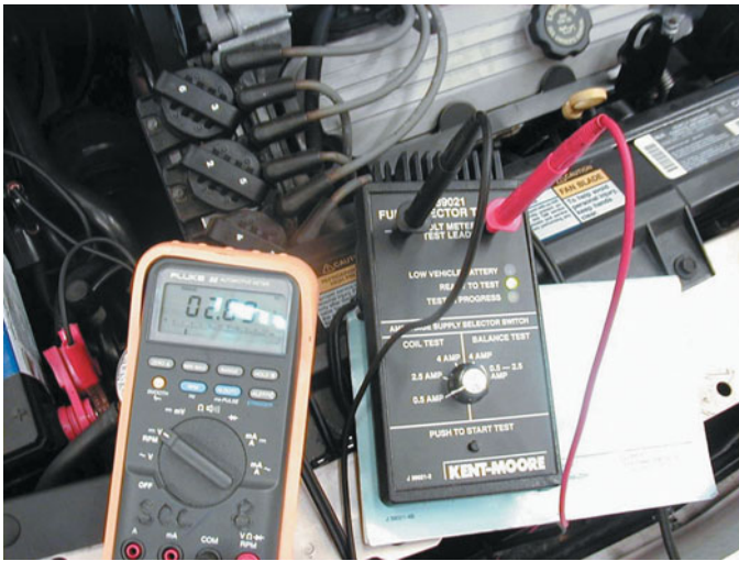
FIGURE 37-16 An injector tester being used to check the voltage drop through the injector while the tester is sending current through the injectors. This test is used to check the coil inside the injector. This same tester can be used to check for equal pressure drop of each injector by pulsing the injector on for 500 ms.
