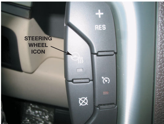
FIGURE 24–21 The heated steering wheel is controlled by a switch on the steering wheel in this vehicle.
