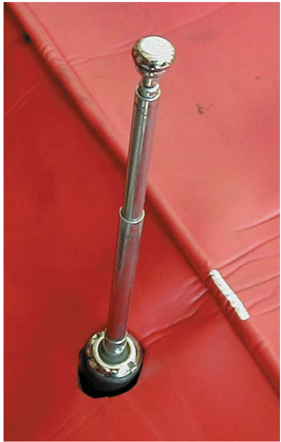
FIGURE 26-9 Cutting a small hole in a fender cover helps to protect the vehicle when replacing or servicing an antenna.
