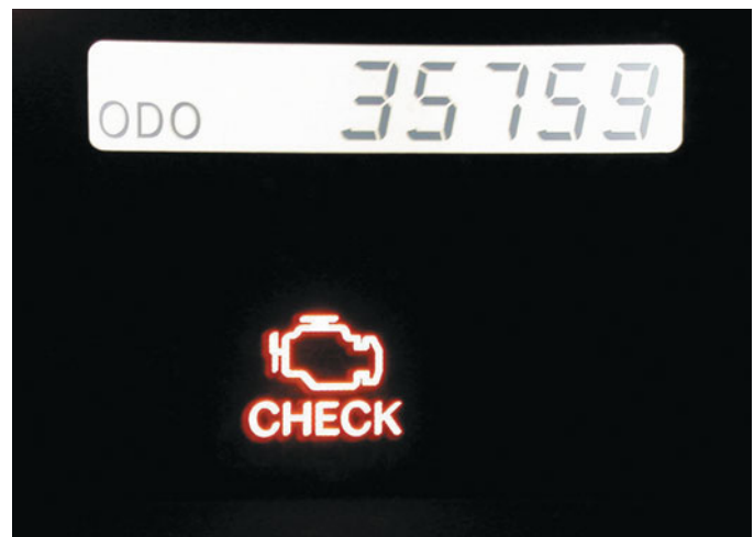
FIGURE 27-1 A typical malfunction indicator lamp (MIL) often labeled “check engine” or “service engine soon” (SES).
