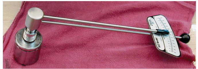
FIGURE 1-27 A beam-type torque wrench that displays the torque reading on the face of the dial. The beam display is read as the beam deflects, which is in proportion to the amount of torque applied to the fastener.
