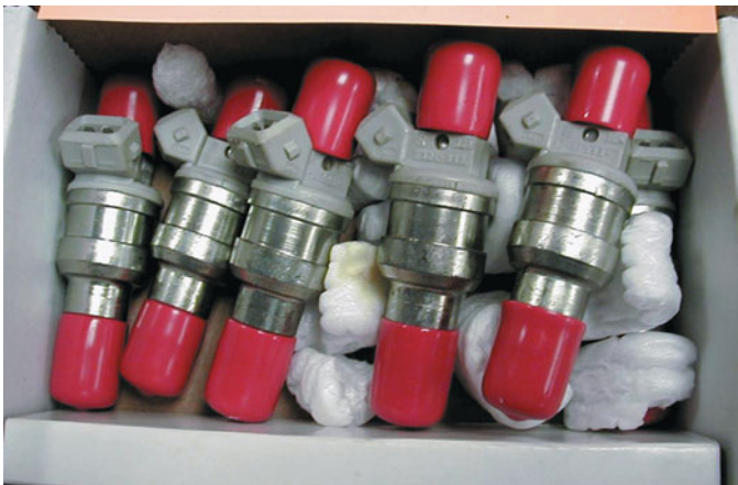
FIGURE 37-20 A set of six reconditioned injectors. The sixth injector is barely visible at the far right.
