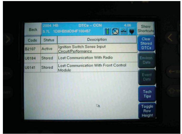
FIGURE 14-22 A Honda scan display showing a B and two U codes, all indicating a BUS-related problem(s).
