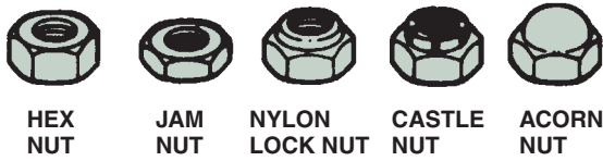
FIGURE 1-13 Nuts come in a variety of styles, including locking (prevailing torque) types, such as the distorted thread and nylon insert type.
