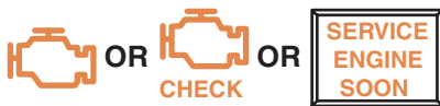
FIGURE 22-5 Malfunction indicator lamp (MIL), also called a check engine light. The light means the engine control computer has detected a fault.
