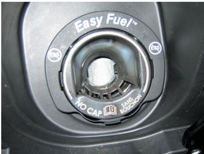
FIGURE 39-29 A capless system from a Ford Flex does not use a replaceable cap; instead, it has a spring-loaded closure.
