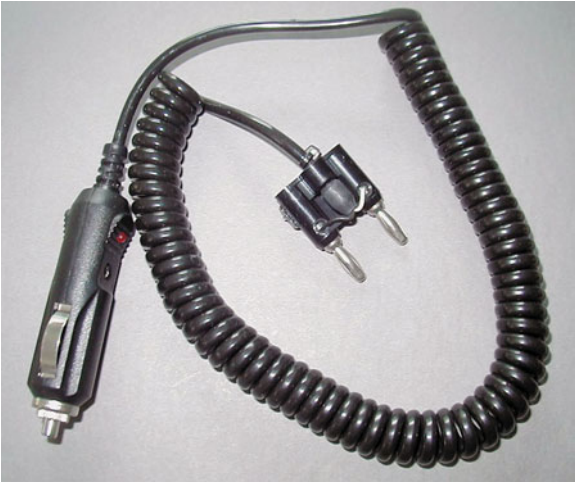
FIGURE 20-8 Charging system voltage can be easily checked at the lighter plug by connecting a lighter plug to the voltmeter through a double banana plug.
