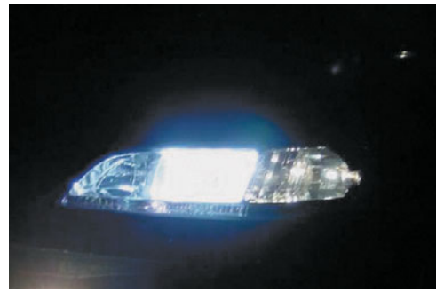
FIGURE 21-20 HID (xenon) headlights emit a whiter light than halogen headlights and usually look blue compared to halogen bulbs.
