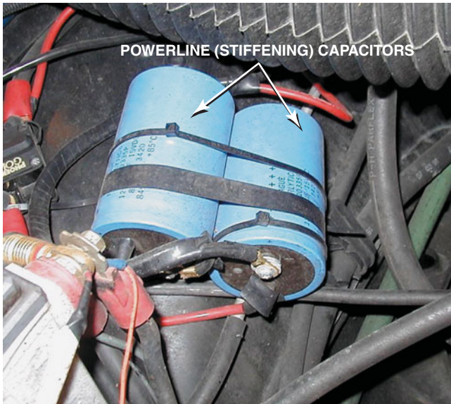
FIGURE 26-15 Two capacitors connected in parallel provide the necessary current flow to power large subwoofer speakers.
