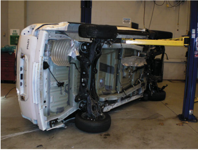
FIGURE 1-72 This training vehicle fell from the hoist because the pads were not set correctly. No one was hurt, but the vehicle was damaged.
