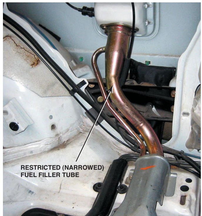
FIGURE 39-34 A restricted fuel fill pipe shown on a vehicle with the interior removed.
