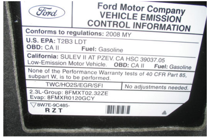
FIGURE 1-2 The vehicle emissions control information (VECI) sticker is placed under the hood.
