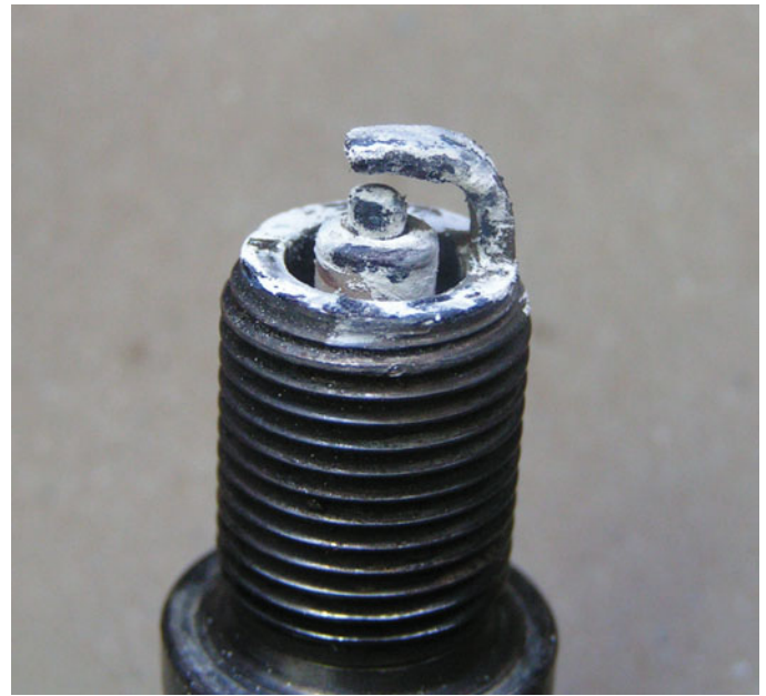
FIGURE 33-40 A spark plug from an engine that had a blown head gasket. The white deposits could be from the aluminum of the position or from the additives in the coolant.
