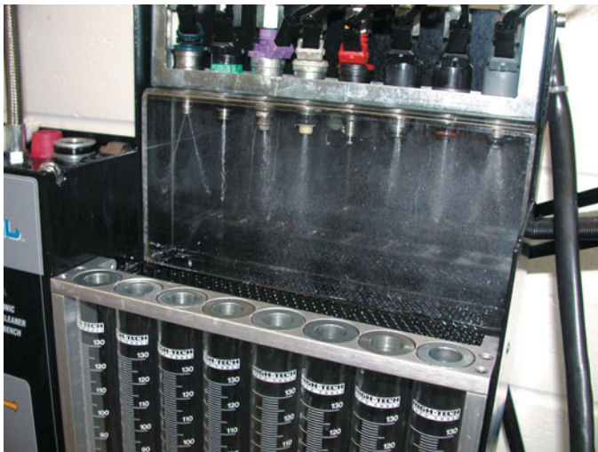
FIGURE 35-17 Each of the eight injectors shown are producing a correct spray pattern for the applications. While all throttle-body injectors spray a conical pattern, most port fuel injections do not.
