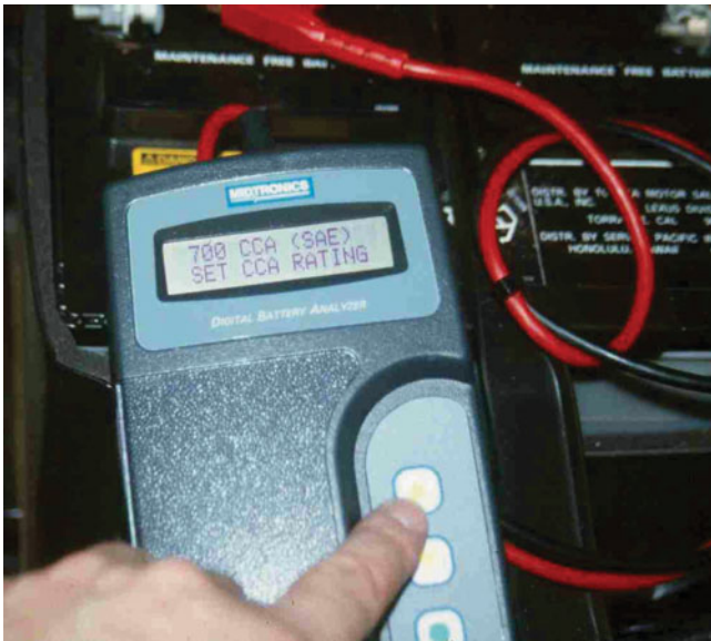
FIGURE 16-10 A conductance tester is very easy to use and has proved to accurately determine battery condition if the connections are properly made. Follow the instructions on the display exactly for best results.
