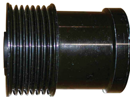
FIGURE 20-6 This overrunning alternator dampener (OAD) is longer than an overrunning alternator pulley (OAP) because it contains a dampener spring as well as a one way clutch. Be sure to check that it locks in one direction.
