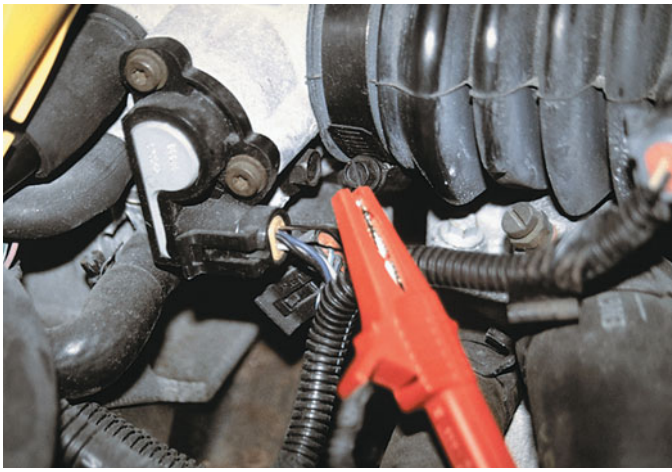
FIGURE 29-3 A meter lead connected to a T-pin that was gently pushed along the signal wire of the TP sensor until the point of the pin touched the metal terminal inside the plastic connector.
