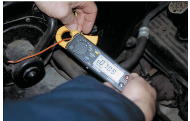
FIGURE 23-22 Using a mini AC/DC clamp-on multimeter to measure the current draw of a blower motor.
