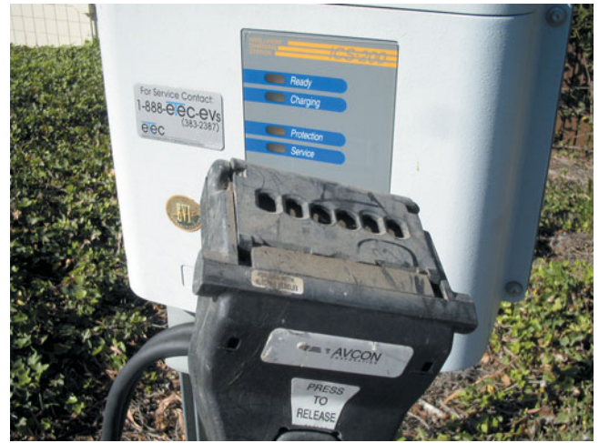
FIGURE 42-29 A conductive-type charging connector. This type of battery charging connector is sometimes called an AVCON connector, named for the manufacturer.
