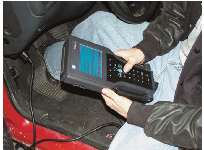
FIGURE 40-11 A TECH 2 scan tool is the factory scan tool used on General Motors vehicles.
