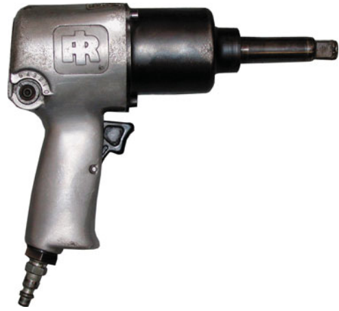
FIGURE 1-55 A typical 1/2 in. drive air impact wrench. The direction of rotation can be changed to loosen or tighten a fastener.
