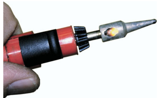
FIGURE 8-19 A butane-powered soldering tool. The cap has a built-in striker to light a converter in the tip of the tool. This handy soldering tool produces the equivalent of 60 watts of heat. It operates for about 1/2 hour on one charge from a commonly available butane refill dispenser.
