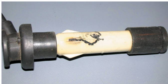
FIGURE 33-30 This spark plug boot on an overhead camshaft engine has been arcing to the valve cover causing a misfire to occur.
