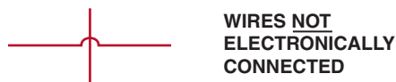
FIGURE 9-10 Wires that cross, but do not electrically contact each other, are shown with one wire bridging over the other.
