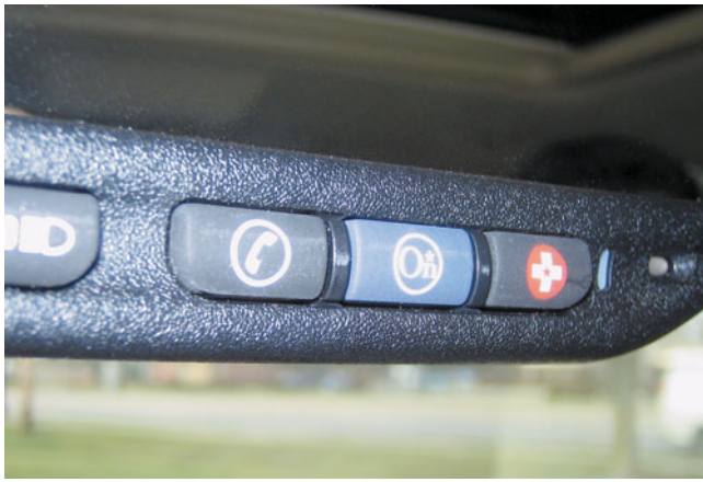
FIGURE 22-47 The three-button OnStar control is located on the inside rearview mirror. The left button (telephone handset icon) is pushed if a hands-free cellular call is to be made. The center button is depressed to contact an OnStar advisor and the right emergency button is used to request that help be sent to the vehicle's location.
