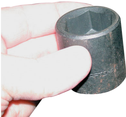
FIGURE 1-57 A black impact socket. Always use an impact-type socket whenever using an impact wrench to avoid the possibility of shattering the socket, which could cause personal injury.
