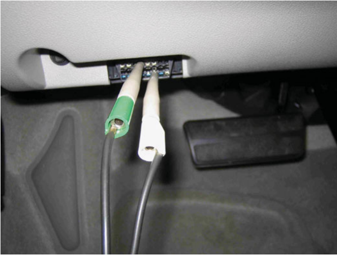
FIGURE 14–28 Use front-probe terminals to access the data link connector. Always follow the specified back-probe and front-probe procedures as found in service information.
