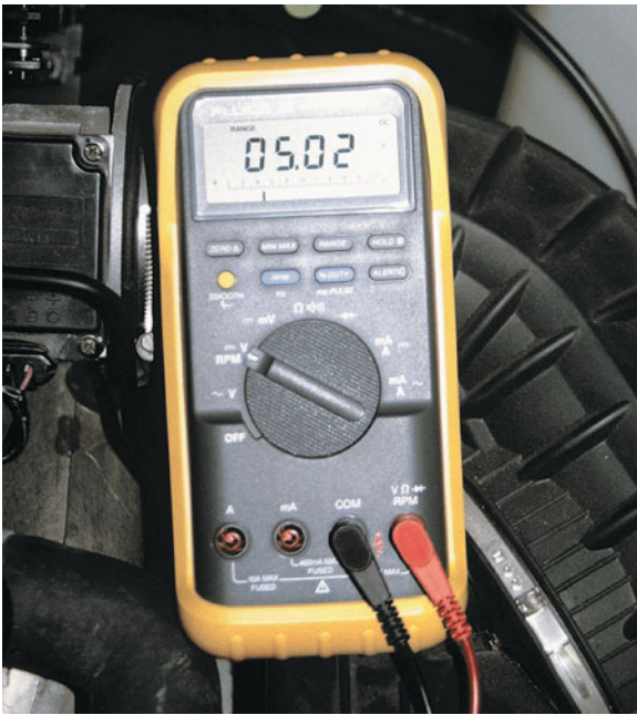
FIGURE 29-5 Checking the 5-volt reference from the computer being applied to the TP sensor with the ignition switch on (engine off). The reading for this vehicle (5.02 volts DC) is within the normal range for the 5-volt reference voltage of 4.9 to 5.1 volts.
