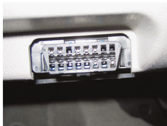
FIGURE 40-16 A typical OBD-II data link connector (DLC). The location varies with make and model and may even be covered, but a tool is not needed to gain access. Check service information for the exact location if needed.
