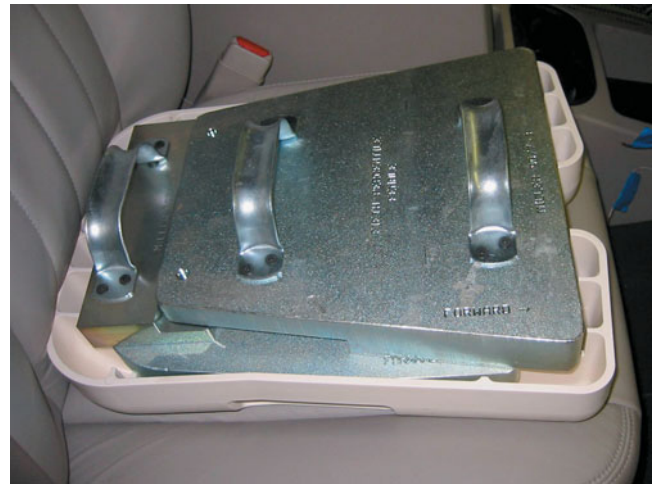
FIGURE 25-23 A test weight is used to calibrate the occupant detection system on a Chrysler vehicle.
