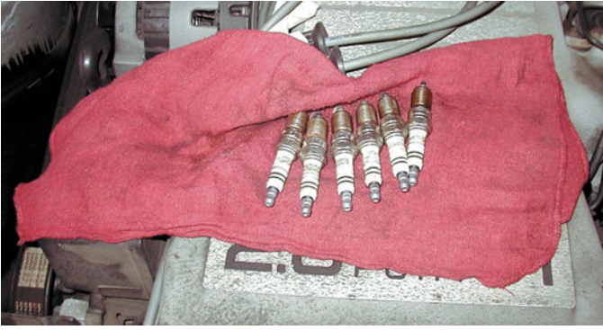
FIGURE 33-36 When removing spark plugs, it is wise to arrange them so that they can be compared and any problem can be identified with a particular cylinder.
