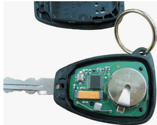
FIGURE 24-26 A key fob remote with the cover removed showing the replaceable battery.
