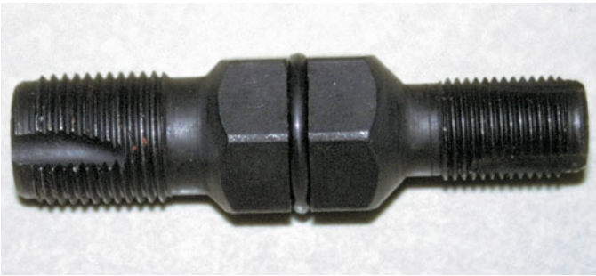
FIGURE 33-37 A spark plug thread chaser is a low-cost tool that hopefully will not be used often, but is necessary to use to clean the threads before new spark plugs are installed.
