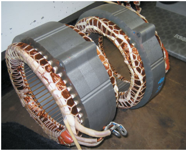
FIGURE 42-15 Drive motors in fuel-cell hybrid vehicles often use stator assemblies similar to ones found in Toyota hybrid electric vehicles. The rotor turns inside the stator and has permanent magnets on its outer circumference.
