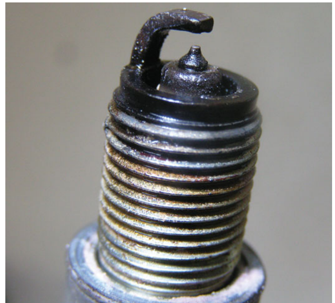
FIGURE 33-41 A platinum tipped spark plug that is fuel soaked indicating a fault with the fuel system or the ignition system causing the spark plug to not fire.
