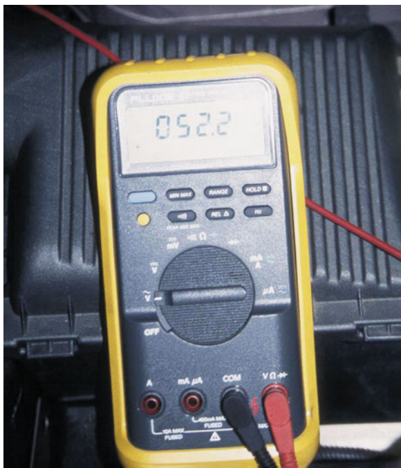
FIGURE 6-19 This meter display shows 052.2 AC volts. Notice that the zero beside the 5 indicates that the meter can read over 100 volts AC with a resolution of 0.1 volt.
