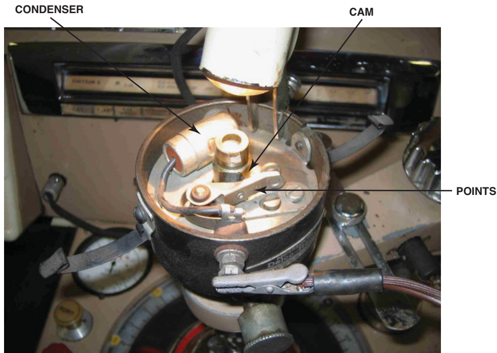
FIGURE 10-7 A point-type distributor shown with the condenser from an old vehicle being tested on a distributor machine.
