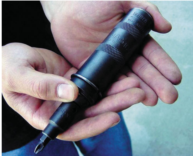
FIGURE 1-32 An impact screwdriver used to remove slotted or Phillips head fasteners that cannot be broken loose using a standard screwdriver.
