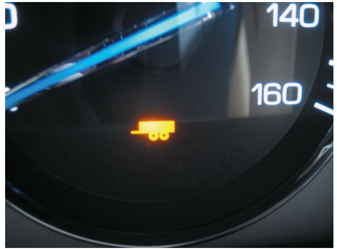
FIGURE 24-5 A trailer icon lights on the dash of this Cadillac when the transmission trailer towing mode is selected.
