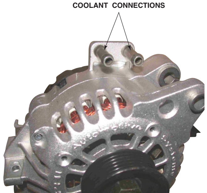
FIGURE 19-20 A coolant-cooled alternator showing the hose connections where coolant from the engine flows through the rear frame of the alternator.
