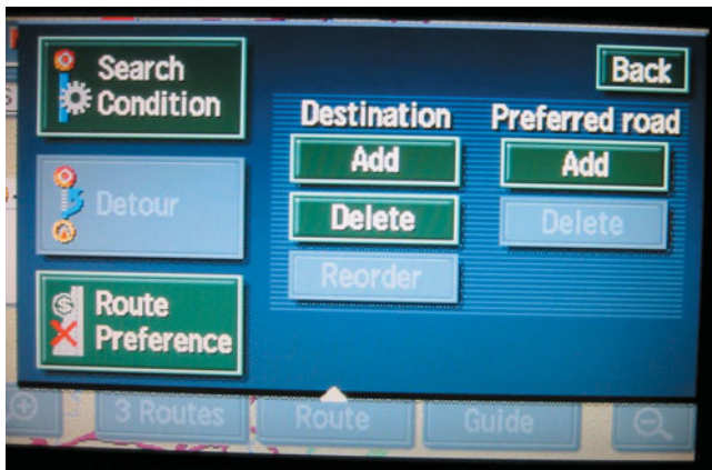
FIGURE 22-45 A typical navigation display showing various options. Some systems do not allow access to these functions if the vehicle is in gear and/or moving.
