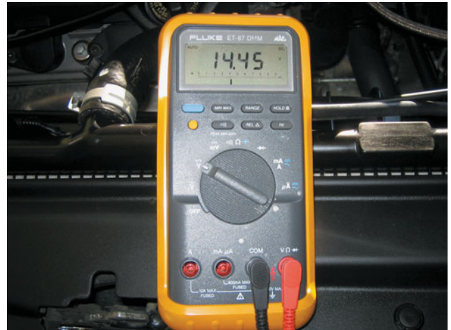
FIGURE 20-1 The digital multimeter should be set to read DC volts, with the red lead connected to the positive (+) battery terminal and the black meter lead connected to the negative (-) battery terminal.
