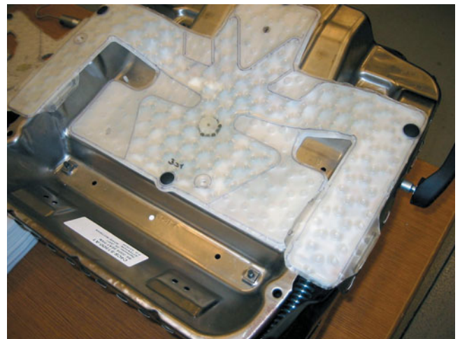
FIGURE 25-21 A gel-filled (bladder-type) occupant detection sensor showing the pressure sensor and wiring.
