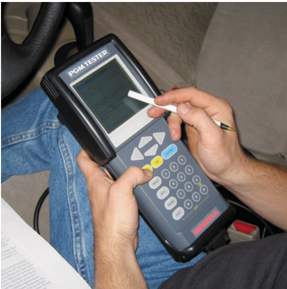
FIGURE 20-2 A scan tool can be used to diagnose charging system problems.
