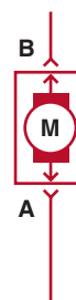
FIGURE 9-14 An electric motor symbol shows a circle with the letter M in the center and two black sections that represent the brushes of the motor. This symbol is used even though the motor is a brushless design.
