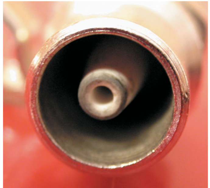
FIGURE 33-23 A close-up showing the recessed center electrode on a spark tester. It is recessed 3/8 in. into the shell and the spark must then jump another 3/8 in. to the shell for a total gap of 3/4 in.
