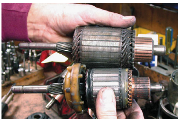
9 Notice that the length of a direct-drive starter armature (top) is the same length as the overall length of a gear-reduction armature except smaller in diameter.
