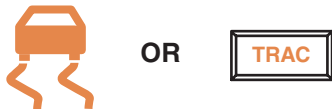
FIGURE 22-19 Low traction detected. Traction control system is functioning to restore traction (usually flashes when actively working to restore traction).
