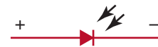
FIGURE 12-16 Symbol for a photodiode. The arrows represent light striking the P-N junction of the photodiode.
