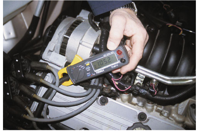
FIGURE 20-9 A mini clamp-on meter can be used to measure alternator output as shown here (105.2 Amp.). Then the meter can be used to check AC current ripple by selecting AC Amps on the rotary dial. AC ripple current should be less than 10% of the DC current output.
