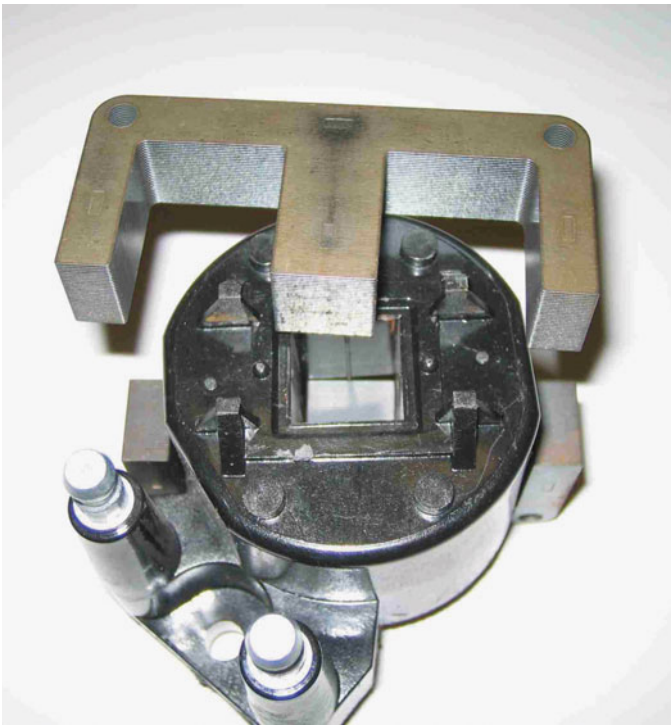
FIGURE 11-21 A GM waste-spark ignition coil showing the section of laminations that is shaped like the letter E . These mild steel laminations improve the efficiency of the coil.
