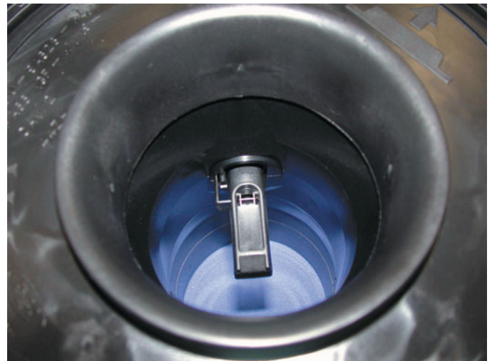
FIGURE 31-4 The sensing wire in a typical hot wire mass air flow sensor.
