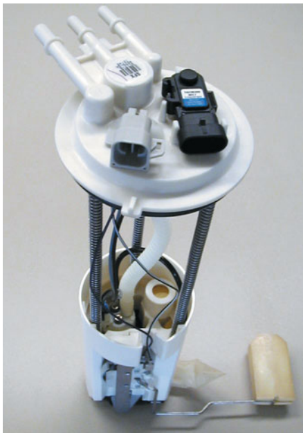
FIGURE 34-16 A typical fuel-pump module assembly, which includes the pickup strainer and fuel pump, as well as the fuel-pressure sensor and fuel level sensing unit.
