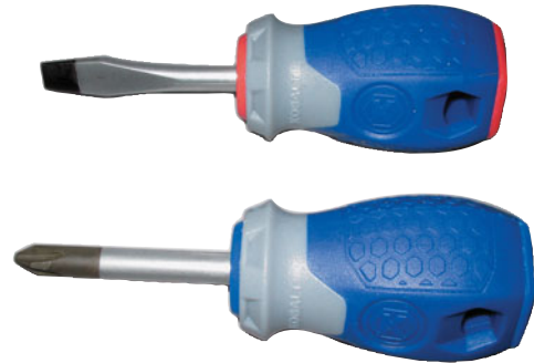
FIGURE 1-30 Two stubby screwdrivers used to access screws that have limited space above. A straight blade is on top and a #2 Phillips screwdriver is on the bottom.
