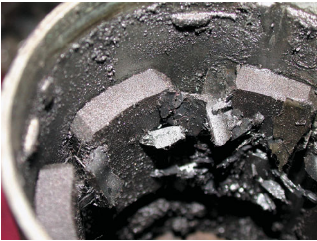
FIGURE 17-19 This starter permanent magnet field housing was ruined when someone used a hammer on the field housing in an attempt to “fix” a starter that would not work. A total replacement is the only solution in this case.
