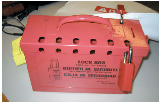
FIGURE 41-10 A lock box is a safe location to keep the ignition keys of a hybrid electric vehicle while it is being serviced.
