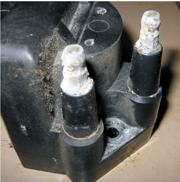
FIGURE 33-29 Corroded terminals on a waste-spark coil can cause misfire diagnostic trouble codes to be set.
