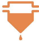
FIGURE 22-3 Water detected in fuel. Notice to drain the water from the fuel filter assembly on a vehicle equipped with a diesel engine.
