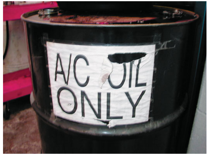
FIGURE 2-9 Air-conditioning refrigerant oil must be kept separated from other oils because it contains traces of refrigerant and must be treated as hazardous waste.
