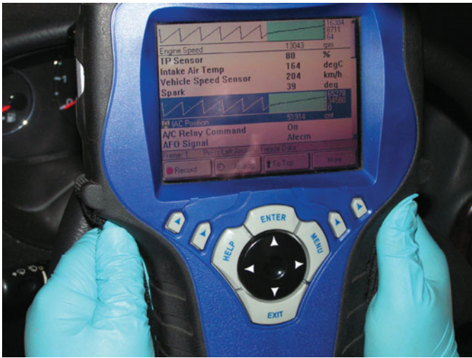
FIGURE 37-6 Using a scan tool to check for IAC counts or percentage as part of a diagnostic routine.
