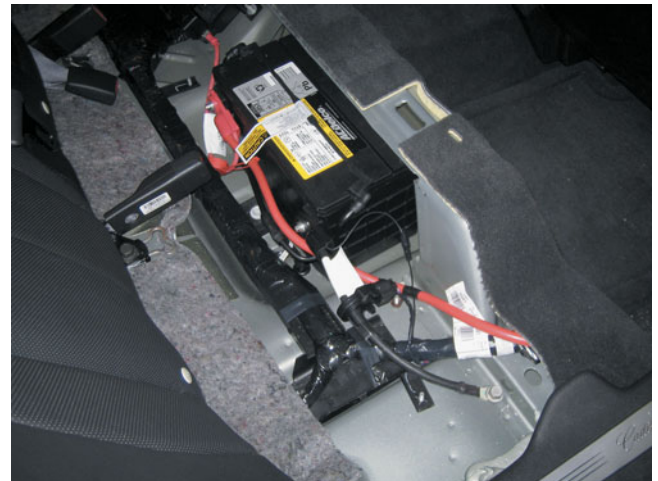
FIGURE 16-20 Many newer vehicles have batteries that are sometimes difficult to find. Some are located under plastic panels under the hood, under the front fender, or even under the rear seat as shown here. The jump-start instructions indicate that the spare tire hold-down bolt is to be used as the ground connection if jump starting is necessary.
