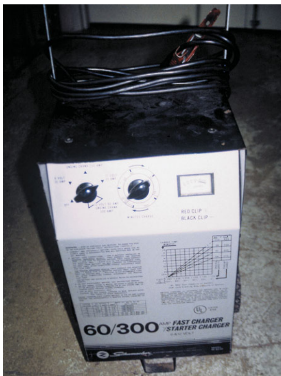
FIGURE 16-11 A typical industrial battery charger. Be sure that the ignition switch is in the off position before connecting any battery charger. Connect the cables of the charger to the battery before plugging the charger into the outlet. This helps prevent a voltage spike and spark that could occur if the charger happened to be accidentally left on. Always follow the battery charger manufacturer's instructions.
