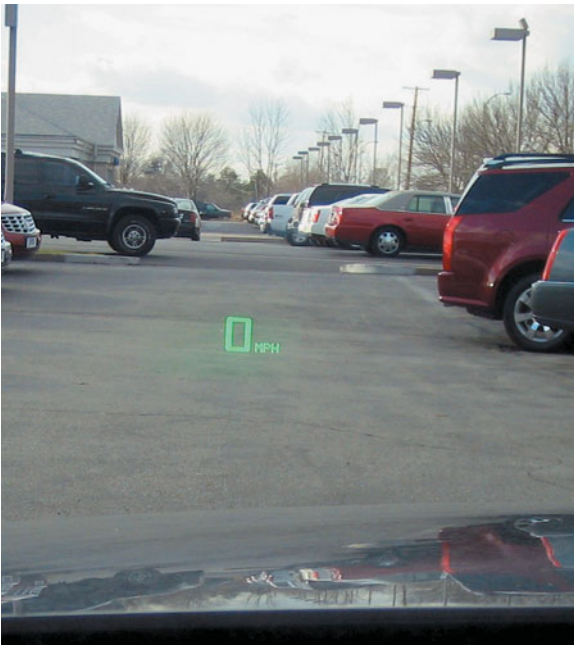
FIGURE 22-31 A typical head-up display showing zero miles per hour, which is actually projected on the windshield from the head-up display in the dash.
