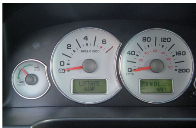
FIGURE 41-6 The Ford Escape Hybrid instrument panel showing the vehicle in park and the tachometer on “EV” instead of 0 RPM. This means that the gasoline engine could start at any time depending on the state-of-charge of the high-voltage batteries and other factors.
