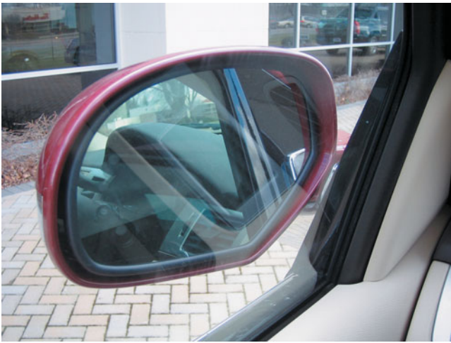
FIGURE 24-23 Electrically folded mirror in the folded position.
