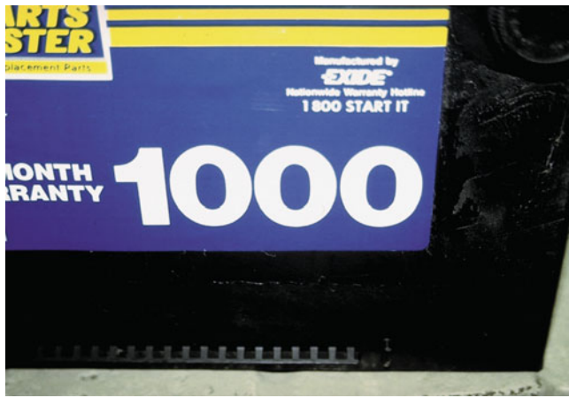
FIGURE 15-11 This battery has a cranking amperes (CA) rating of 1,000. This means that this battery is capable of cranking an engine for 30 seconds at a temperature of 32°F (0°C) at a minimum of 1.2 volts per cell (7.2 volts for a 12 volt battery).
