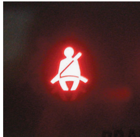
FIGURE 25-3 A typical safety belt warning light.
