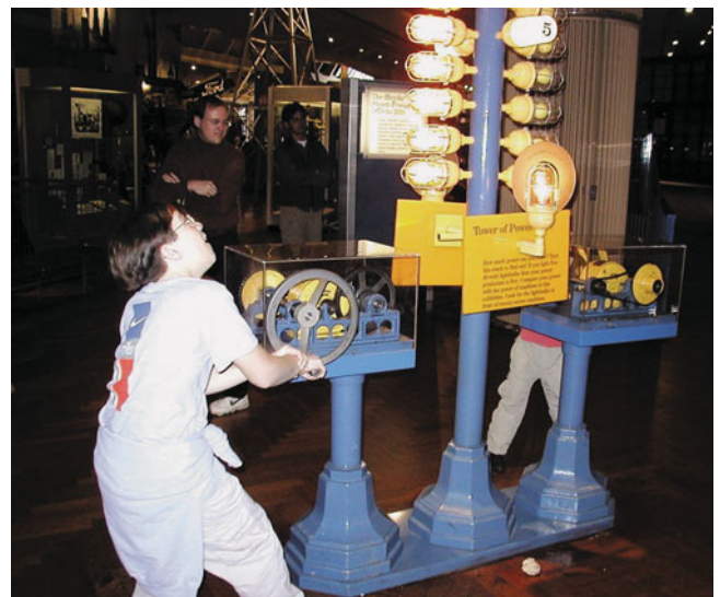
FIGURE 3-20 A display at the Henry Ford Museum in Dearborn, Michigan, which includes a hand-cranked generator and a series of light bulbs. This figure shows a young man attempting to light as many bulbs as possible. The crank gets harder to turn as more bulbs light because it requires more power to produce the necessary watts of electricity.
