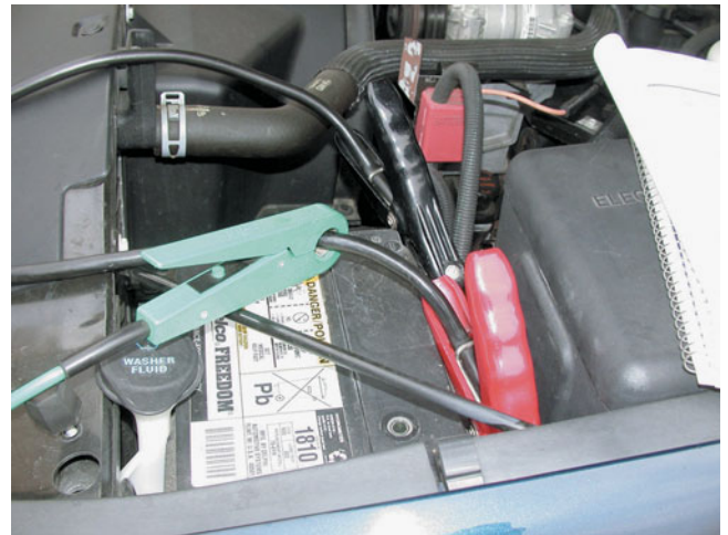
FIGURE 6-14 An inductive ammeter clamp is used with all starting and charging testers to measure the current flow through the battery cables.
