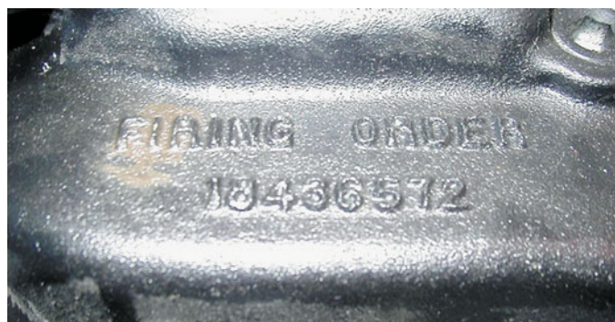
FIGURE 33-12 The firing order is cast or stamped on the intake manifold on most engines that have a distributor ignition.
