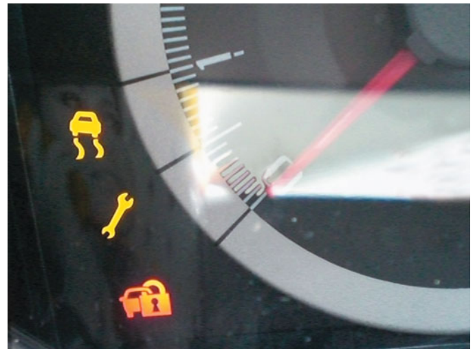
FIGURE 36-9 A wrench symbol warning lamp on a Ford vehicle. The symbol can also be green.
