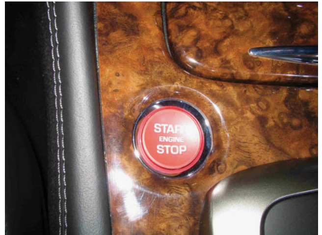
FIGURE 17-4 Instead of using an ignition key to start the engine, some vehicles are using a start button which is also used to stop the engine, as shown on this Jaguar.
