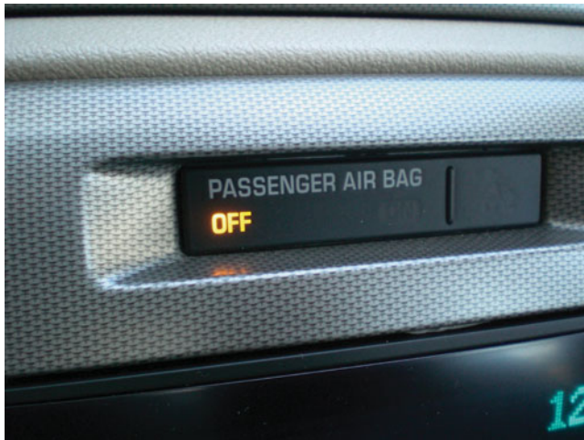
FIGURE 25-19 A dash warning lamp will light if the passenger side airbag is off because no passenger was detected by the seat sensor.
