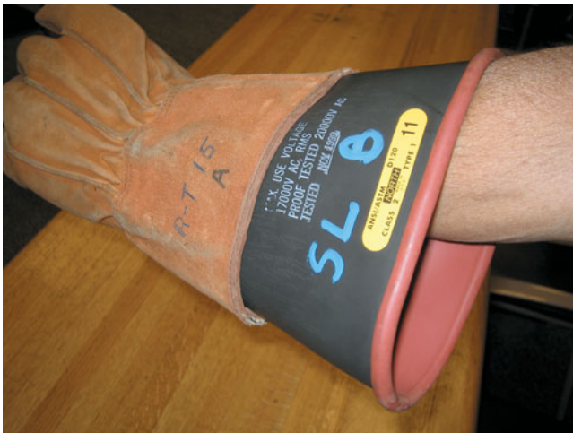
FIGURE 41-2 Wearing leather gloves over the lineman's gloves helps protect the rubber gloves from damage.
