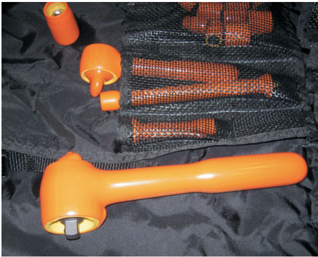
FIGURE 41-11 Insulated tools, such as this socket set, would provide an additional margin of safety to the service technician when working around high-voltage components and systems.
