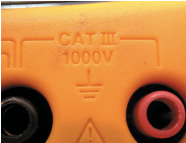
FIGURE 41-4 Be sure to only use a meter that is CAT III-rated when taking electrical voltage measurements on a hybrid electric or electric vehicle.
