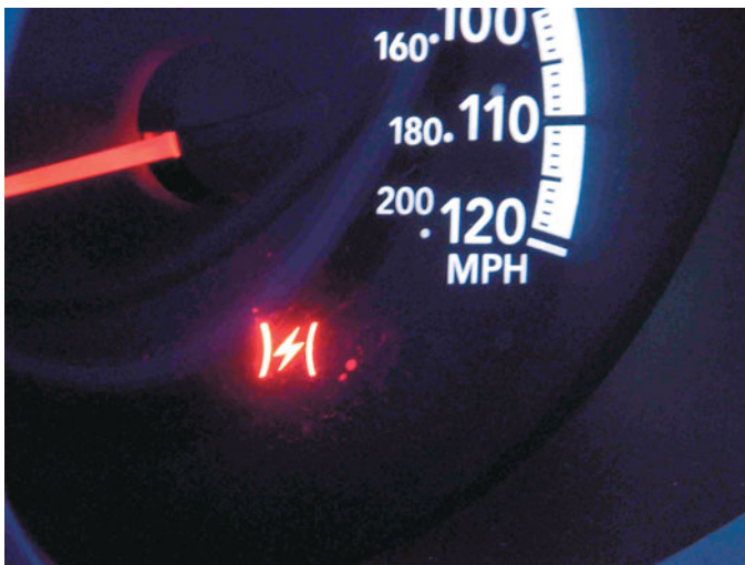
FIGURE 36-10 A symbol used on a Chrysler vehicle indicating a fault with the electronic throttle control.
