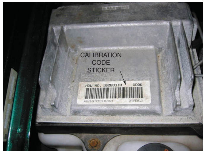
FIGURE 1-3 A typical calibration code sticker on the case of a controller. The information on the sticker is often needed when ordering parts or a replacement controller.
