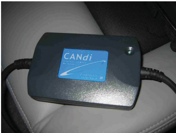
FIGURE 14-12 A CANdi module will flash the green LED rapidly if communication is detected.
