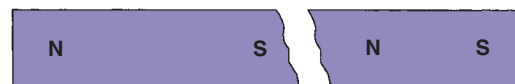
FIGURE 11-2 If a magnet breaks or is cracked, it becomes two weaker magnets.
