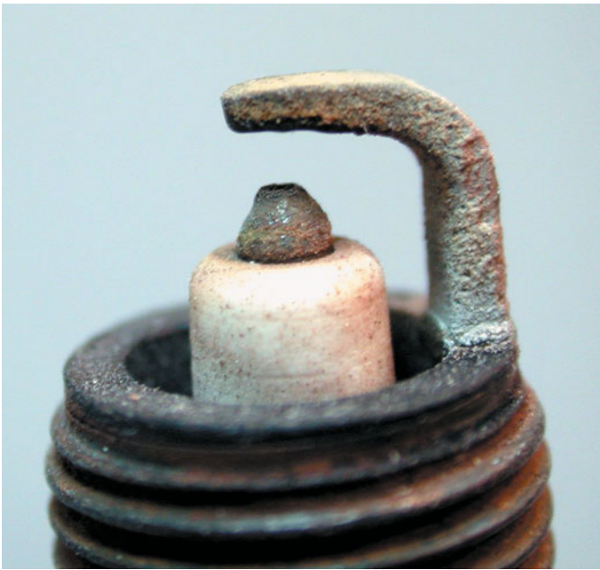
FIGURE 33-38 A normally worn spark plug that uses a tapered platinum-tipped center electrode.
