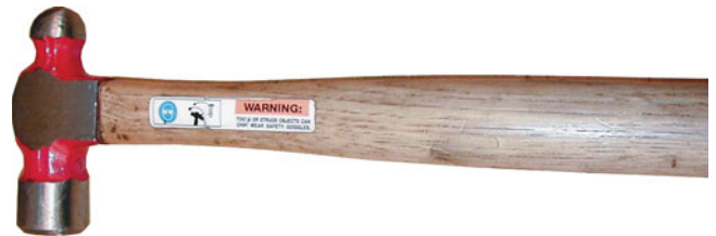
FIGURE 1-33 A typical ball-peen hammer.
