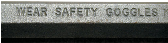
FIGURE 1-47 Warning stamped in the side of a punch that goggles should be worn when using this tool. Always follow safety warnings.
