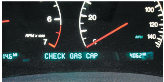
FIGURE 39-35 Some vehicles will display a message if an evaporative control system leak is detected that could be the result of a loose gas cap.
