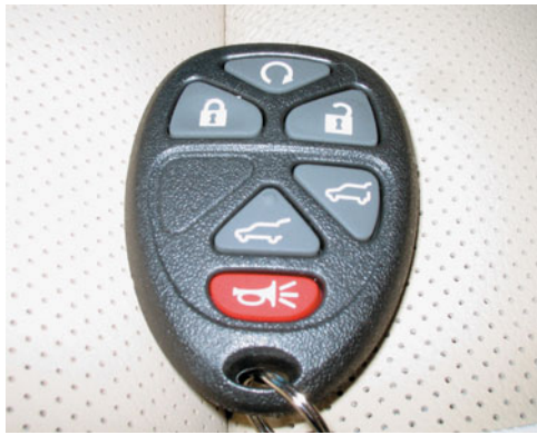
FIGURE 17-5 The top button on this key fob is the remote start button.
