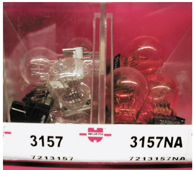
FIGURE 21-2 Bulbs that have the same trade number have the same operating voltage and wattage. The NA means that the bulb uses a natural amber glass ampoule with clear turn signal lenses.
