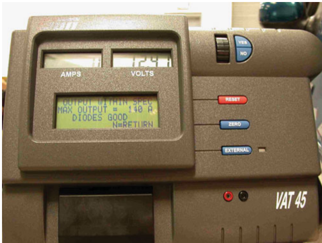
FIGURE 20-11 A typical tester used to test batteries as well as the cranking and charging system. Always follow the operating instructions.
