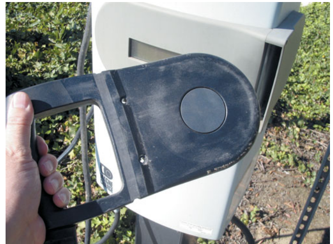
FIGURE 42-30 An inductive-type electric vehicle battery charger connector. This type of connector fits into a charging slot in the vehicle, but does not make electrical contact.
