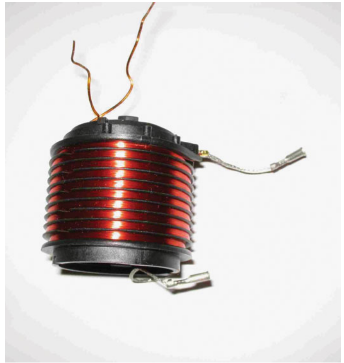
FIGURE 11-22 The coil-on-plug (COP) design typically uses a bobbin-type coil.
