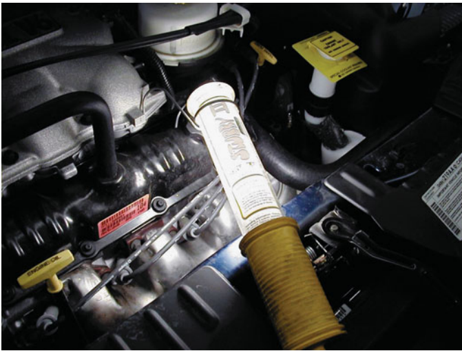
FIGURE 1-54 A fluorescent trouble light operates cooler and is safer to use in the shop because it is protected against accidental breakage where gasoline or other flammable liquids would happen to come in contact with the light.
