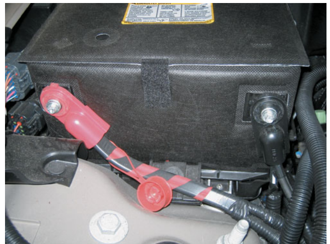
FIGURE 8-2 Battery cables are designed to carry heavy starter current and are therefore usually 4 gauge or larger wire. Note that this battery has a thermal blanket covering to help protect the battery from high underhood temperatures. The wiring is also covered with plastic conduit called split-loom tubing.
