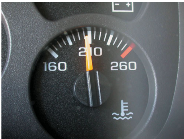
FIGURE 22-24 A temperature gauge showing normal operating temperature between 180°F and 215°F, depending on the specific vehicle and engine.
