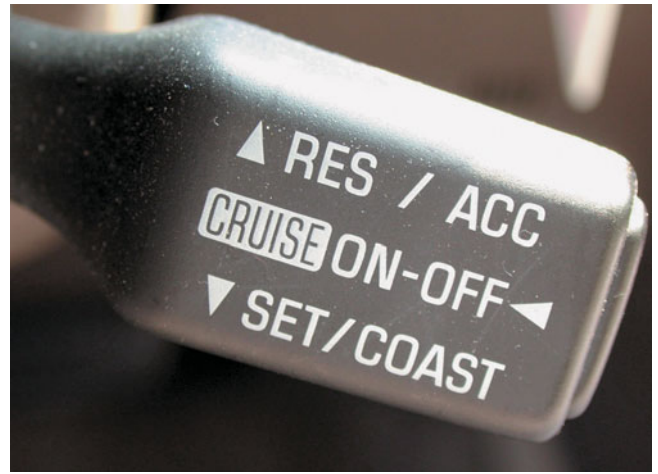
FIGURE 24-2 A cruise control used on a Toyota/Lexus.
