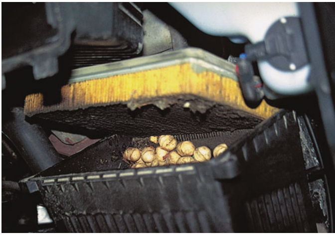
FIGURE 40-4 This is what was found when removing an air filter from a vehicle that had a lack-of-power concern. Obviously the nuts were deposited by squirrels or some other animal, blocking a lot of the airflow into the engine.
