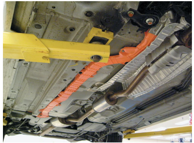
FIGURE 41-12 The high-voltage wiring on this Honda hybrid is colored orange for easy identification.
