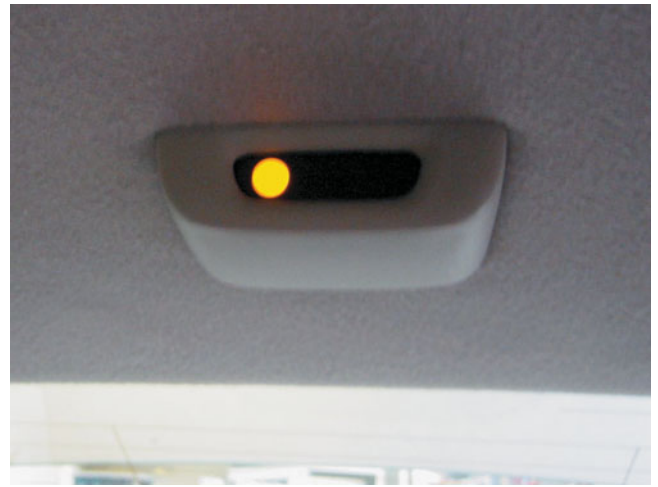
FIGURE 22-50 A typical backup sensor display located above the rear window inside the vehicle. The warning lights are visible in the inside rearview mirror.
