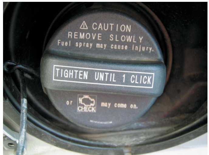
FIGURE 39-40 This Toyota cap has a warning. The check engine light will come on if not tightened until one click.
