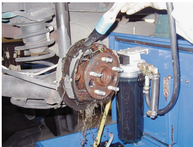
FIGURE 2-2 All brakes should be moistened with water or solvent to help prevent brake dust from becoming airborne.
