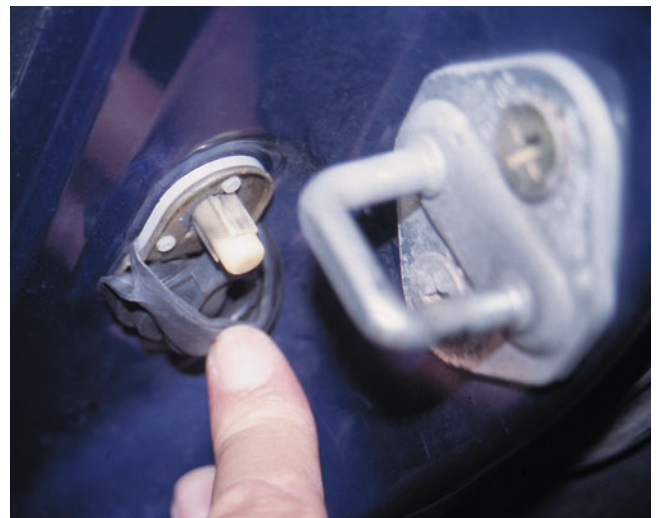
FIGURE 21-29 A typical courtesy light doorjamb switch. Newer vehicles use the door switch as an input to the vehicle computer and the computer turns the interior lights on or off. By placing the lights under the control of the computer, the vehicle engineers have the opportunity to delay the lights after the door is closed and to shut them off after a period of time to avoid draining the battery.
