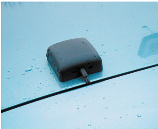
FIGURE 26-21 An aftermarket XM radio antenna mounted on the rear deck lid. The deck lid acts as the ground plane for the antenna.
