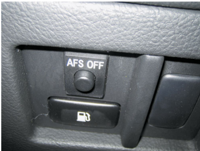
FIGURE 21-26 Typical dash-mounted switch that allows the driver to disable the front lighting system.
