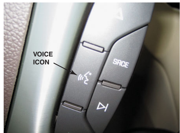
FIGURE 26-18 The voice command icon on the steering wheel of a Cadillac.
