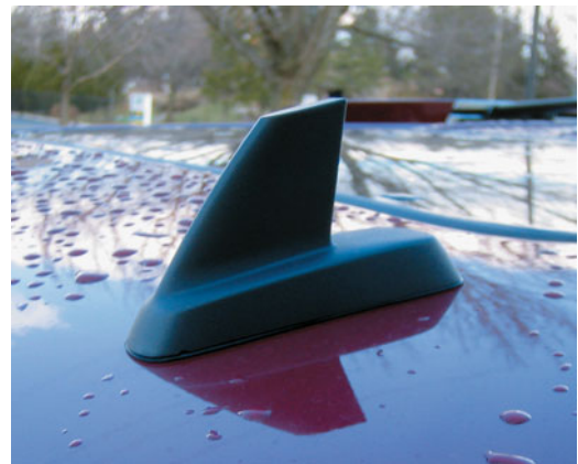
FIGURE 26-22 A shark-fin-type factory antenna used for both XM and OnStar.
