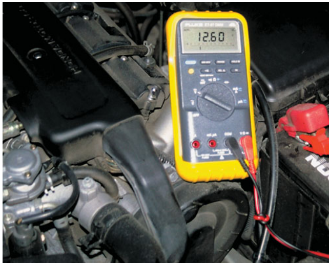
FIGURE 3-18 This digital multimeter set to read DC volts is being used to test the voltage of a vehicle battery. Most multimeters can also measure resistance (ohms) and current flow (amperes).
