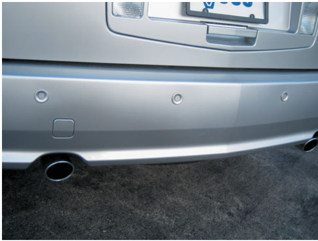
FIGURE 22-51 The small round buttons in the rear bumper are ultrasonic sensors used to sense distance to an object.
