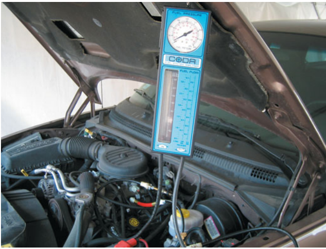
FIGURE 34–27 A fuel system tester connected in series in the fuel system so all of the fuel used flows through the meter which displays the rate-of-flow and the fuel pressure.
