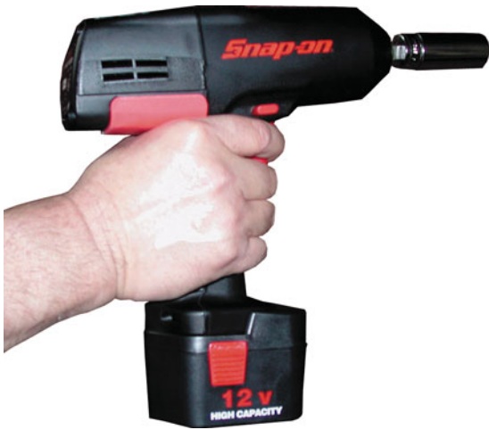
FIGURE 1-56 A typical battery-powered 3/8 in. drive impact wrench.
