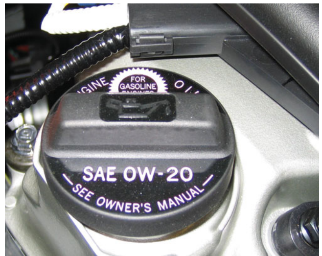
FIGURE 41-14 Always use the specified viscosity of oil in a hybrid electric vehicle not only for best fuel economy but also because of the need for fast lubrication because of the engine (idle) stop feature.
