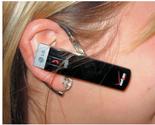
FIGURE 26-19 Bluetooth earpiece that contains a microphone and speaker unit that is paired to a cellular phone. The telephone has to be within 33 ft (10 m) of the earpiece.
