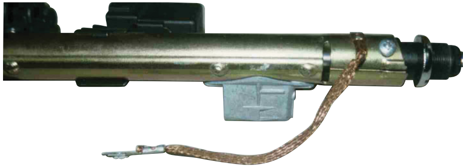
FIGURE 11–23 To help prevent underhood electromagnetic devices from interfering with the antenna input, it is important that all ground wires, including the one from this power antenna, be properly grounded.
