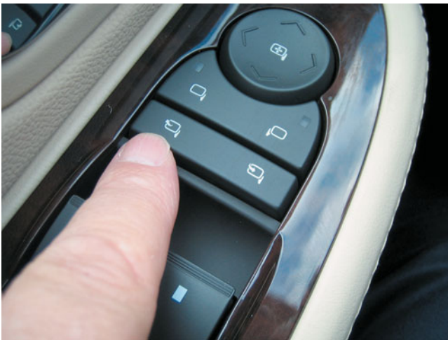
FIGURE 24-24 The electric mirror control is located on the driver's side door panel on this Cadillac Escalade.
