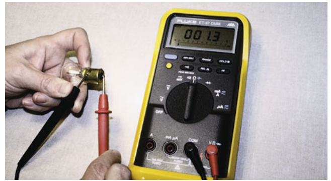
FIGURE 6-10 Using a digital multimeter set to read ohms ( \Omega ) to test this light bulb. The meter reads the resistance of the filament.
