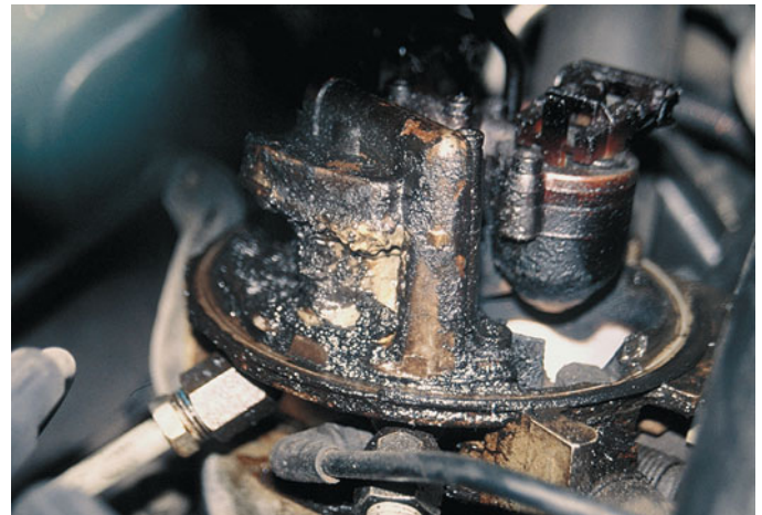
FIGURE 37-3 A clogged PCV system caused the engine oil fumes to be drawn into the air cleaner assembly. This is what the technician discovered during a visual inspection on this TBI system.
