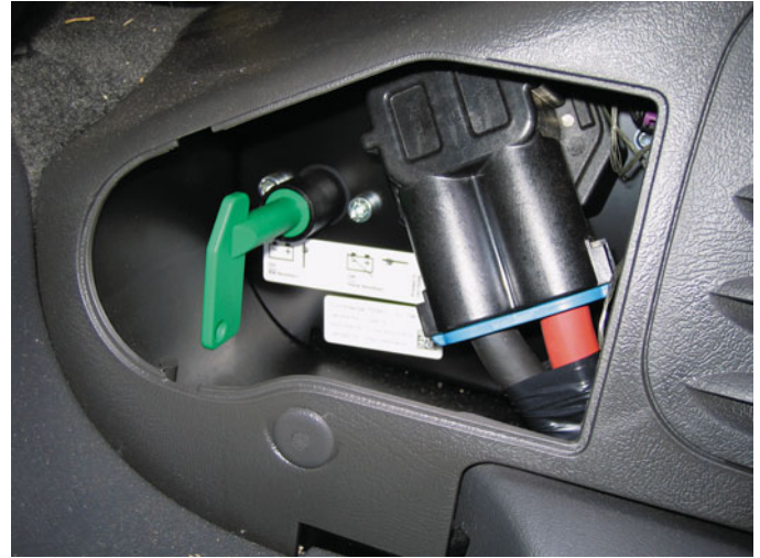
FIGURE 1-87 The shut-off switch on a GM parallel hybrid truck is green because this system uses 42 volts instead of higher, and possible fatal, voltages used in other hybrid vehicles.
