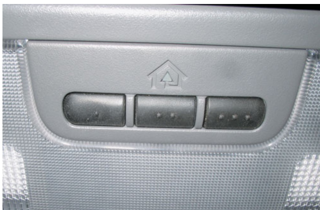
FIGURE 24–12 Typical HomeLink garage door opener buttons. Notice that three different units can be controlled from the vehicle using the HomeLink system.
