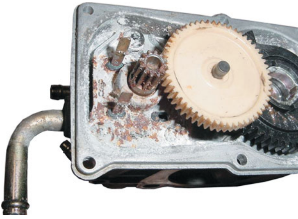
FIGURE 36-12 A corroded electronic throttle control assembly shown with the cover removed.
