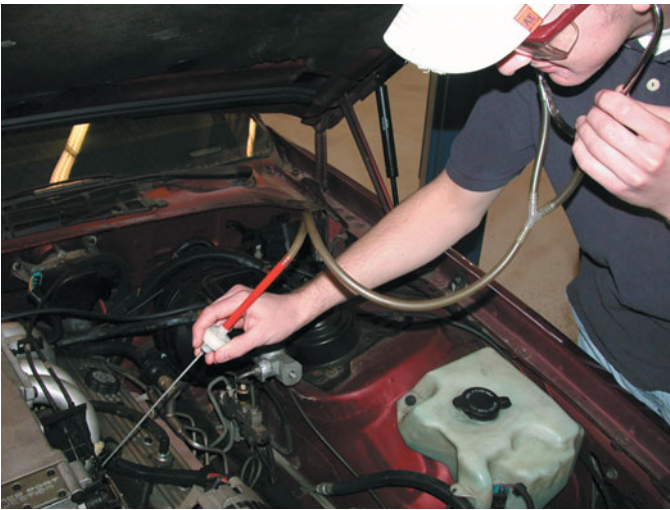
FIGURE 37-4 All fuel injectors should make the same sound with the engine running at idle speed. A lack of sound indicates a possible electrically open injector or a break in the wiring. A defective computer could also be the cause of a lack of clicking (pulsing) of the injectors.
