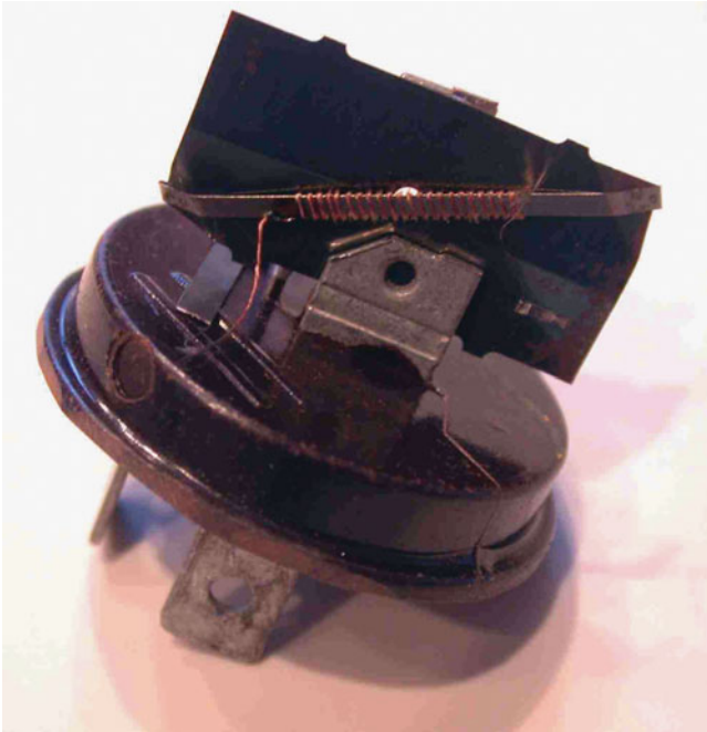
FIGURE 21-13 A hazard warning flasher uses a parallel resistor across the contacts to provide a constant flashing rate regardless of the number of bulbs used in the circuit.
