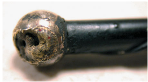
FIGURE 26–26 The tip of this antenna was struck by lightning.
