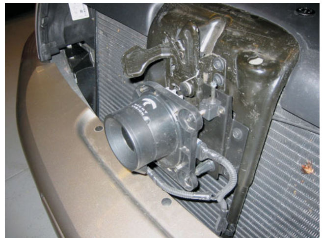
FIGURE 22-34 A night vision camera behind the grille of a Cadillac.
