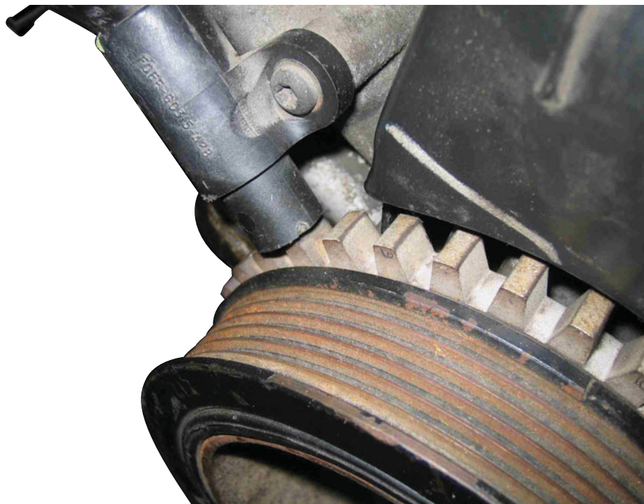
FIGURE 11-6 A crankshaft position sensor and reluctor (notched wheel).
