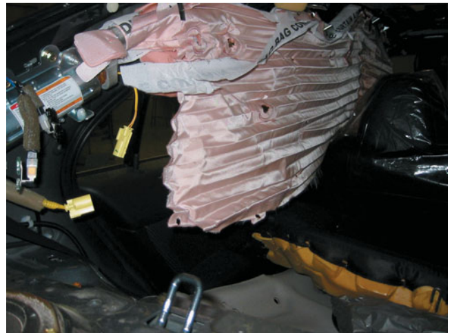
FIGURE 25-8 This shows a deployed side curtain airbag on a training vehicle.
