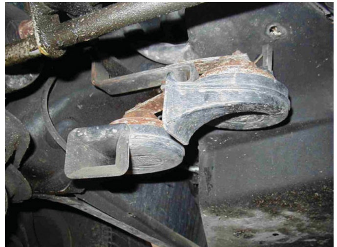
FIGURE 23-1 Two horns are used on this vehicle. Many vehicles use only one horn, often hidden underneath the vehicle.
