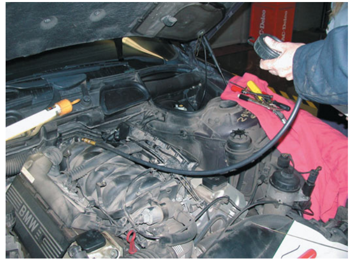
FIGURE 37-7 Checking the fuel pressure using a fuel-pressure gauge connected to the Schrader valve.
