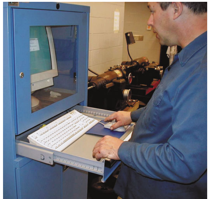
FIGURE 40-8 After checking for stored diagnostic trouble codes (DTCs), the wise technician checks service information for any technical service bulletins that may relate to the vehicle being serviced.
