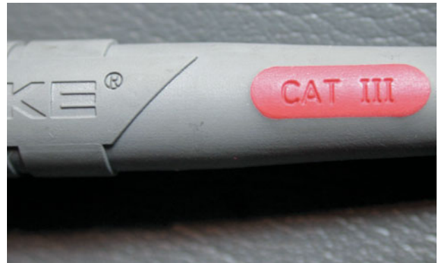
FIGURE 41-5 The meter leads should also be CAT III-rated when checking voltages on a hybrid electric vehicle.
