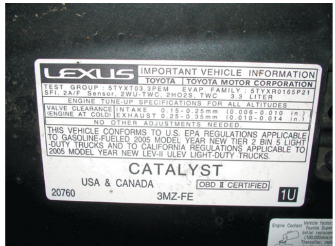
FIGURE 38-1 The underhood decal showing that this Lexus RX-330 meets both national (Tier 2; BIN 5) and California LEV-II (ULEV) regulation standards.
