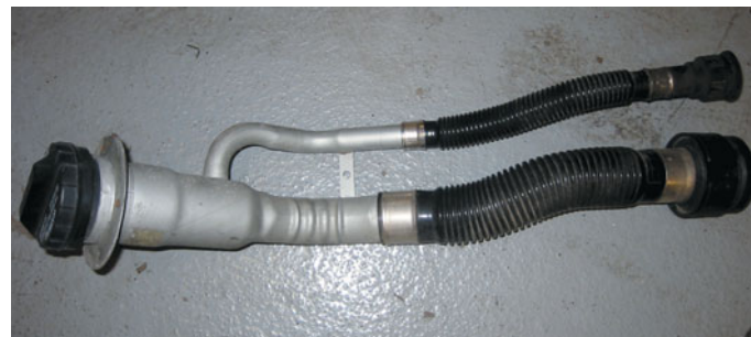
FIGURE 34-4 Vehicles equipped with onboard refueling vapor recovery usually have a reduced-size fill tube.
