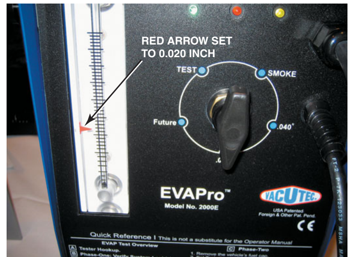
FIGURE 39-36 To test for a leak, this tester was set to the 0.020 in. hole and turned on. The ball rose in the scale on the left and the red arrow was moved to that location. When testing the system for leaks, if the ball rises higher than the arrow, then the leak is larger than 0.02 in. If the ball does not rise to the level of the arrow, the leak is smaller than 0.02 in.
