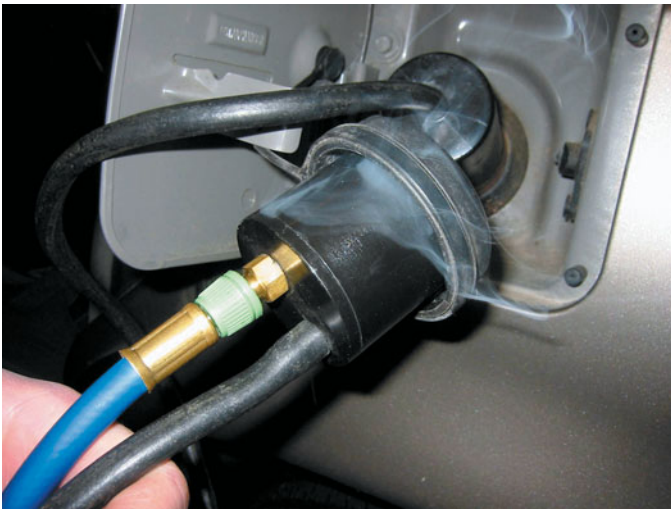
FIGURE 39-37 This unit is applying smoke to the fuel tank through an adapter and the leak was easily found to be the gas cap seal.
