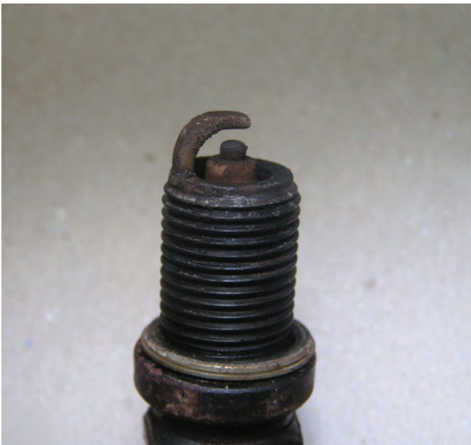
FIGURE 33-39 A worn spark plug showing fuel and/or oil deposits.
