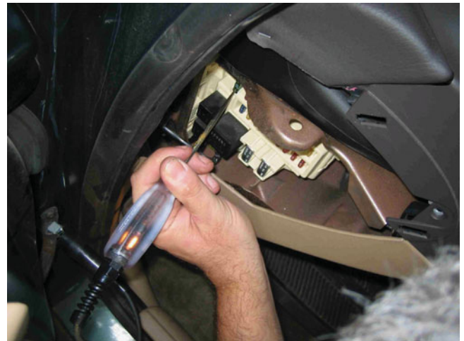
FIGURE 8-7 To test a fuse, use a test light to check for power at the power side of the fuse. The ignition switch and lights may have to be on before some fuses receive power. If the fuse is good, the test light should light on both sides (power side and load side) of the fuse.
