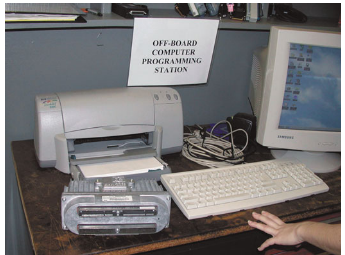
FIGURE 40-20 Connecting cables and a computer to perform off-board programming.
