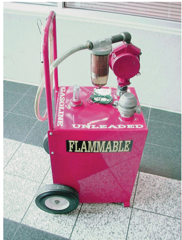
FIGURE 2-8 This red gasoline container holds about 30 gallons of gasoline and is used to fill vehicles used for training.
