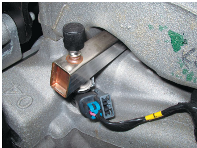
FIGURE 35-15 A rectangular-shaped fuel rail is used to help dampen fuel system pulsations and noise caused by the injectors opening and closing.
