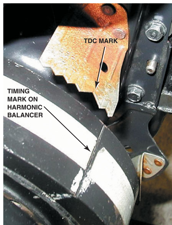
FIGURE 33-42 Ignition timing marks are found on the harmonic balancers on engines equipped with distributors that can be adjusted for timing.
