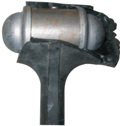
FIGURE 1-35 A dead-blow hammer that was left outside in freezing weather. The plastic covering was damaged, which destroyed this hammer. The lead shot is encased in the metal housing and then covered.
