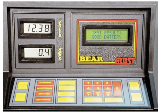
FIGURE 16-7 An alternator regulator battery starter tester (ARBST) automatically loads the battery with a fixed load for 15 sec. to remove the surface charge, then removes the load for 30 sec. to allow the battery to recover, and then reapplies the load for another 15 sec. The results of the test are then displayed.
