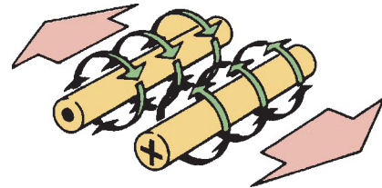
FIGURE 11-10 Conductors with opposing magnetic fields will move apart into weaker fields.
