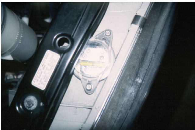
FIGURE 21-23 Many composite headlights have a built-in bubble level to make aiming easy and accurate.
