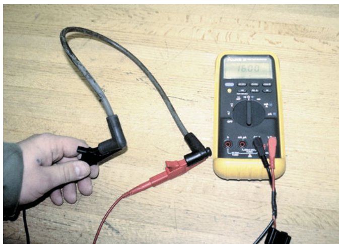
FIGURE 33-31 Measuring the resistance of a spark plug wire with a multimeter set to the ohms position. The reading of 16.03 k \Omega (16,030 ohms) is okay because the wire is about 2 ft long. Maximum allowable resistance for a spark plug wire this long would be 20 k \Omega (20,000 ohms).
