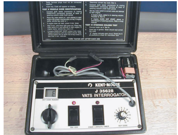
FIGURE 24-30 A special tool is needed to diagnose a General Motors VATS security system and special keys that contain a resistor pellet.
