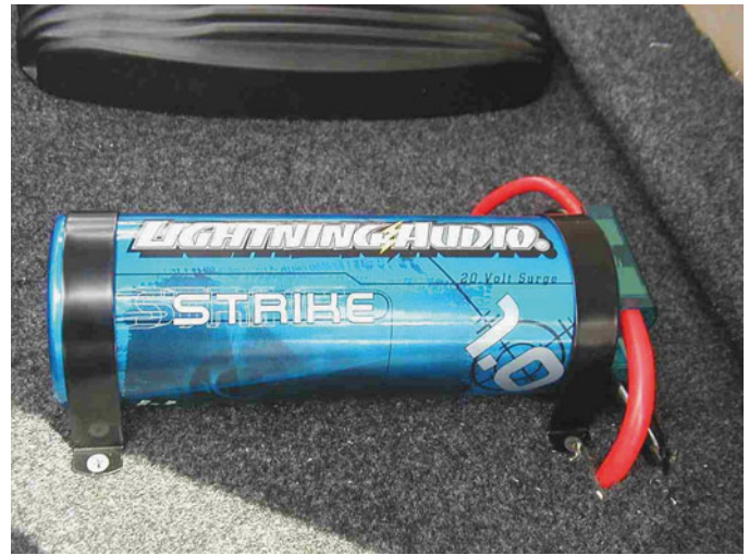
FIGURE 10-9 A 1 farad capacitor used to boost the power to large speakers.
