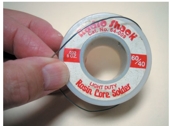
FIGURE 8-18 Always use rosin-core solder for electrical or electronic soldering. Also, use small-diameter solder for small soldering irons. Use large-diameter solder only for large-diameter (large-gauge) wire and higher-wattage soldering irons (guns).
