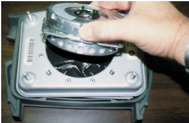
FIGURE 25-7 The inflator module is being removed from the airbag housing. The squib, inside the inflator module, is the heating element that ignites the pyrotechnic gas generator that rapidly produces nitrogen gas to fill the airbag.
