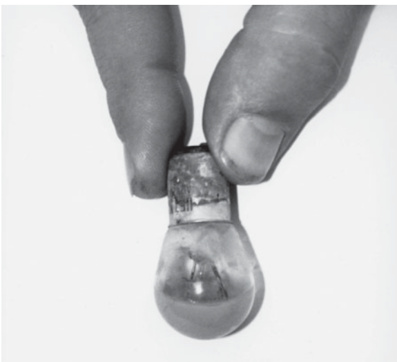
FIGURE 21-5 Often the best diagnosis is a thorough visual inspection. This bulb was found to be filled with water, which caused weird problems.
