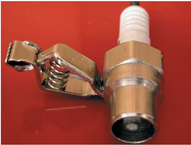
FIGURE 33-22 A spark tester looks like a regular spark plug with an alligator clip attached to the shell. This tester has a specified gap that requires at least 25,000 volts (25 kV) to fire.
