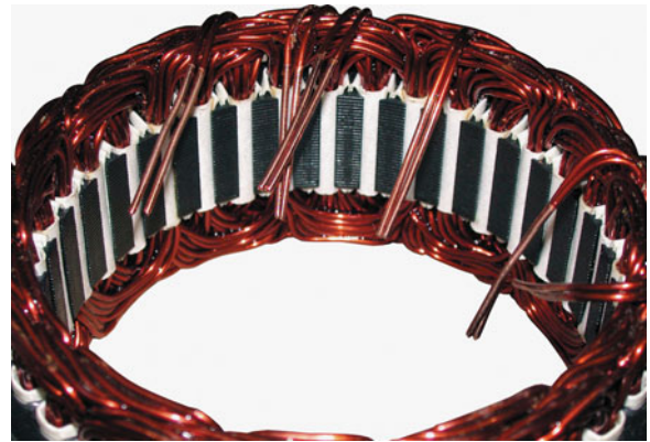
FIGURE 19-16 A stator assembly with six, rather than the normal three, windings.
