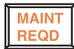
FIGURE 22-4 Maintenance required. This usually means that the engine oil is scheduled to be changed or other routine service items replaced or checked.
