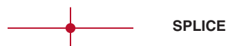
FIGURE 9-9 Two wires that cross at the dot indicate that the two are electrically connected.
