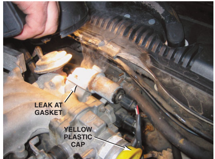
FIGURE 40-5 Using a bright light makes seeing where the smoke is coming from easier. In this case, smoke was added to the intake manifold with the inlet blocked with a yellow plastic cap and smoke was seen escaping past a gasket at the idle air control.
