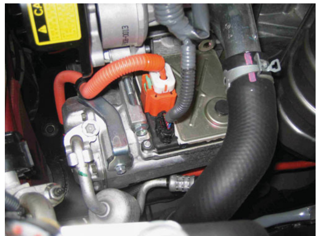
FIGURE 8-27 Always follow the vehicle manufacturer's instructions which include the use of linesman's (high-voltage) gloves if working on circuits that are covered in orange conduit.
