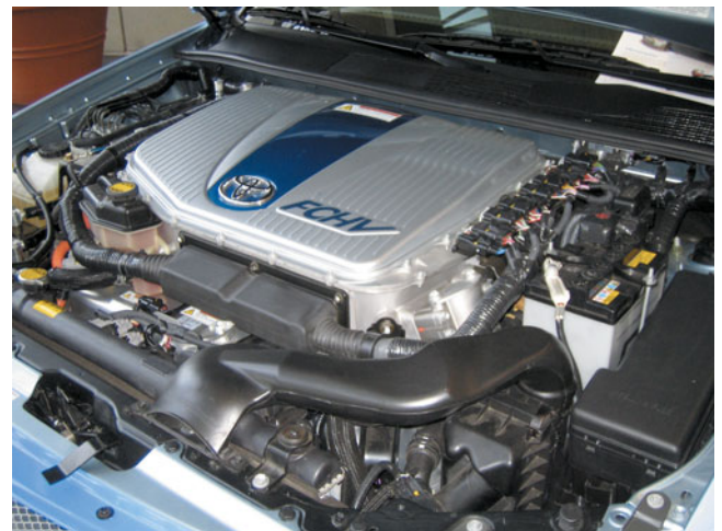
FIGURE 42-11 Space is limited at the front of the Toyota FCHV engine compartment, so an auxiliary heat exchanger is located under the vehicle to help cool the fuel-cell stack.
