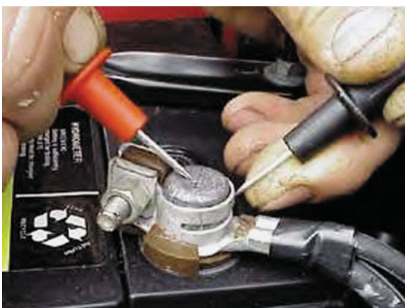
FIGURE 18-4 To test the voltage drop of the battery cable connection, place one voltmeter lead on the battery terminal and the other voltmeter lead on the cable end and crank the engine. The voltmeter will read the difference in voltage between the two leads, which should not exceed 0.20 volt (200 mV).
