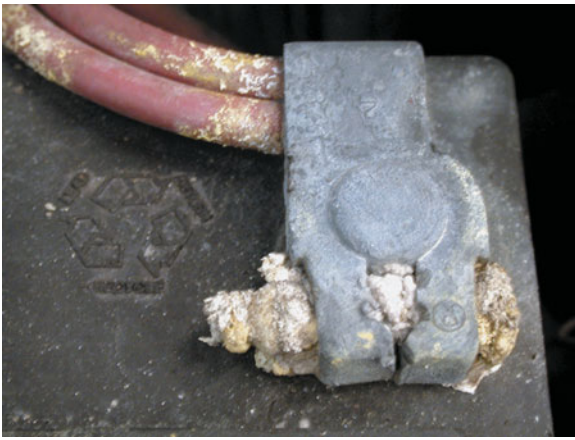
FIGURE 16-2 Corrosion on a battery cable could be an indication that the battery itself is either being overcharged or is sulfated, creating a lot of gassing of the electrolyte.
