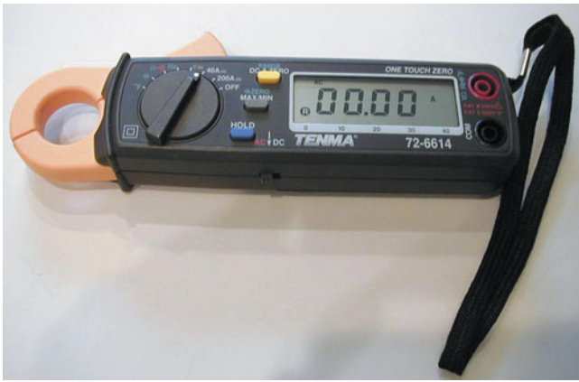
FIGURE 6-15 A typical mini clamp-on-type digital multimeter. This meter is capable of measuring alternating current (AC) and direct current (DC) without requiring that the circuit be disconnected to install the meter in series. The jaws are simply placed over the wire and current flow through the circuit is displayed.
