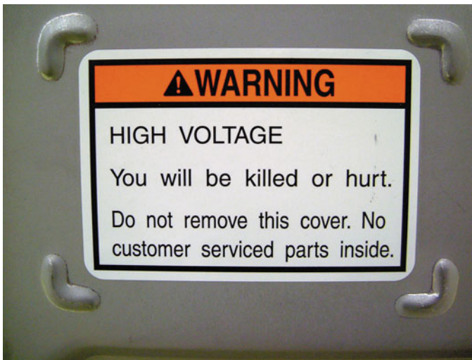
FIGURE 1-84 A warning label on a Honda hybrid warns that a person can be killed due to the high-voltage circuits under the cover.
