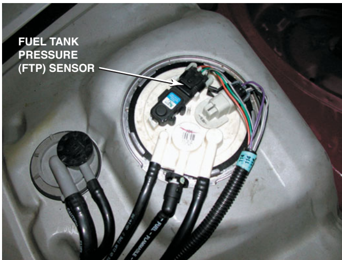
FIGURE 39-39 The fuel tank pressure sensor looks like a MAP sensor and is usually located on top of the fuel pump module (white unit).
