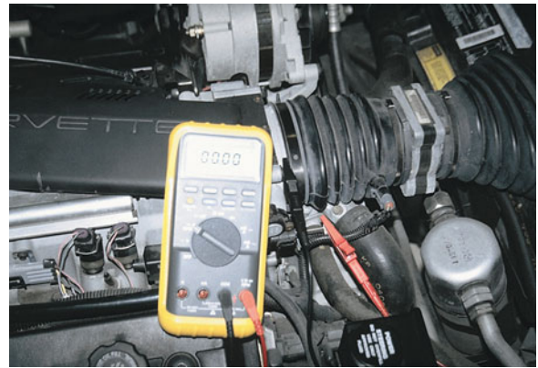
FIGURE 29-6 Checking the voltage drop between the TP sensor ground and a good engine ground with the ignition on (engine off). A reading of greater than 0.2 volt (200 mV) represents a bad computer ground.
