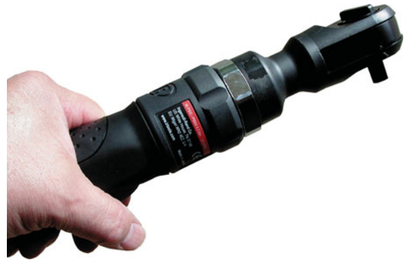
FIGURE 1-58 An air ratchet is a very useful tool that allows fast removal and installation of fasteners, especially in areas that are difficult to reach or do not have room enough to move a hand ratchet or wrench.
