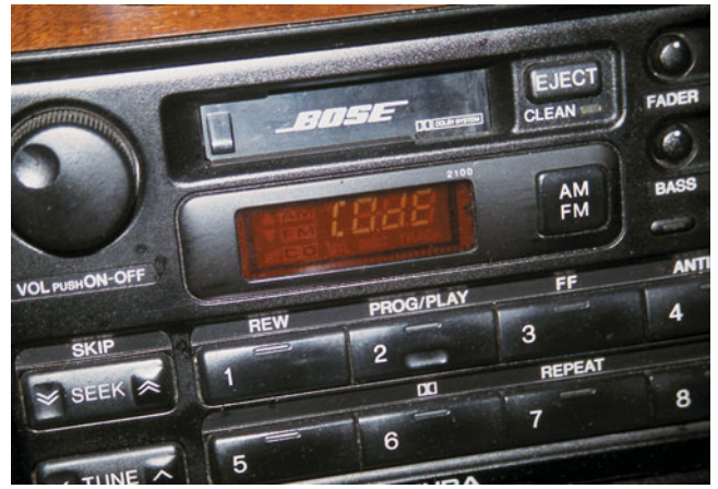
FIGURE 16-18 The battery was replaced in this Acura and the radio displayed “code” when the replacement battery was installed. Thankfully, the owner had the five-digit code required to unlock the radio.
