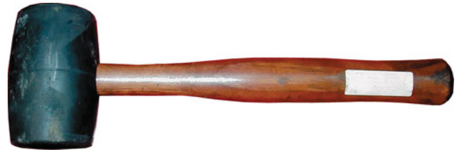
FIGURE 1-34 A rubber mallet used to deliver a force to an object without harming the surface.
