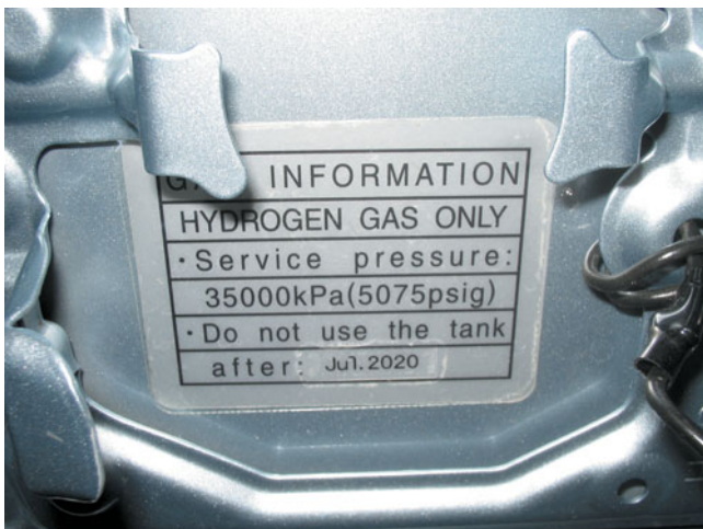
FIGURE 42-23 Note that high-pressure hydrogen storage tanks must be replaced in 2020.
