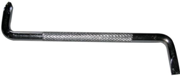
FIGURE 1-31 An offset screwdriver is used to install or remove fasteners that do not have enough space above to use a conventional screwdriver.
