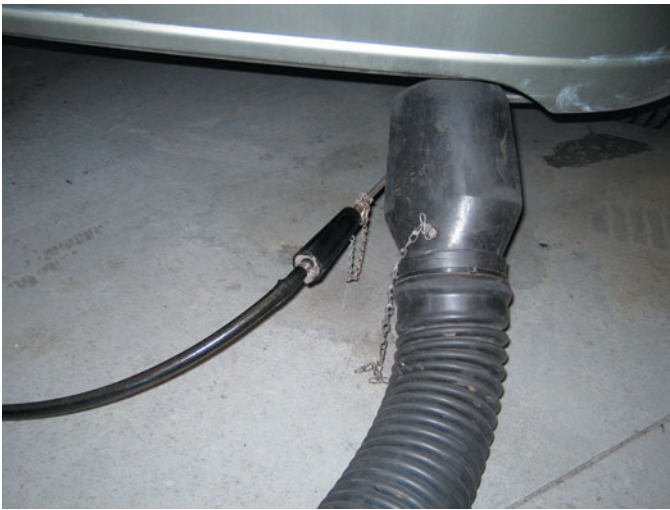
FIGURE 38–6 A partial stream sampling exhaust probe being used to measure exhaust gases in parts per million (PPM) or percent (%).
