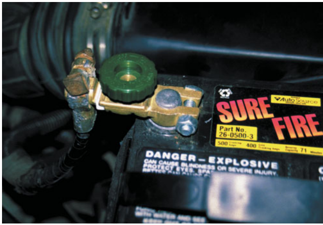
FIGURE 16-17 After connecting the shut-off tool, start the engine and operate all accessories. Stop the engine and turn off everything. Connect the ammeter across the shut-off switch in parallel. Wait 20 minutes. This time allows all electronic circuits to “time out” or shut down. Open the switch—all current now will flow through the ammeter. A reading greater than specified (usually greater than 50 mA, or 0.05 A) indicates a problem that should be corrected.
