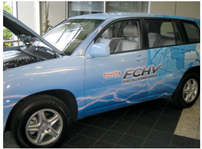
FIGURE 42-4 The Toyota FCHV is based on the Highlander platform and uses much of Toyota's Hybrid Synergy Drive (HSD) technology in its design.
