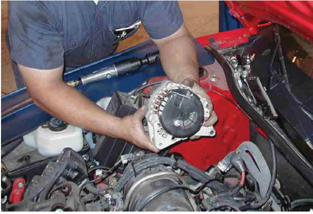
FIGURE 20-13 Replacing an alternator is not always as easy as it is from a Buick with a 3800 V-6, where the alternator is easy to access. Many alternators are difficult to access, and require the removal of other components.
