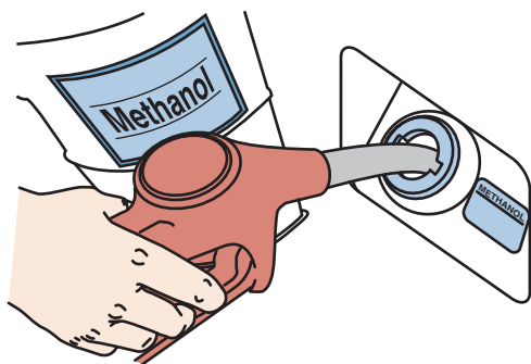
FIGURE 42-8 A direct methanol fuel cell can be refueled similar to a gasoline-powered vehicle.
