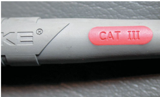
FIGURE 6-21 Always use meter leads that are CAT III rated on a meter that is also CAT III rated, to maintain the protection needed when working on hybrid vehicles.
