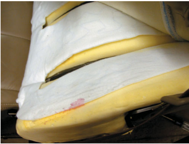
FIGURE 24-19 The heating element of a heated seat is a replaceable part, but service requires that the upholstery be removed. The yellow part is the seat foam material and the entire white cover is the replaceable heating element. This is then covered by the seat material.
