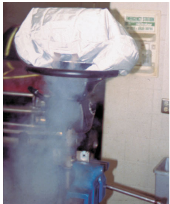
FIGURE 25-18 An airbag being deployed as part of a demonstration in an automotive laboratory.
