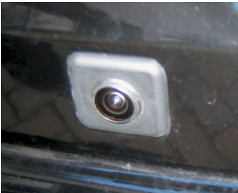
FIGURE 22-49 A typical fisheye-type backup camera usually located near the center on the rear of the vehicle near the license plate.
