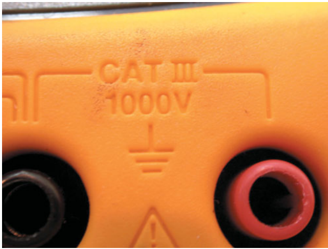
FIGURE 6-20 Be sure to only use a meter that is CAT III rated when taking electrical voltage measurements on a hybrid vehicle.
