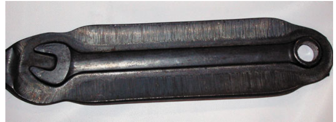
FIGURE 1-15 A forged wrench after it has been forged but before the flashing (extra material around the wrench) has been removed.
