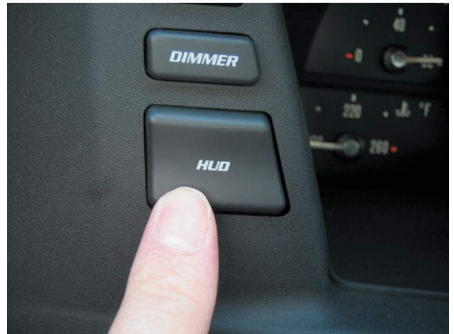
FIGURE 22-32 The dash-mounted control for the head-up display on this Cadillac allows the driver to move the image up and down on the windshield for best viewing.
