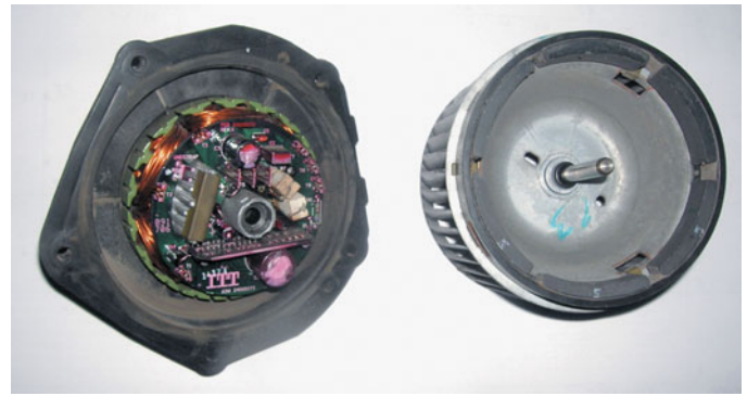
FIGURE 23-21 A brushless DC motor that uses the body computer to control the speed. (Courtesy of Sammy's Auto Service, Inc.)
