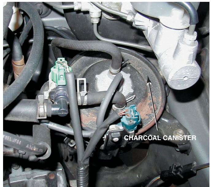
FIGURE 39-30 A charcoal canister can be located under the hood or underneath the vehicle.
