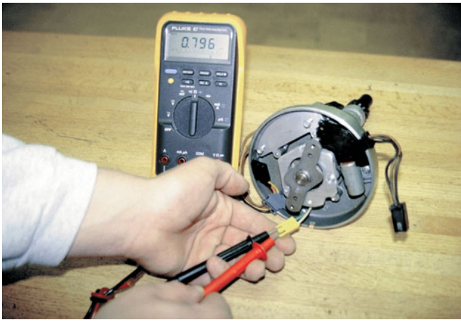
FIGURE 33–25 Measuring the resistance of an HEI pickup coil using a digital multimeter set to the ohms position. The reading on the face of the meter is 0.796 kΩ or 796 ohms in the middle of the 500 to 1,500 ohm specifications.
