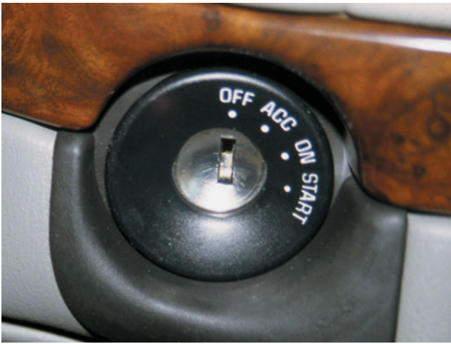
FIGURE 22-39 Many newer vehicles place the ignition switch on the dash and incorporate antitheft controls. Note the location of the accessory position.
