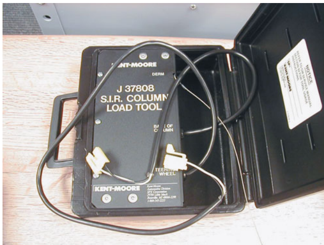
FIGURE 25–14 An airbag diagnostic tester. Included in the plastic box are electrical connectors and a load tool that substitutes for the inflator module during troubleshooting.
