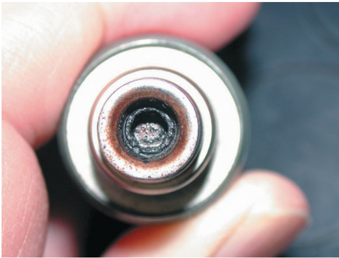
FIGURE 37-14 If an injector has the specified resistance, this does not mean that it is okay. This injector had the specified resistance yet it did not deliver the correct amount of fuel because it was clogged.
