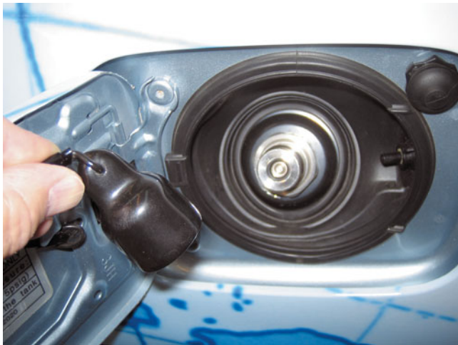
FIGURE 42-22 The high-pressure fitting used to refuel a fuel-cell hybrid vehicle.
