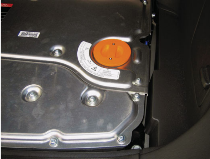
FIGURE 1-86 The high-voltage shut-off switch on a Ford Escape hybrid. The switch is located under the carpet at the rear of the vehicle.
