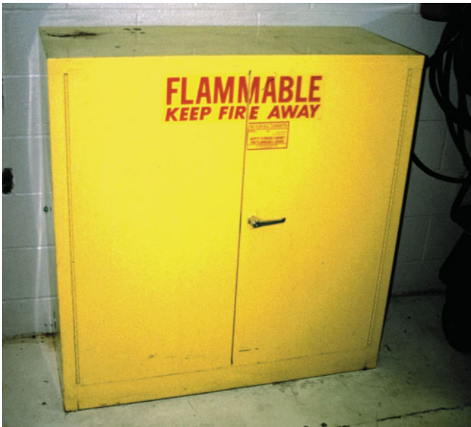
FIGURE 2-5 Typical fireproof flammable storage cabinet.
