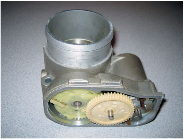
FIGURE 24-4 A typical electronic throttle with the protective covers removed.
