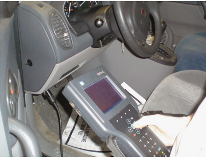
FIGURE 40-17 The first step in the reprogramming procedure is to determine the current software installed using a scan tool. Not all scan tools can be used. In most cases using the factory scan tool is needed for reprogramming unless the scan tool is equipped to handle reprogramming.
