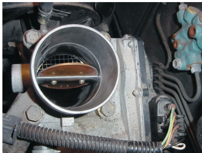
FIGURE 36-11 The throttle plate stayed where it was moved, which indicates that there is a problem with the electronic throttle body control assembly.
