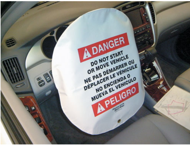
FIGURE 41-9 Using a warning cover over the steering wheel helps others realize that work is being performed on the high-voltage system and that no one is to attempt to start or move the vehicle.
