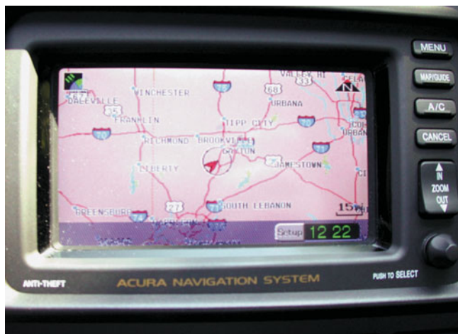
FIGURE 22-36 A typical navigation system. This Honda/Acura system uses some of the climate control functions as well as the trip information on the display. This particular unit uses a DVD unit in the trunk along with a global positioning satellite (GPS) to display a map and your exact location for the entire country.
