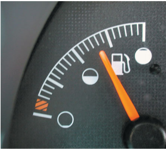
FIGURE 39-41 The fuel level must be between 15% and 85% before the EVAP monitor will run on most vehicles.
