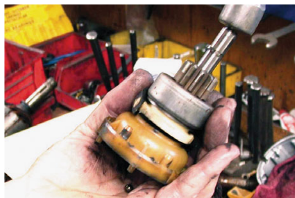
10 A light tap with a hammer dislodges the armature thrust ball (in the palm of the hand) from the center of the gear reduction assembly.
