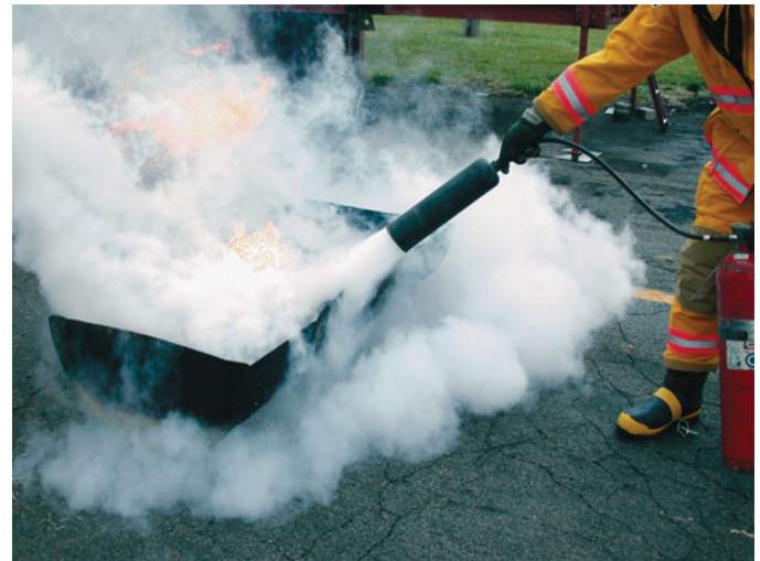
FIGURE 1-80 A CO 2 fire extinguisher being used on a fire set in an open drum during a demonstration at a fire training center.
