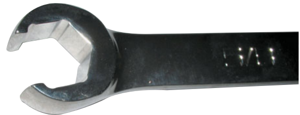
FIGURE 1-20 The end of a typical line wrench, which shows that it is capable of grasping most of the head of the fitting.
