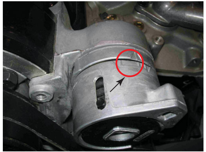
FIGURE 20-5 Check service information for the exact marks where the tensioner should be located for proper belt tension.
