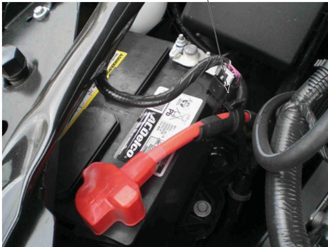
FIGURE 19-21 A Hall-effect current sensor attached to the positive battery cable is used as part of the EPM system.
