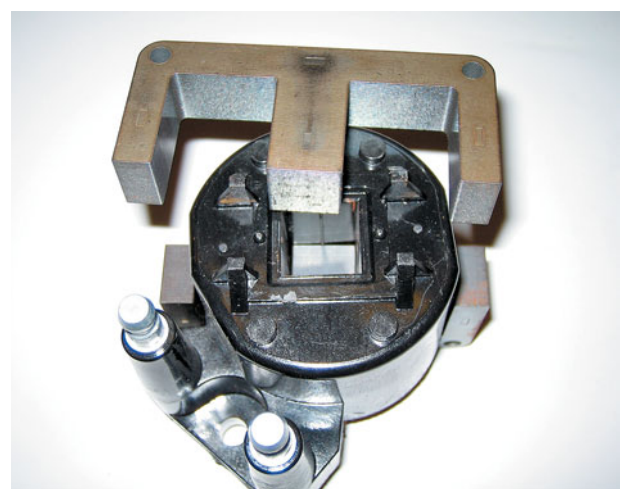
FIGURE 33-3 The steel lamination used in an E coil helps increase the magnetic field strength, which helps the coil produce higher energy output for a more complete combustion in the cylinders.
