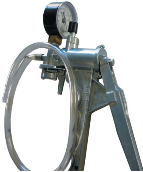
FIGURE 30-7 A typical hand-operated vacuum pump.
