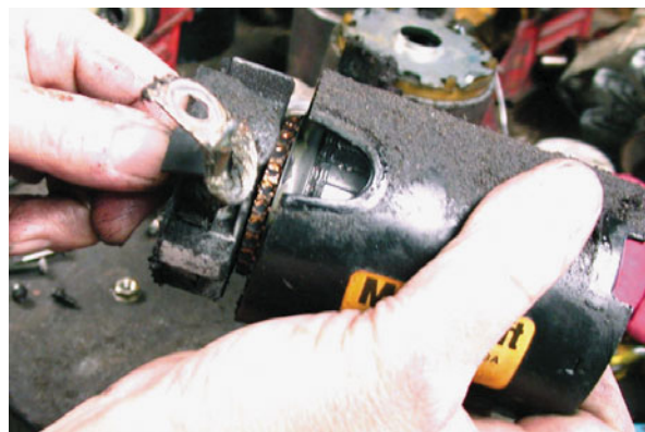
8 The armature assembly is removed from the field frame.
