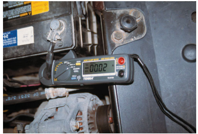
FIGURE 16-16 This mini clamp-on digital multimeter is being used to measure the amount of battery electrical drain that is present. In this case, a reading of 20 mA (displayed on the meter as 00.02 A) is within the normal range of 20 to 30 mA. Be sure to clamp around all of the positive battery cable or all of the negative battery cable, whichever is easiest to get the clamp around.
