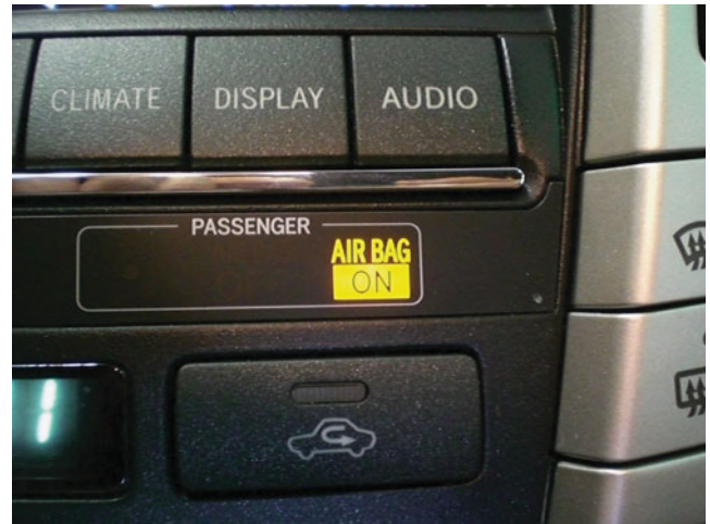
FIGURE 25-20 The passenger side airbag “on” lamp will light if a passenger is detected on the passenger seat.
