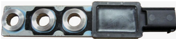
FIGURE 25-22 A resistor-type occupant detection sensor. The weight of the passenger strains these resistors, which are attached to the seat, thereby signaling to the module the weight of the occupant.
