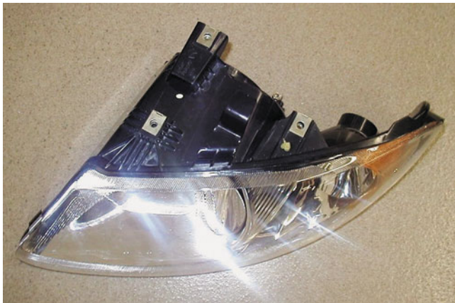
FIGURE 21-17 A typical composite headlamp assembly. The lens, housing, and bulb sockets are usually included as a complete assembly.
