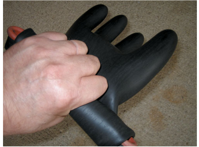
FIGURE 41-3 Checking rubber lineman's gloves for pinhole leaks.
