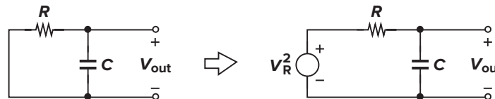
Figure 7.15 Noise generated in a low-pass filter.
