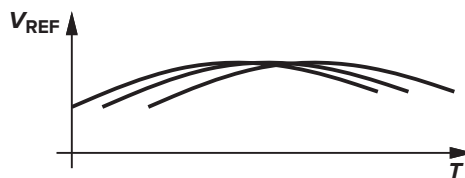
Figure 12.17 Variation of the zero-TC temperature for different samples.
