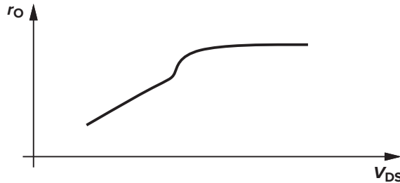
Figure 17.15 Kink in output resistance in Level 3 model.
