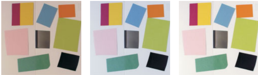
Figure 6.43 Simple colour correction. Left: original image captured under incandescent lights, resulting in a yellowish red cast; centre: correcting assuming the average is grey, using Equation 6.86; right: correcting assuming the brightest pixel is white, using Equation 6.88.
