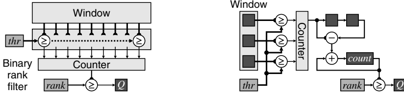
Figure 8.36 Binary rank filter for threshold decomposition. Left: thresholding to create binary values, and counting; right: an efficient implementation exploiting commonality between adjacent window positions.
