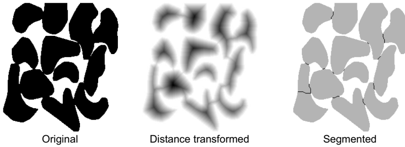
Figure 11.27 Watershed segmentation for separating touching objects. Left: original image; centre: applying the 3,4 chamfer distance transform; right: original with watershed boundaries overlaid.
