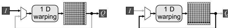
Figure 9.6 Two pass forward mapping. Left: in the first pass each row is warped and written to a frame buffer, while the previous image is streamed out; right: in the second pass, each column is processed and written back to the frame buffer.
