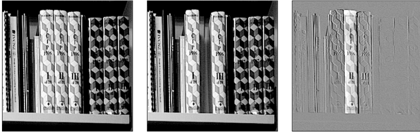
Figure 6.20 Image subtraction to detect change. Left: original scene; centre: the changed scene; right: the difference image (offset to represent zero difference as a mid grey).
