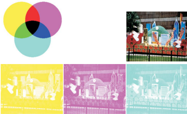
Figure 6.32 CMY colour space. Top left: combining yellow, magenta and cyan secondary colours; bottom: the yellow, magenta and cyan components of the colour image on the top right.
