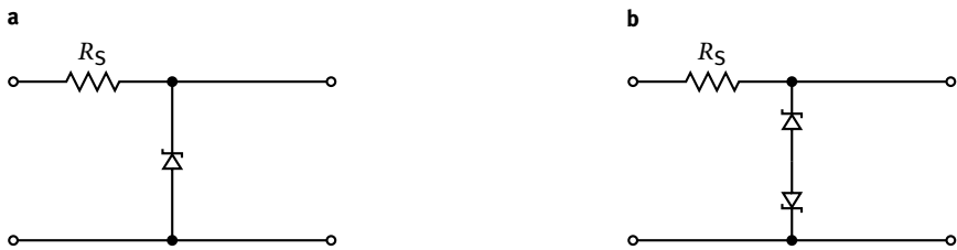
Fig. 2.38. Voltage limiter circuits. (a) Using one Zener diode and (b) having two oppositely biased Zener diodes in series.
