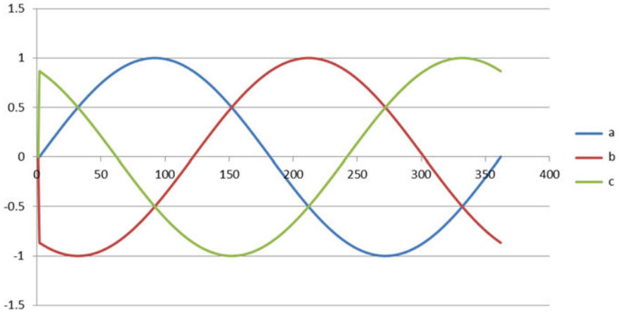
Fig. 1.2 Phase voltages for three-phase bridge rectifier
