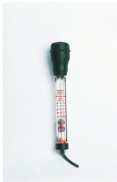
Figure 10-8 Hydrometer to check specific gravity of lead-acid battery.
