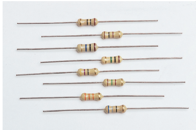
Figure 3-2 Carbon resistors with same physical size but different resistance values. The physical size indicates a power rating of \frac{1}{2} W.
