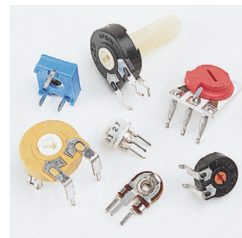
Figure 3-19 Small potentiometers and trimmers often used for variable controls in electronic circuits. Terminal leads are formed for insertion into a PC board.
