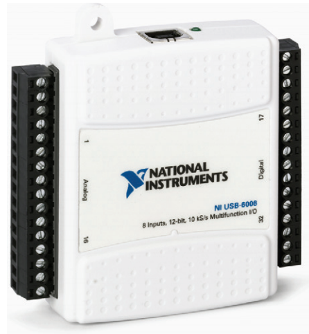
Figure S12-2 The NI USB 6008 DAQ. Its dimensions are 8.5 by 8.2 by 2.3 cm. The screw terminals on both sides are used for connecting the external sensor cables from transducers or signal-conditioning equipment. The USB connector is on the top.
