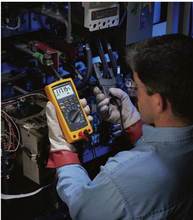
Figure 12-14 DMM with amp-clamp accessory.
