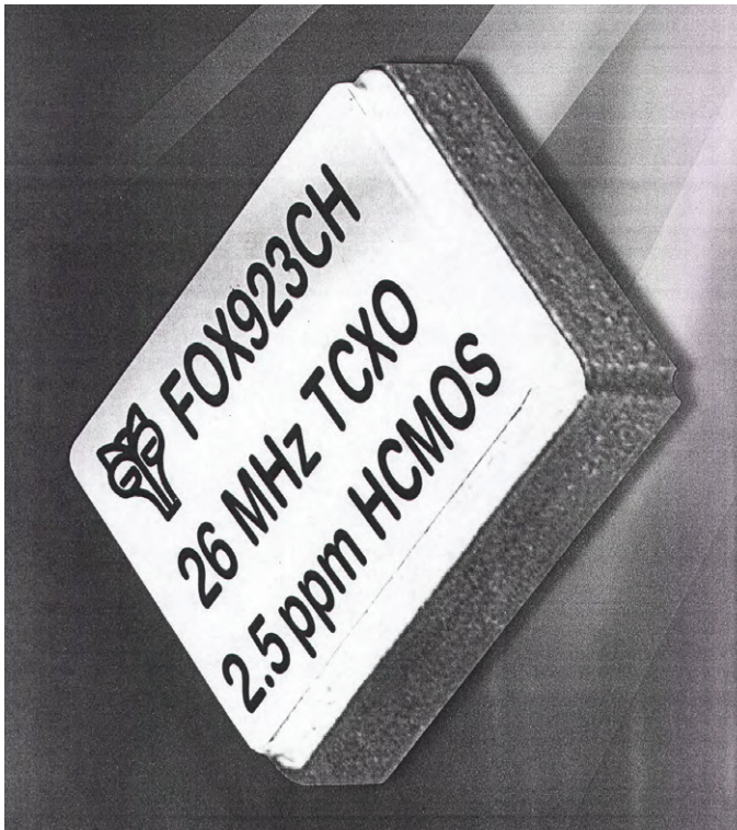
Figure 38-14 A TCXO in a 3.2- by 2.5-mm package.
