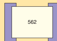
Figure 3-14 Chip resistor with number coding.
