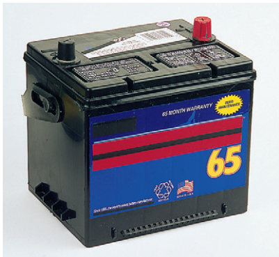
Figure 10-2 Example of a 12-V auto battery using six lead-acid cells in series. This is a secondary type, which can be recharged.
