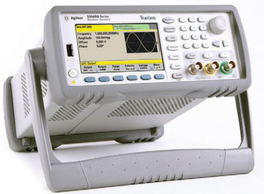
Figure 26-21 A modern arbitrary waveform generator. (Courtesy Agilent Technologies.)
