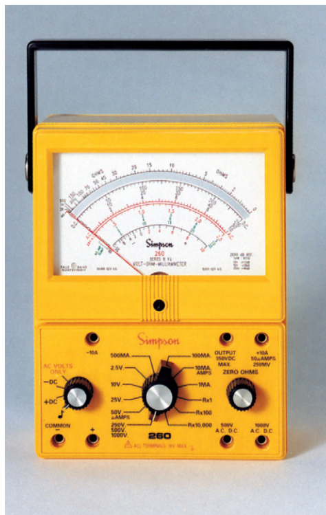
Figure 12-12 Analog VOM that combines a function selector and range switch.
