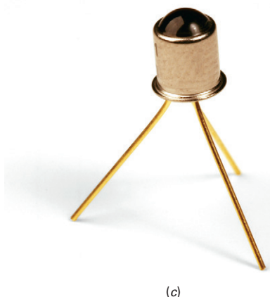
Figure 33-47 Phototransistor. (a) Open base gives maximum sensitivity. (b) Variable base resistor changes sensitivity. (c) Typical phototransistor.
