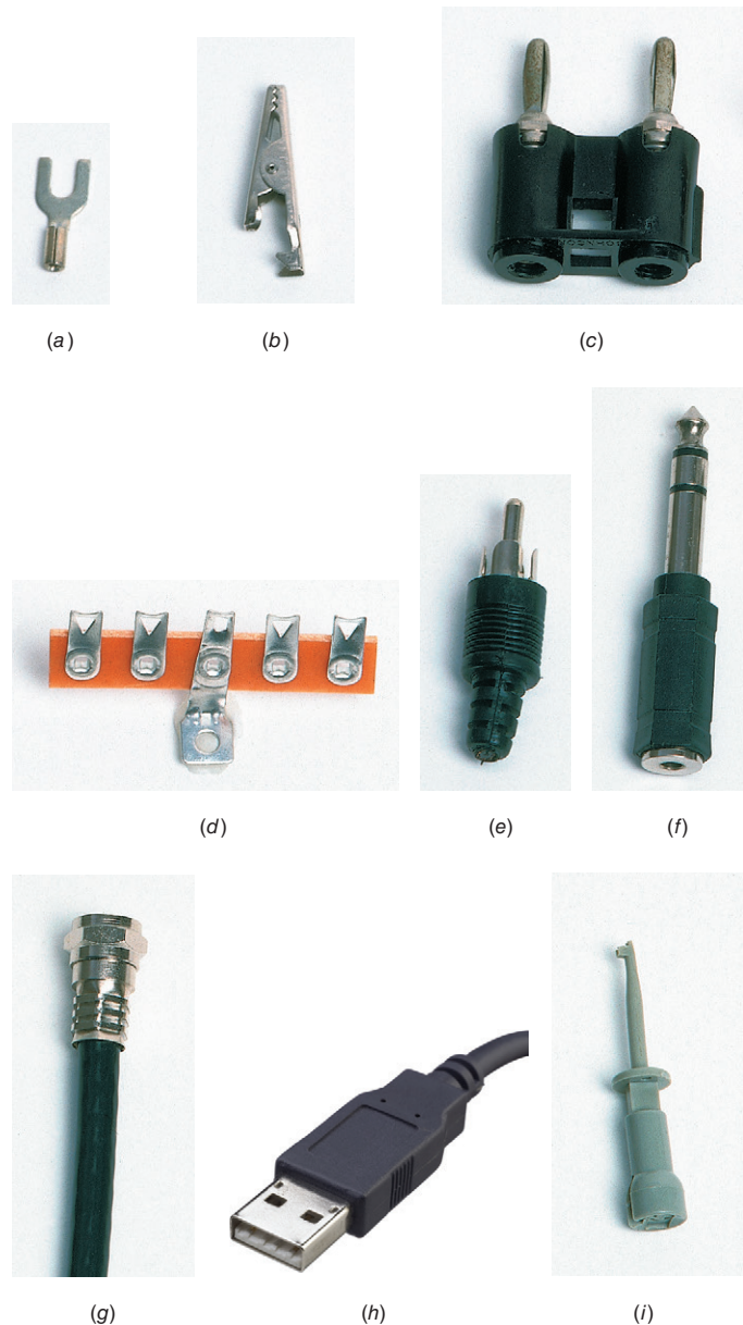
Figure 9-5 Common types of connectors for wire conductors. (a) Spade lug. (b) Alligator clip. (c) Double banana-pin plug. (d) Terminal strip. (e) RCA-type plug for audio cables. (f) Phone plug. (g) F-type plug for cable TV. (h) Multiple-pin connector plug. (i) Spring-loaded metal hook as grabber for temporary connection in testing circuits.
