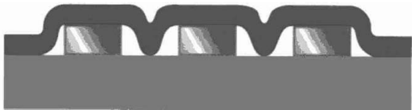
Figure 7.7 Illustration of soda straws of solder resist over three adjacent conductor traces [72]. With permission from the Institute for Interconnecting and Packaging Electronic Circuits.
