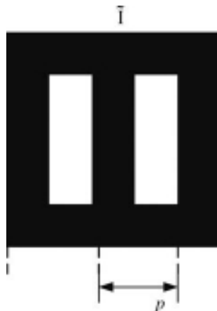
Figure 10.7 Desired pattern of the aerial image searched on the wafer.
