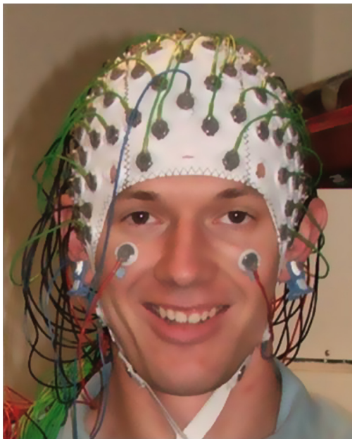
Figure 11.8 Subject with high-density EEG electrode array cap. Image © Flinders University.
