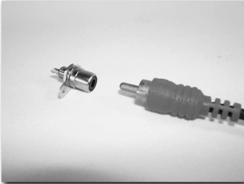
FIGURE 6-25: RCA jack and plug
