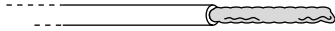
FIGURE 8-11: Tinned, stranded wire should be firm with even solder coating and penetration
