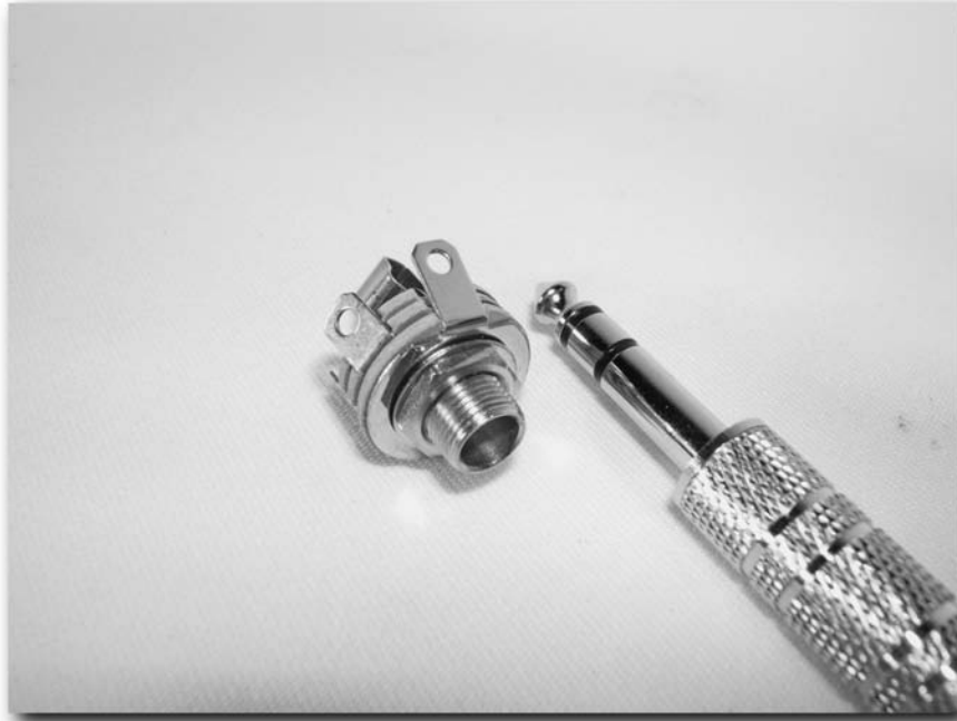
FIGURE 6-24: One-quarter-inch guitar jack and plug
