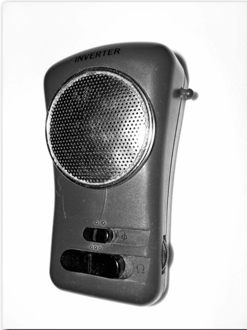
FIGURE 25-1: The Inverter (with internal mercury switch)
