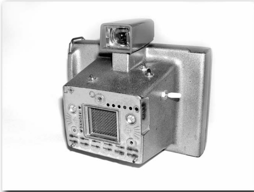
FIGURE 30-3: Ultra-simple Sample Stacker—the same circuit housed inside an emptied Polaroid camera body
