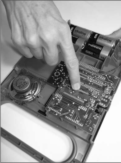
FIGURE 9-11: Touching the circuit while listening for changes in sound
