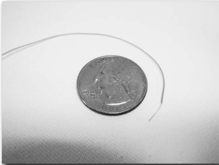
FIGURE 6-21: Wire-wrap wire is thin!
