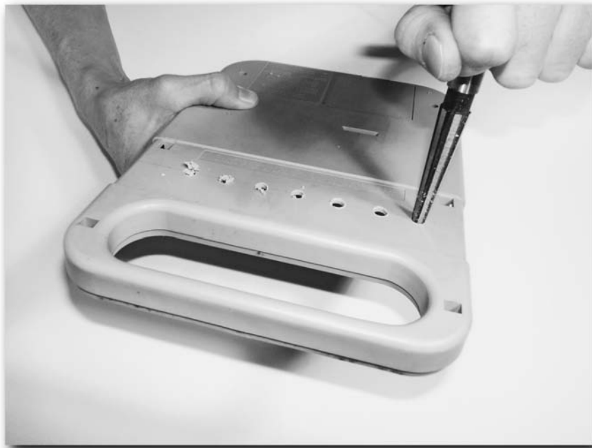
FIGURE 10-8: Using a hand bore to increase pilot hole size
