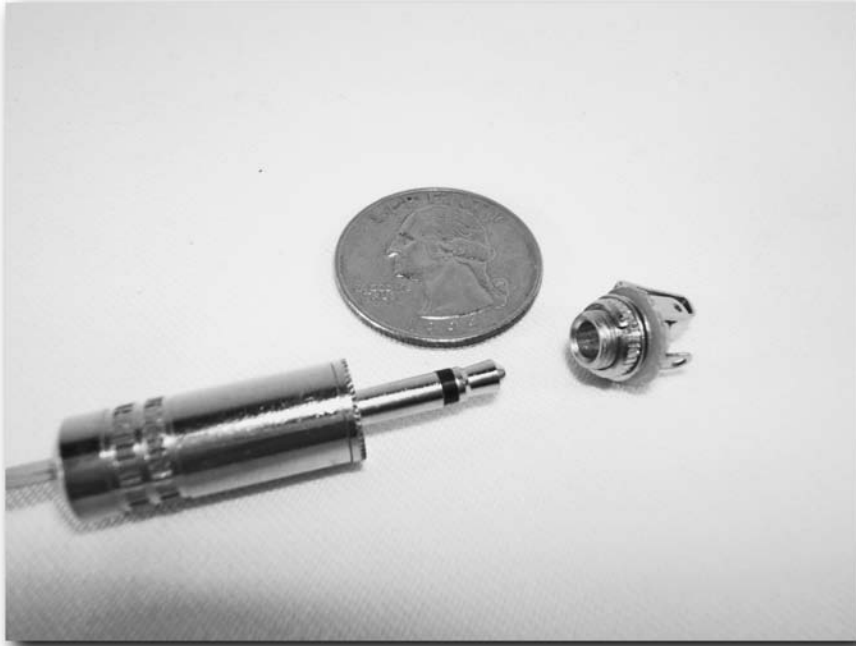
FIGURE 6-26: One-eighth-inch mini-jack and plug
