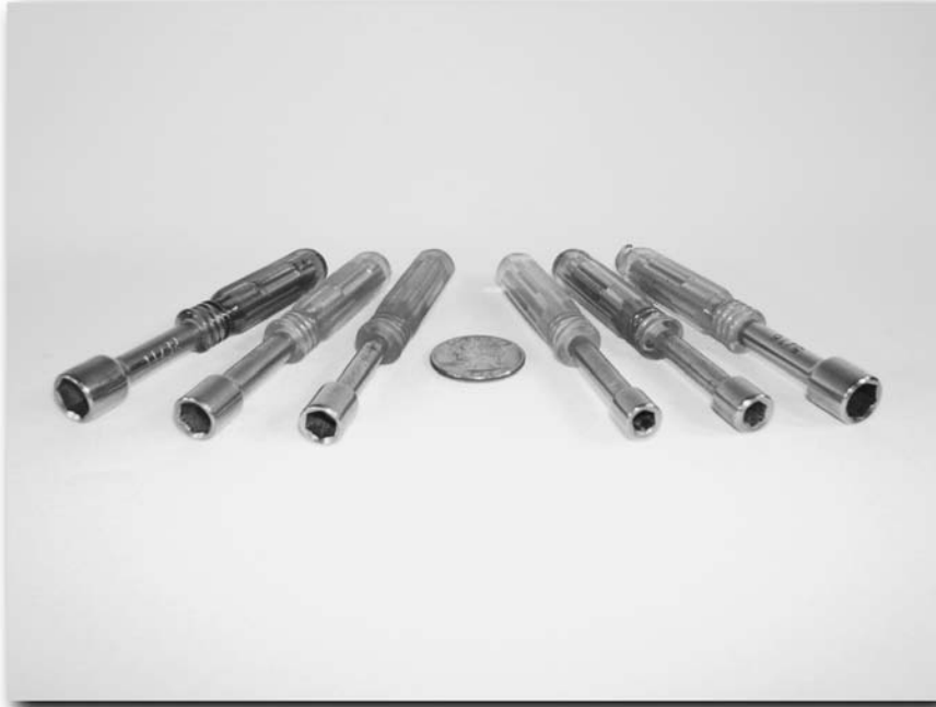
FIGURE 5-7: Socket drivers with hollow shafts
