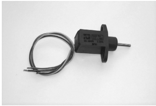
FIGURE 21.5: Resistive linear position sensor
