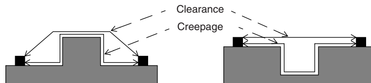
FIGURE 39.2: Creepage and clearance distance
