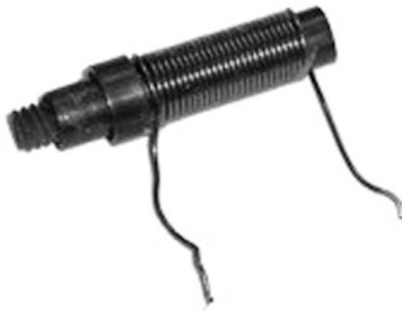
FIGURE 1.63: An adjustable ferrite cored inductor
