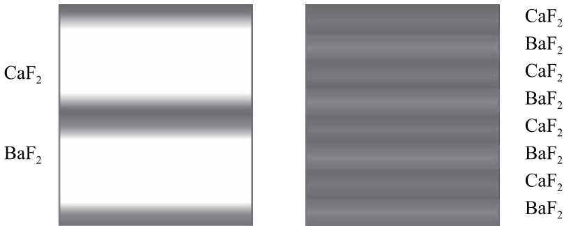
Figure 10.8 (See also colour plates.) Schematic illustration of space charge regions with enhanced ionic conductivity in \text{BaF}_2/\text{CaF}_2 heterostructures.
