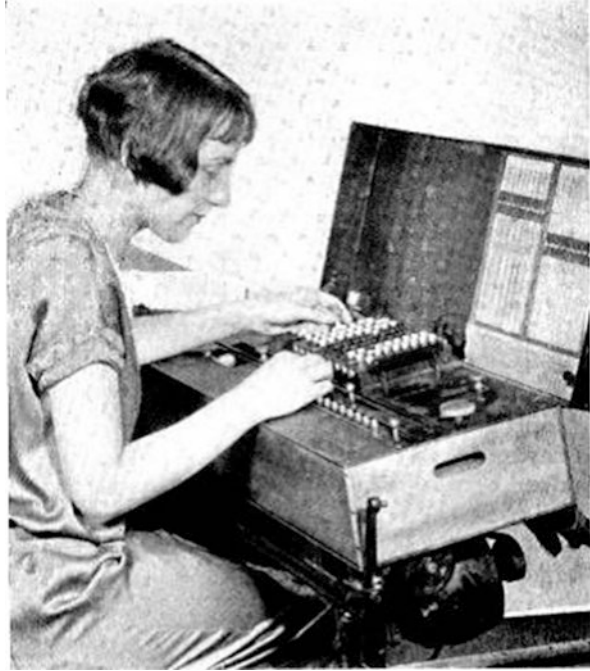
Fig. 4.12 Photograph of Rose Araneo, a Bell Labs computer at the department headed by Thorton Fry, working with a Millionaire calculating machine (1925)
