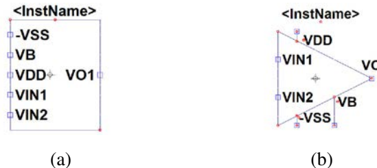
Figure 5.4: LTspice autogenerated symbol (a) and edited symbol (b) for the differential-input pair.
