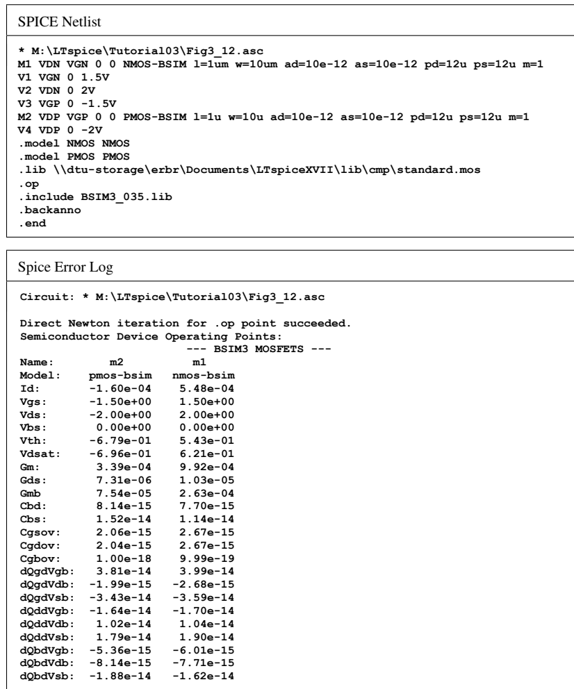
Figure 3.12: Netlist file and error log file for the circuit from Fig. 3.8 simulated with the device models included in BSIM3_035.lib.
