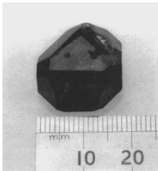
Figure 14.10 The world's largest synthetic diamond crystal grown by the temperature-gradient method (ELEMENTSIX, formerly DeBeers)
