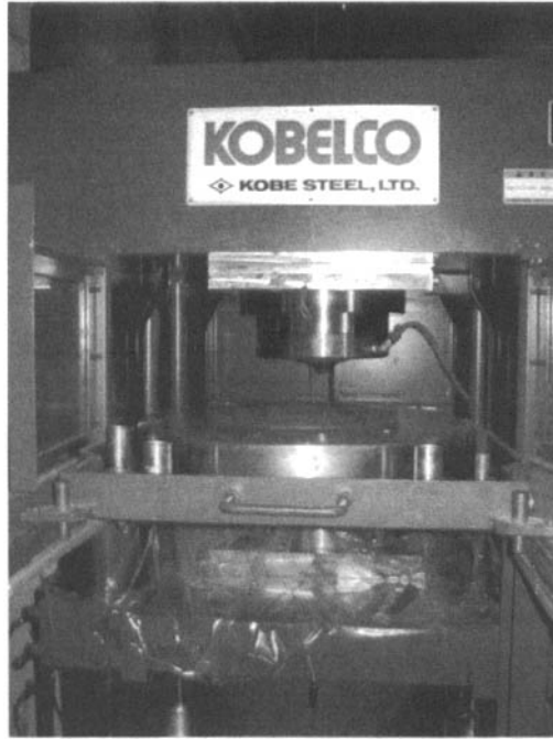
Figure 14.2 1500-ton belt-type high-pressure apparatus (National Institute of Advanced Industrial Science and Technology, Japan)
