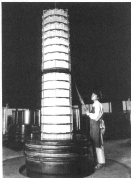
Figure 13.4 Growth of quartz crystals in the world's largest autoclave at Toyo Communications Ltd., Japan
