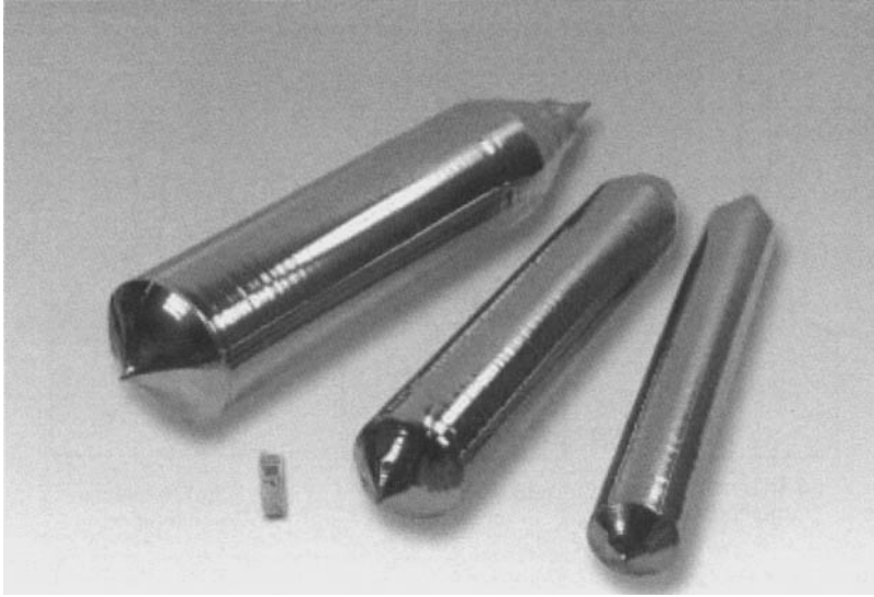
Figure 1.9 Dislocation-free silicon crystals grown recently (diameters of 150, 200 and 300 mm)
