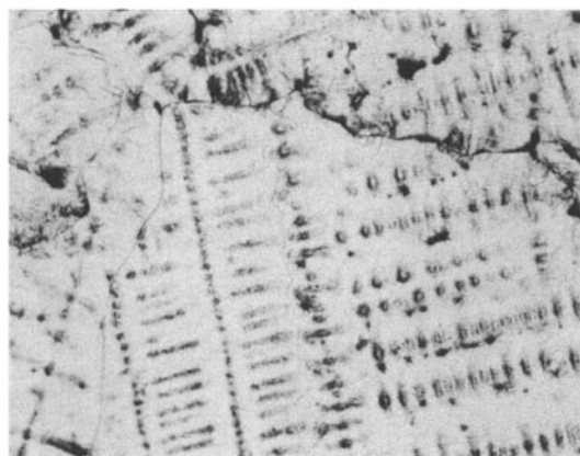
Figure 7.5 As-quenched microstructure showing dendrites and misfit dislocations (Reprinted from Tregilgas, Prog. Cryst. Growth Charac. 28 (1994) 57, copyright (1994) with permission from Elsevier Science)
