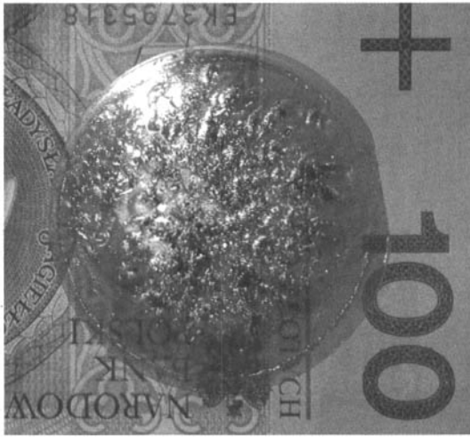
Figure 6.26 150- \mu m thick GaN grown on GaN/Al 2 O 3 substrate
