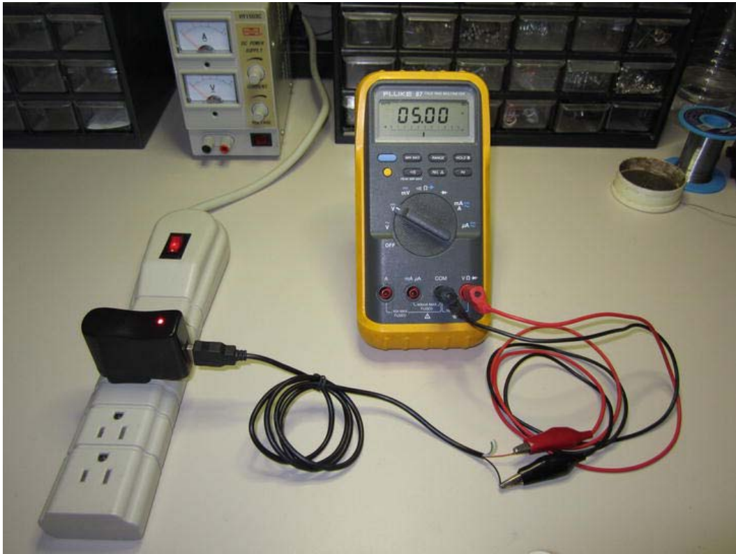
Figure A-7. Measure the voltage coming from the USB charger before connecting it to any of your circuits. This one reads 5V on the dot! This is a much safer method than trial by fire (i.e., plugging it into your circuit and looking for a fire).
