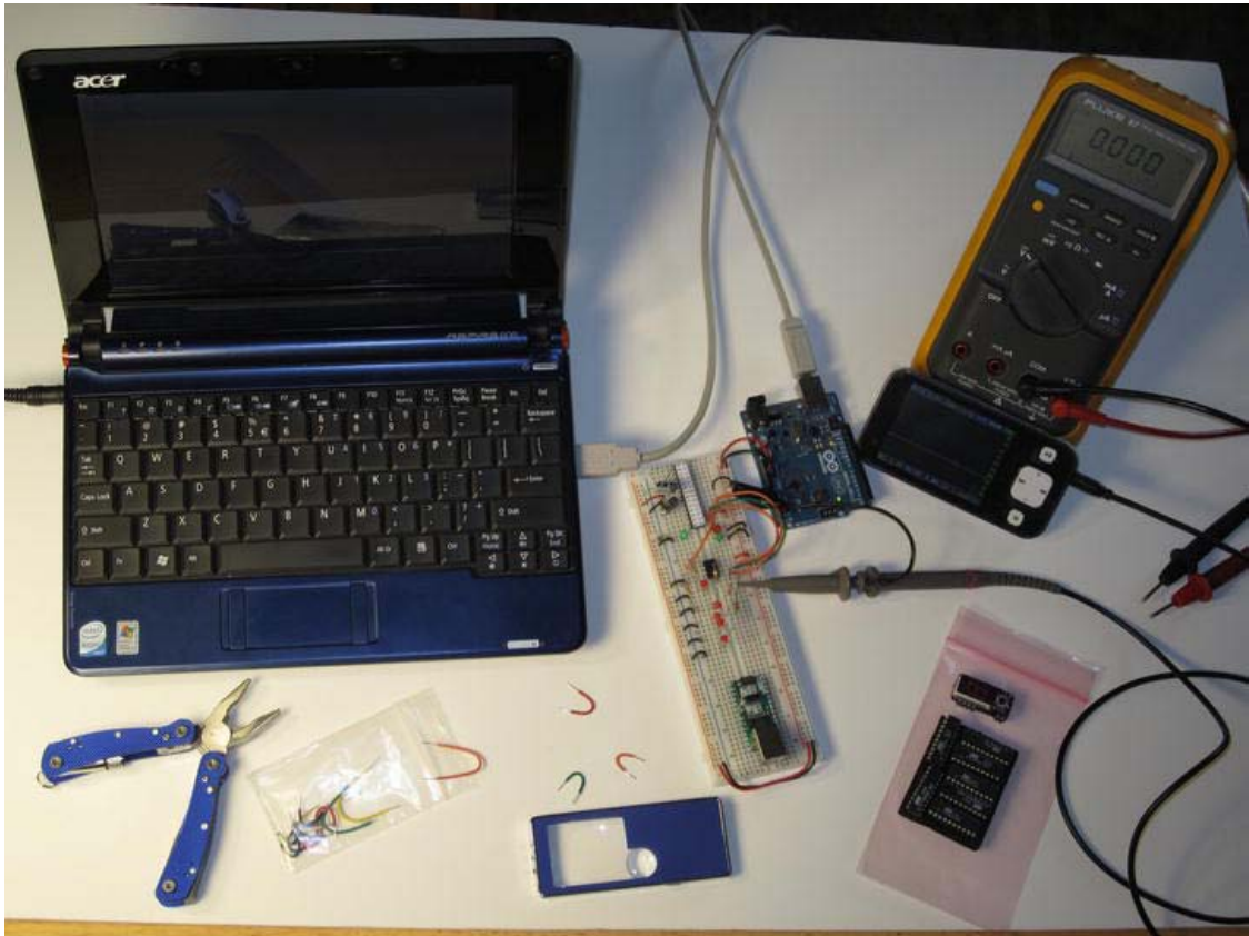
Figure 4-2. The compact executive lab is deployed on a desktop. You have access to lots of electronic building and debugging capabilities in a small area. Using a solderless breadboard helps reduce the number of fabrication tools that you need to carry with you on your adventures.
