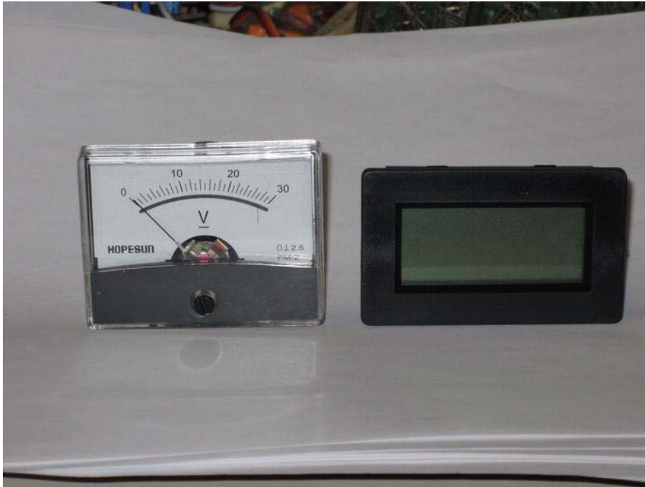
Figure 2-20. A panel-mount analog voltmeter (left) and a digital version (right)
