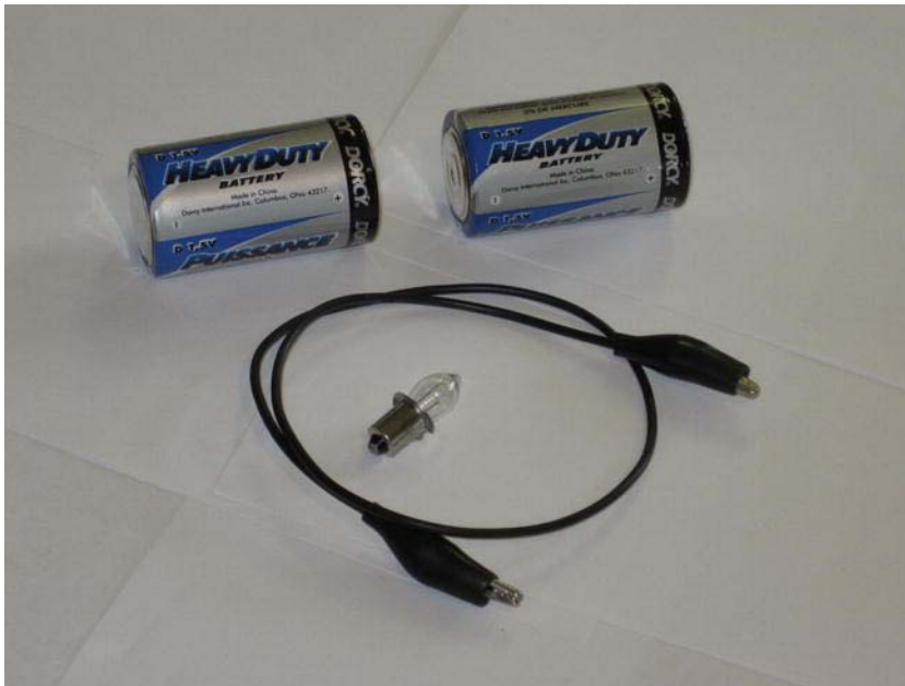
Figure 1-3. All the pieces you'll need to light up the bulb.
