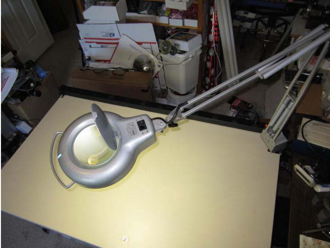
Figure 5-7. You will need some task lighting for your bench. This desk lamp also includes a handy magnifier for really close work.
