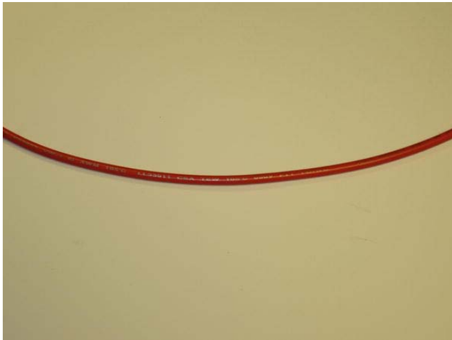
Figure 3-3. The wire's insulation only works up to a point. That point is usually printed on the insulation itself, but you may need to put on your good reading glasses to see it. This wire states, "LL33911 CSA TEW 105°C 600V FTT 14AWG," which translates to the manufacturer's part number, Canadian Standards Association certified thermoplastic equipment wire, maximum temperature of 105°C, 600V insulation dielectric strength, 14 gauge.
