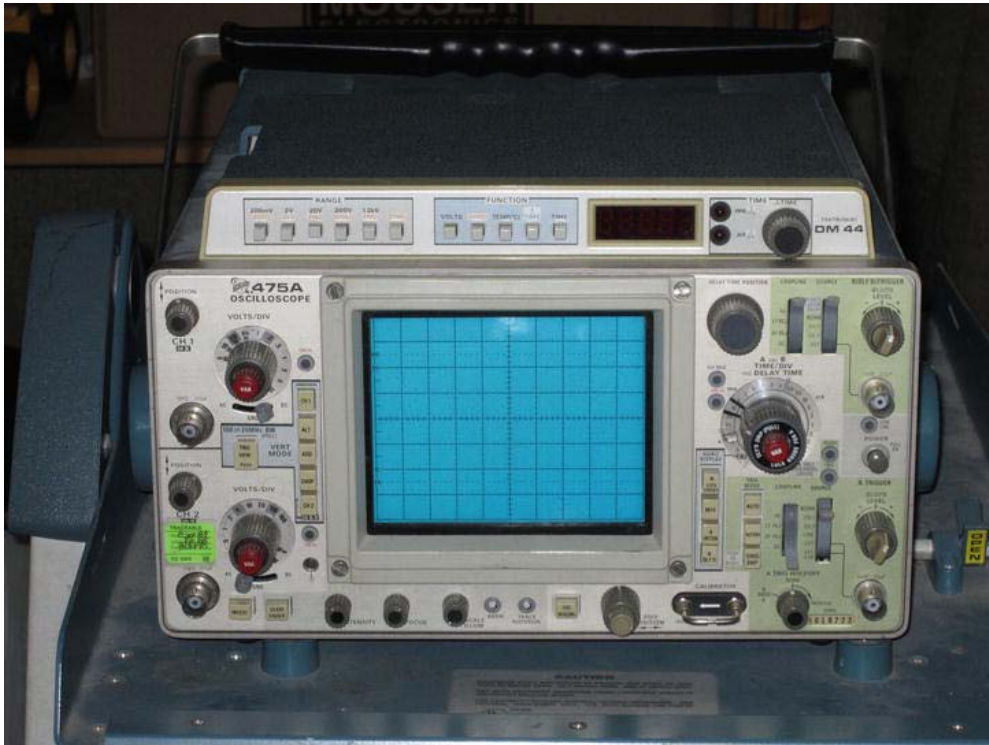
Figure 2-22. A Tektronix 475A oscilloscope. This piece of vintage test equipment is considered by some to be the best analog oscilloscope ever made. It also has a digital multimeter built in along the top edge.
