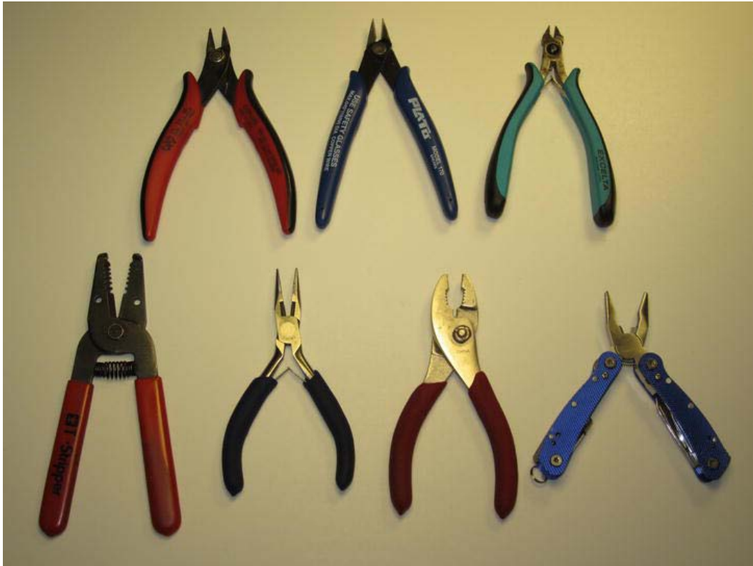
Figure 2-1. Commonly available wire-cutting tools. The top row shows three styles of diagonal cutters, which are the preferred tools for cutting small-gauge copper wire. The bottom row shows some tools that offer wire cutting as a secondary facility, and should only be used when proper wire cutters are not available.
