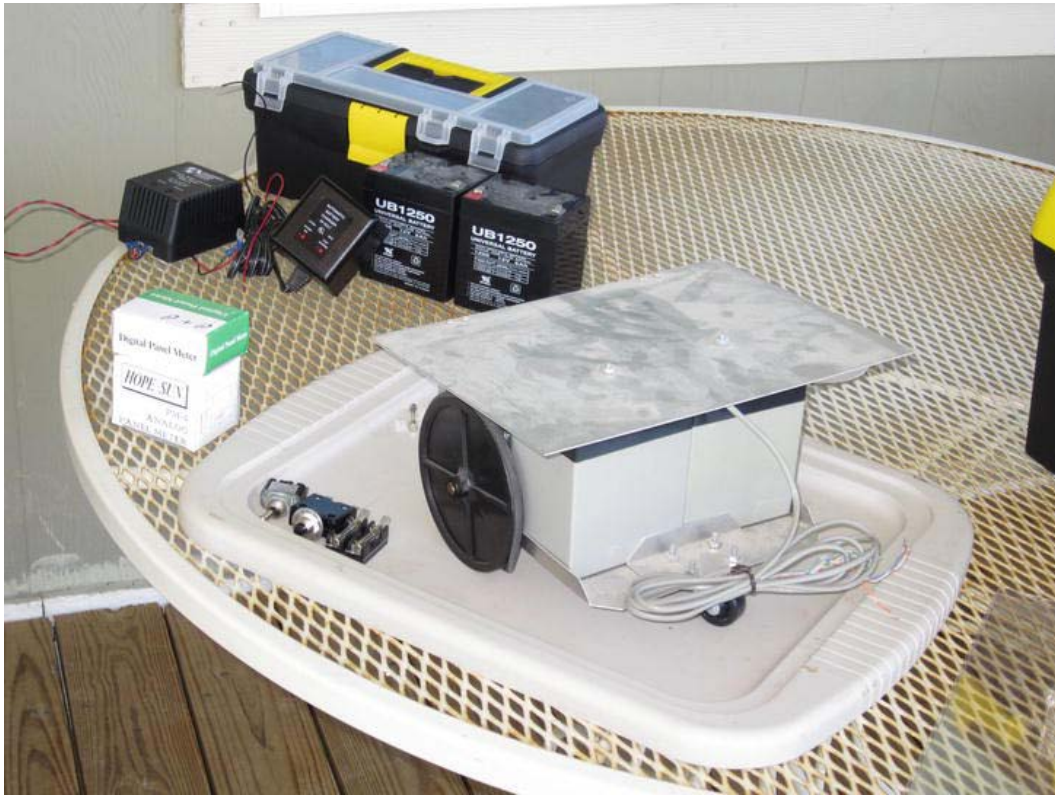
Figure 4-14. Kyle the Robot is a work-in-progress who requires a wide range of specialized tools and components. Some new components are being fitted, including dedicated battery voltmeters, fuses, a circuit breaker, and a master power switch. Once the sharp corners are filed off, Kyle will be able to roll around the house, looking for chores to do.
