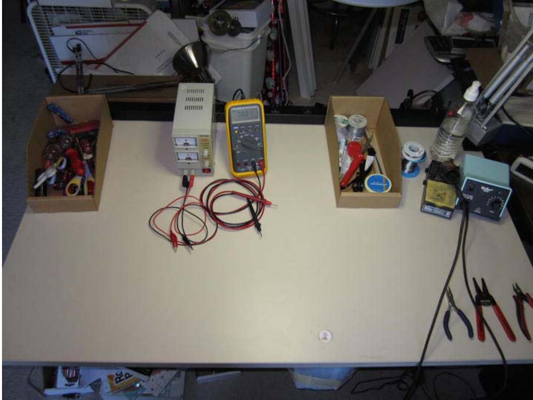
Figure 5-9. A clean bench with just enough tools to have some fun. Extra soldering supplies, including more kinds of solder, extra soldering iron tips, soldering flux, and an emergency backup soldering iron, sit in a box adjacent to the soldering station. Hand tools and basic test-and-measurement equipment complete the set of “most-useful tools.” There’s still room for a few more, when you need them.
