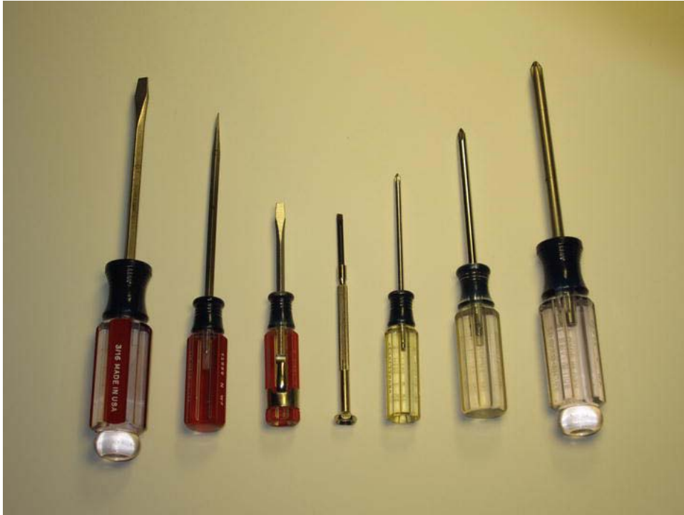
Figure 2-7. A variety of screwdrivers. The four on the left are standard, or straight-bladed, screwdrivers. The three on the right are Phillips-style screwdrivers. Other specialty bits are also available.
