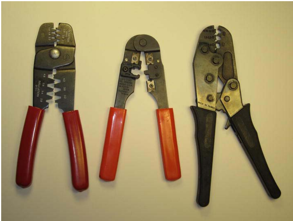
Figure 2-8. Some common crimping tools for affixing electrical connectors to wire
