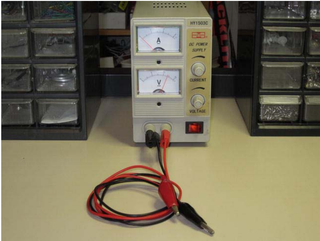
Figure A-1. A professional bench power supply. This device allows both the voltage and the maximum current to be adjusted. It provides two dedicated meters to show how much power is flowing: one for voltage and the other for current. It also provides a modular set of plugs (banana plugs) for easily connecting and disconnecting power leads.
