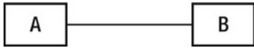
Figure 3-1. A very simple electrical schematic diagram, showing how to get from point A to point B with a single wire. Drawing wires in schematics is easy!
