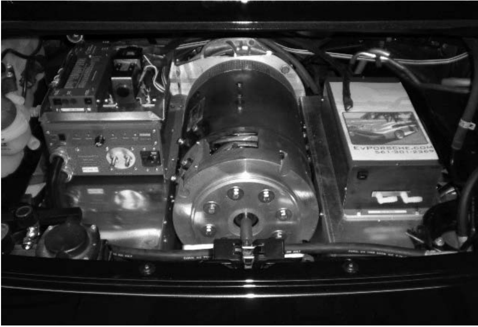
FIGURE 10-13 See how the motor is mounted into the compartment from Figure 10-9.
