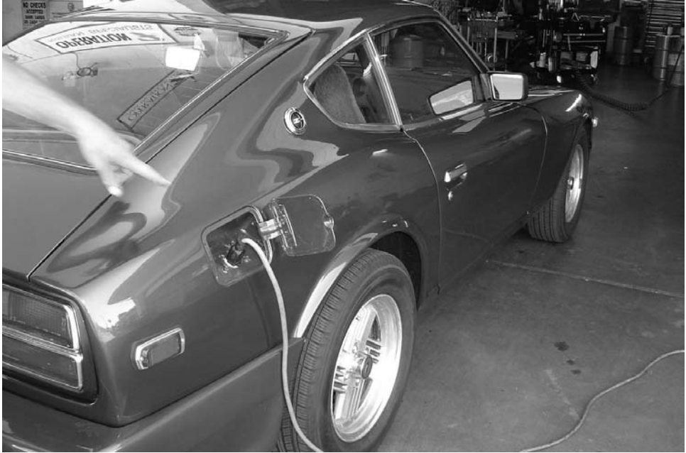
FIGURE 10-30 Operation Z charging connector and charging plug installed.
