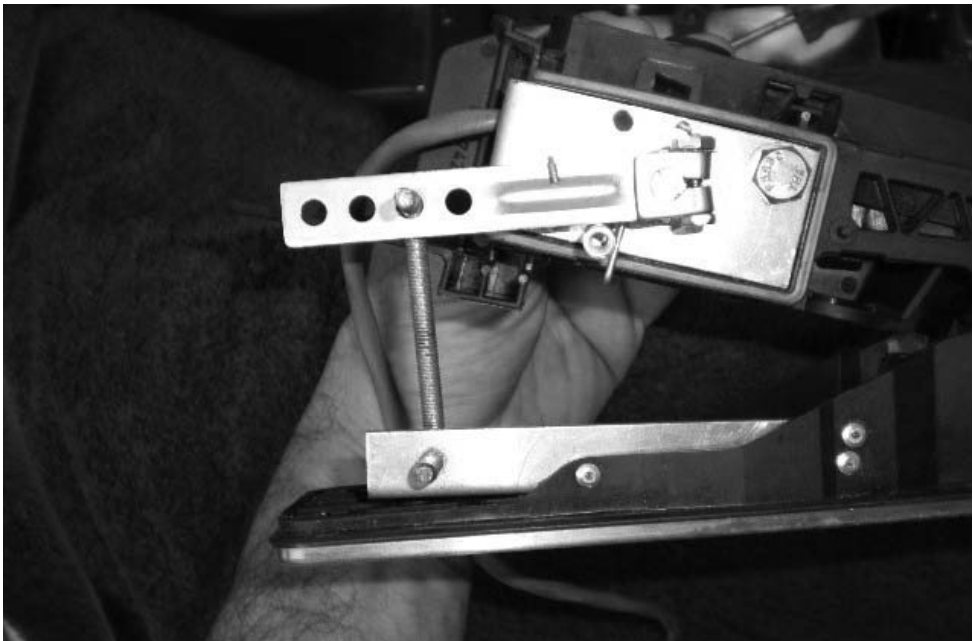
FIGURE 10-23 Electric Porsche throttle potentiometer (Courtesy of CoolGreenCars.net).
