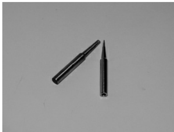
FIGURE 12.5 You'll want a flat-head tip (left) and a fine-point tip (right) for your soldering iron.
