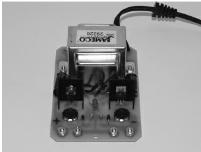
FIGURE 13.8 +DC and Ground on your power supply, along with the R4 adjust for DC output.
