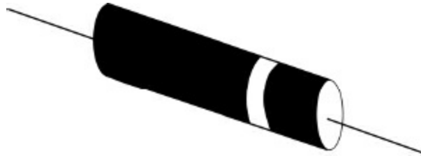
FIGURE 9.2 A silicon diode. The stripe indicates the location of the cathode within the glass tube.
