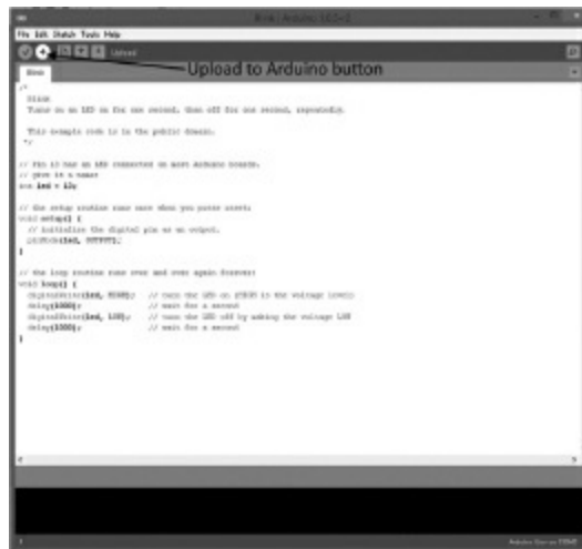
FIGURE 21A.5 Upload to Arduino using the indicated button.
