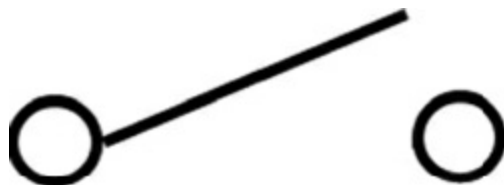
FIGURE 6.1 The symbol for an open switch in a circuit diagram.
