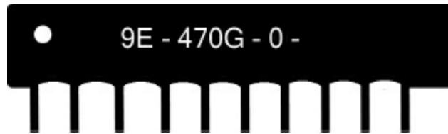
FIGURE 7.3 The SIL resistor pictured here has nine resistors, each delivering 47\Omega . The code reads 470, which equals 47 \times 10^0 , or 47.
