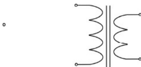
FIGURE 11.6 The symbol for a transformer in a circuit diagram.
