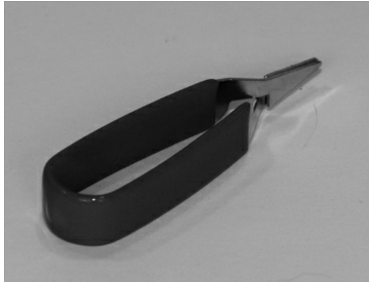
FIGURE 4.11 A heat sink with an insulated handle.
