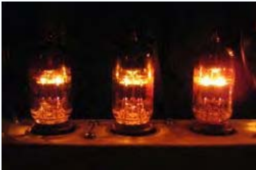
12AX7 tubes inside a modern guitar amplifier.
