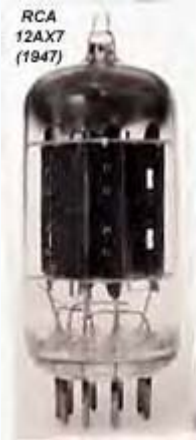
An RCA 12AX7 dual-triode tube (1947)
