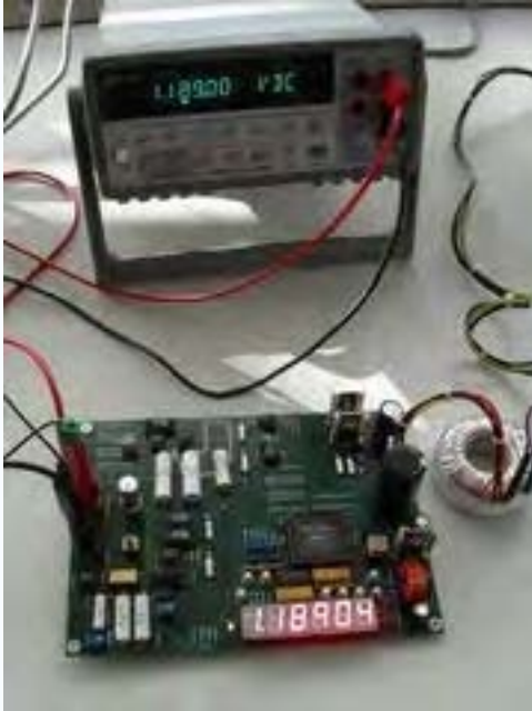
Commercial digital voltmeter checking a prototype
