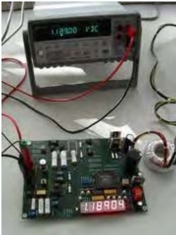
Commercial digital voltmeter checking a prototype
