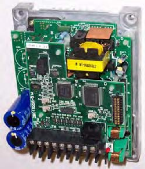
Hitachi J100 adjustable frequency drive chassis.
