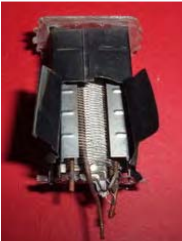
Inside of a vacuum tube with plate cut open.
