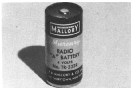
Fig. 6-10 A typical mercury battery. (Courtesy NRI Schools.)
