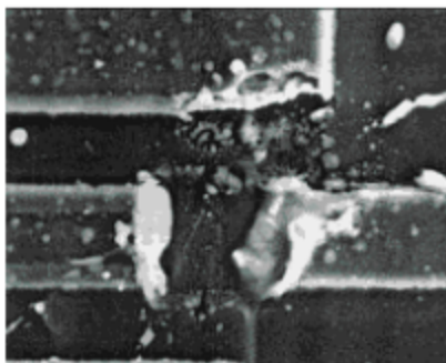
ESD CCA damage
