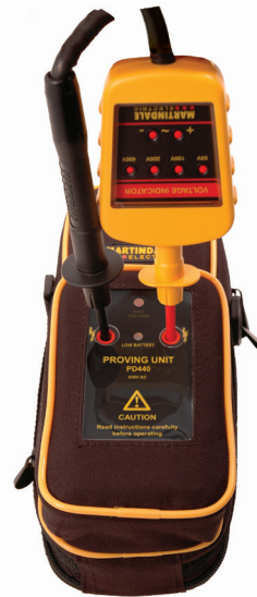
Figure 1.27 Voltage indicator being proved.
