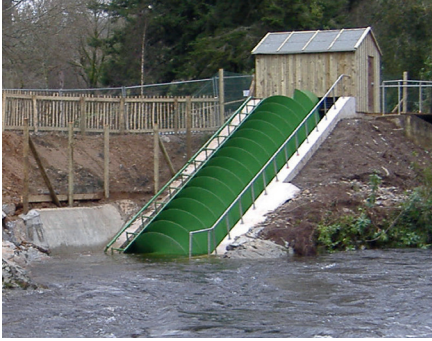
Figure 3.24 An example of an Archimedian Screw at the River Dart country park, Devon. Credit: WRE Limited.
