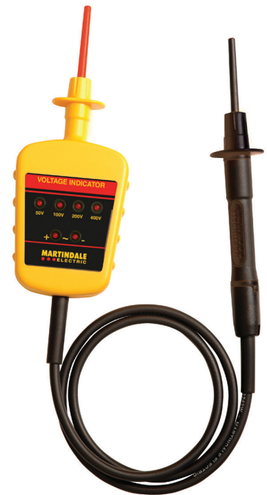
Figure 4.23 Typical voltage indicator.
