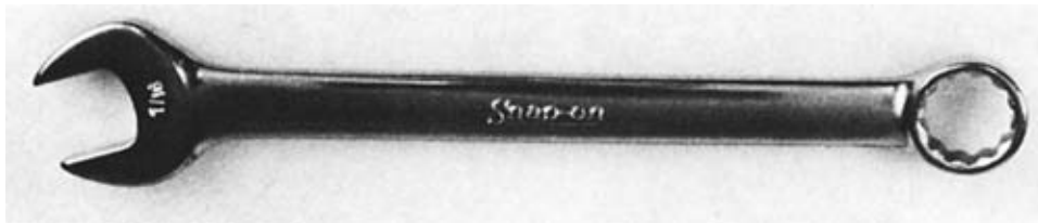
Figure 1-8. Combination wrench. The openings are the same size at both ends. Notice the angle of the open end to permit use in close spaces.
