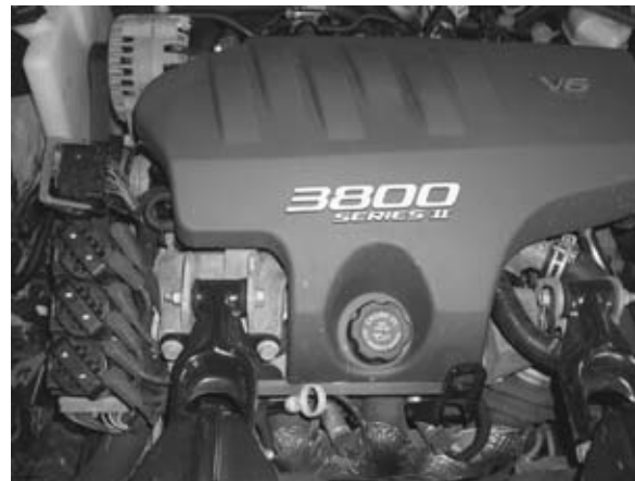
Figure 11-38. A typical distributorless ignition system coil pack may be mounted on the engine in a location that provides easy access.
