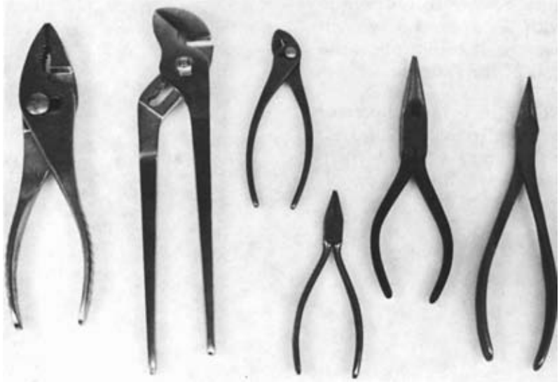
Figure 1-15. Assortment of pliers. Slip-joint pliers (far left) are often confused with water pump pliers (second from left).
