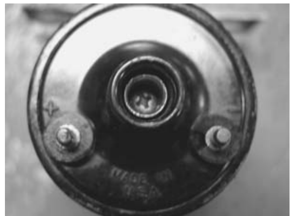
Figure 11-27. Many oil-filled coils are marked with the polarity of the primary leads.
