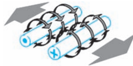
Figure 4-11. Conductors will move apart into weaker fields.
