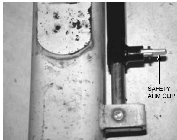
Figure 1-44. The safety arm clip should be engaged to prevent the possibility that the hoist support arms can move.
