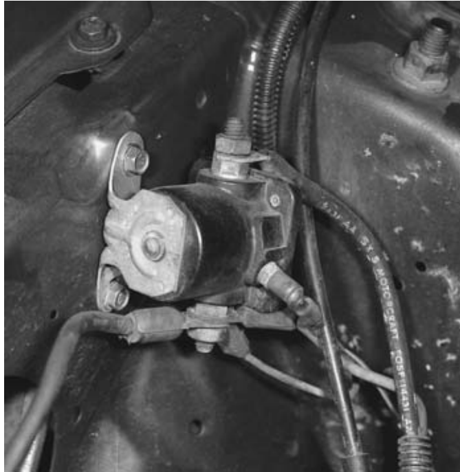
Figure 9-12. The Ford starter relay or magnetic switch.
