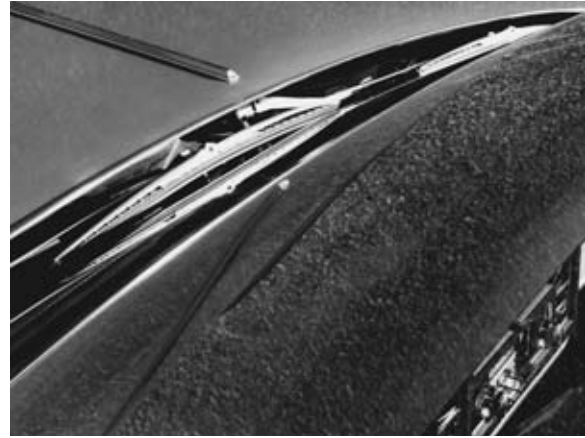
Figure 14-10. Many late-model cars have a depressed-park wiper position.
