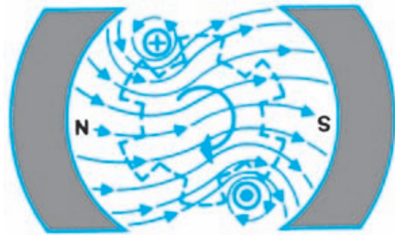
Figure 4-14. Electric motors use field interaction to produce mechanical energy and movement.
