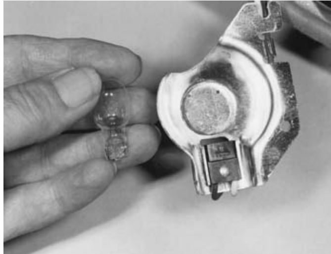
Figure 12-29. Wedge-base bulbs are increasingly used for interior lighting applications.
