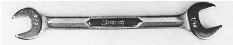
Figure 1-12. Open-end wrench. Each end has a different-sized opening and is recommended for general usage. Do not attempt to loosen or tighten bolts or nuts from or to full torque with an open-end wrench because it could round the flats of the fastener.
