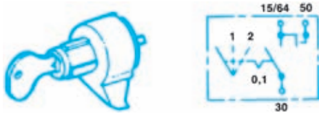
Figure 9-2. This ignition switch acts directly on the contact points. (Reprinted by permission of Robert Bosch GmbH)
