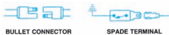
Figure 6-13. Male and female bullet connectors and spade terminals are common automotive connectors. (DaimlerChrysler Corporation)
