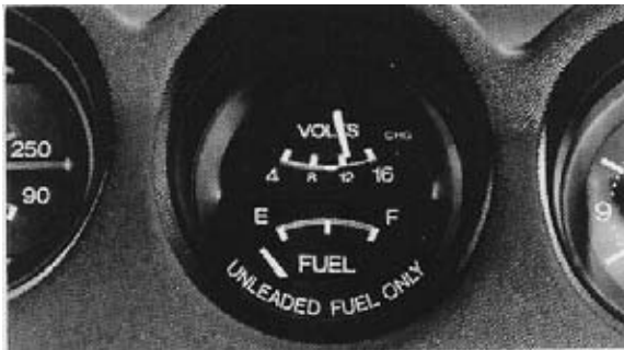
Figure 8-52. Automotive voltmeter in instrument panel.
