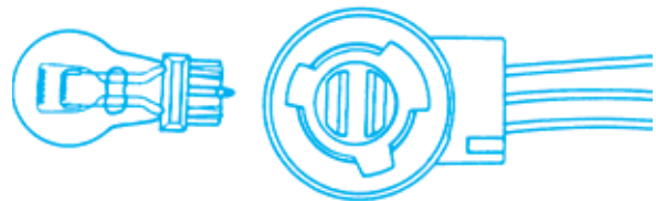
Figure 12-30. Wedge-base bulbs with plastic sockets are used for some external lighting applications. (DaimlerChrysler Corporation)
