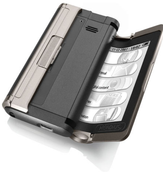
Fig. 1.2 Rollable electrophoretic display for e-readers and mobile phones. Source Polymer vision
