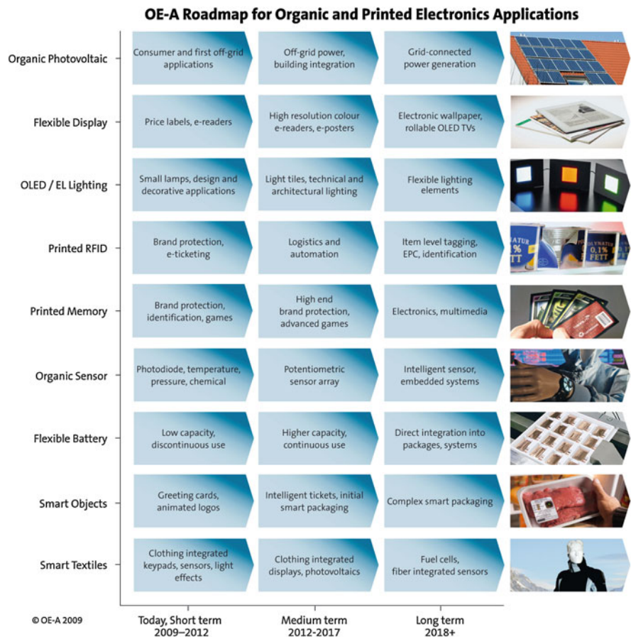
Fig. 1.10 OE-A Roadmap for organic electronics applications. Forecast for the market entry in large volumes (general availability) for the different applications. Source OE-A
