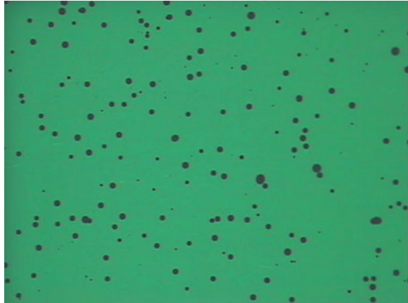
Fig. 4.11 Example of the formation of black spots in electroluminescence of an OLED as a result of storing the device at ambient conditions for a few days. The area of the picture is approximately 3 mm 2
