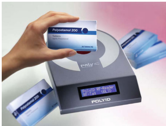
Fig. 6.10 Electronic brand protection with printed RFID in pharmaceutical applications (courtesy PolyIC)
