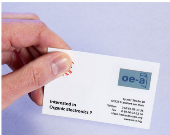
Fig. 1.8 Smart card with flexible battery and electrochromic display. Source OE-A
