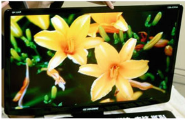
Fig. 3.6 31" AMOLED display made with micro-cavity technology
