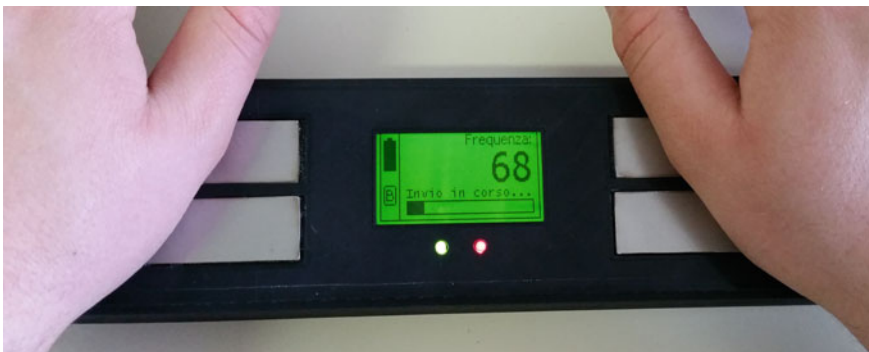
Fig. 4 User interface of the device while recording an ECG
