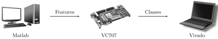
Fig. 6.16 Scheme of the neural network processing on the FPGA board. The board receives the features from a computer running Matlab, but the resulting plaque types (classes) are collected on a laptop through the Xilinx Vivado software
