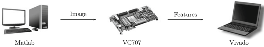
Fig. 6.7 Scheme of the feature extraction procedure on the FPGA board. The chip receives the image from a computer running Matlab, but the resulting features are collected on a laptop through the Xilinx Vivado software
