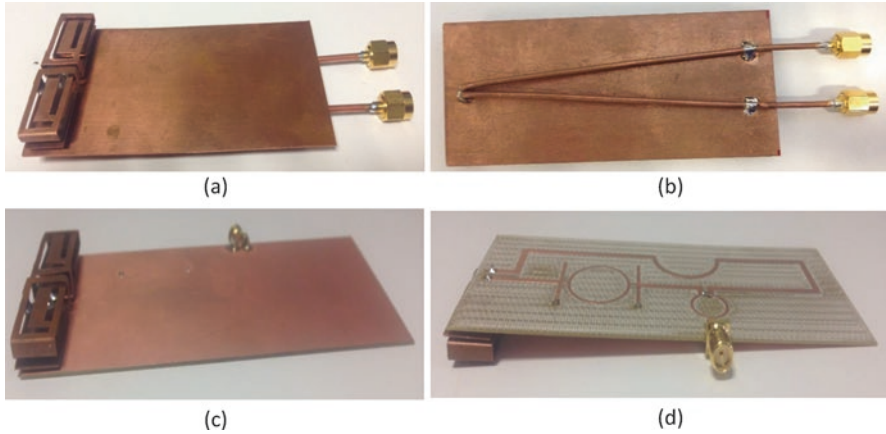
Fig. 13.9 The antenna prototypes, (a) top view antenna without balun, (b) bottom view antenna without balun, (c) top view antenna with balun, (d) bottom view antenna with balun
