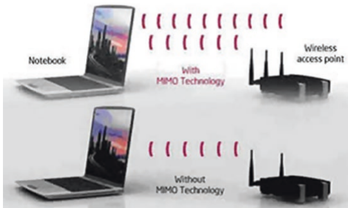
Fig. 1.4 MIMO technology uses multiple radios to transfer more data at the same time
