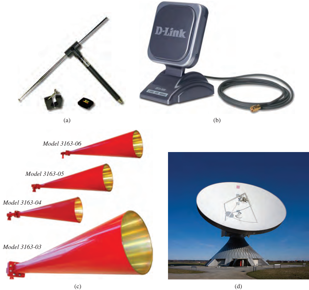
FIGURE 1-2 ■ (a) Dipole antenna [2]. (b) Patch antenna [3]. (c) Conical horn antennas [4]. (d) A high-gain parabolic antenna for satellite communication in Raisting, Germany [5].
