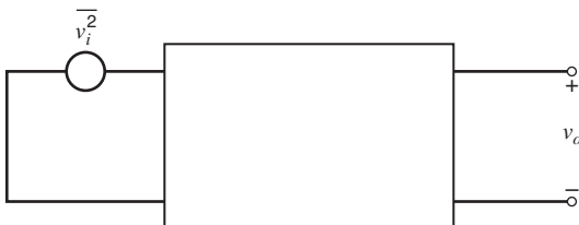
Figure 11.41 Circuit with equivalent input noise voltage generator.
