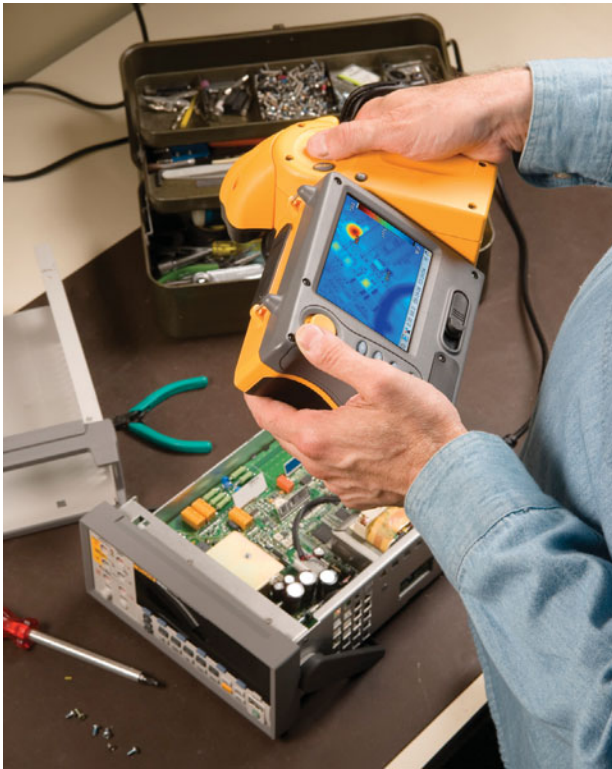
FIGURE SE1-4 Thermal imager showing the temperature profile of the target system (Photo provided courtesy of Fluke Corporation.)
