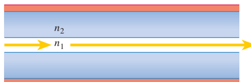
FIGURE 13–47 Single-mode step index fiber optic cable.
