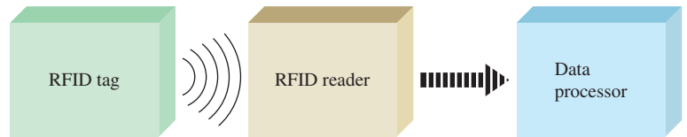
FIGURE SE9-1 Basic block diagram of an RFID system.
